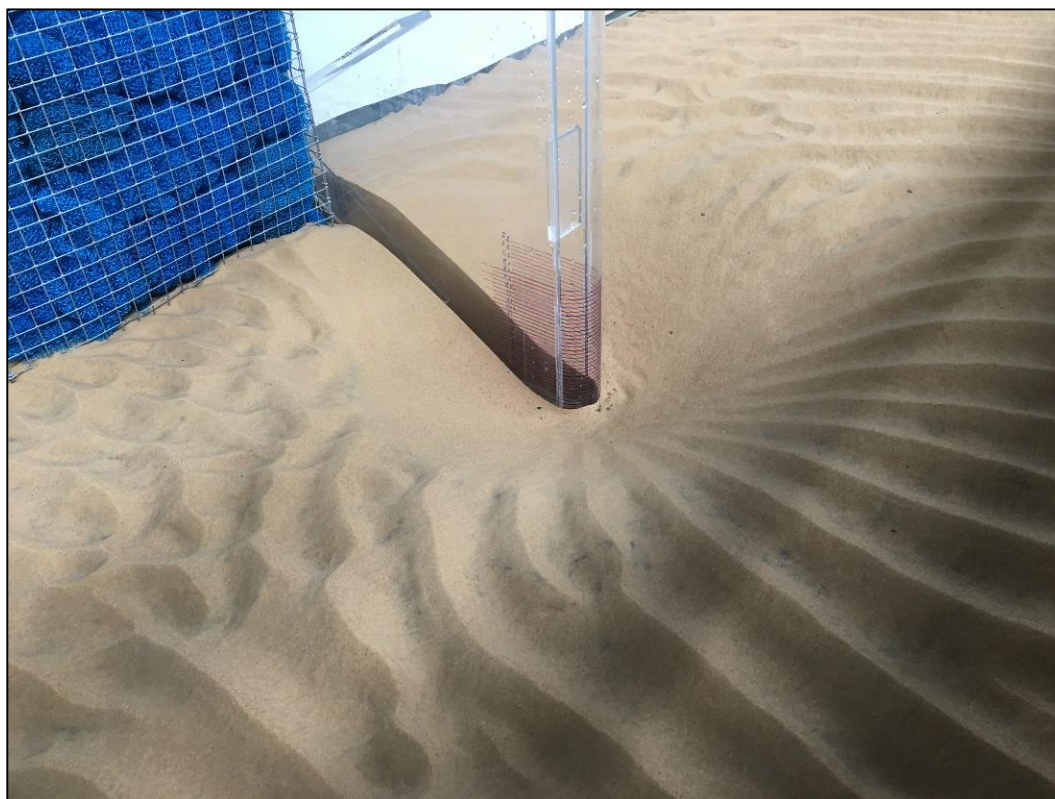
Figure 4.13. Round head structure model with scour hole (after KC=5.347 , ir-3)
