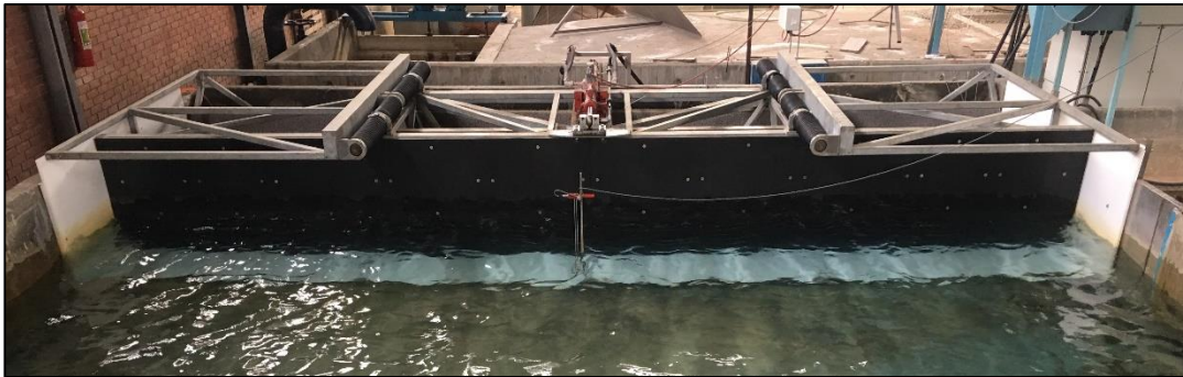
Figure 4.1. Piston-type wave generator
