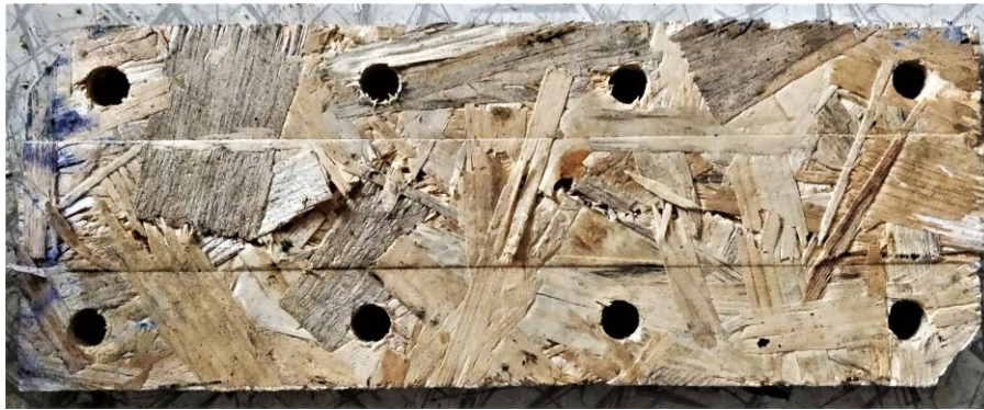
Figure 5.3 Deformed OSB panel specimen
