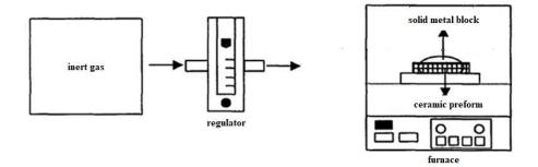
Figure 2.9. Illustration of the pressureless melt infiltration [29]
