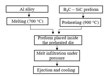
Figure 4.5. Pressure melt infiltration process
