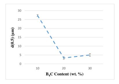
Figure 5.7. Variation of d(0.5) values with respect to  $B_4C$  content
