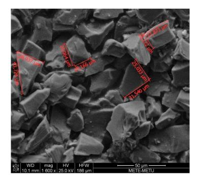
Figure 5.23. SEM analysis of SiC powder
