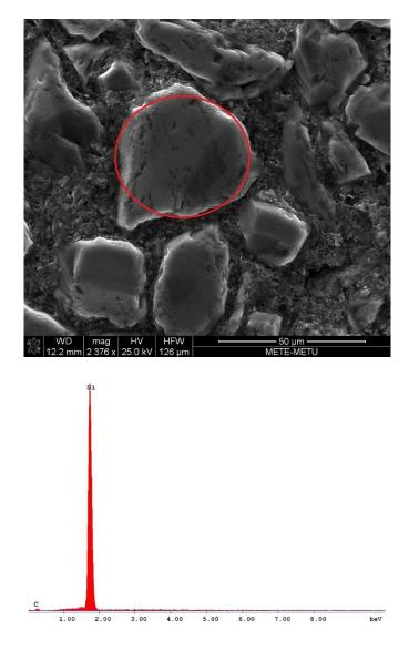
Figure 5.24. SEM-EDX analysis of SiC region of Al infiltrated 80S20B composite
