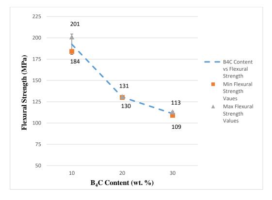
Figure 5.27. Flexural strength with respect to B<sub>4</sub>C content
