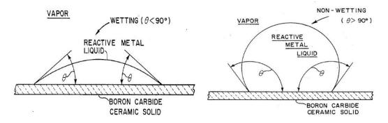
Figure 2.8. Illustration of the wetting and non-wetting conditions between solid ceramic and liquid metal [22]
