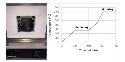
Figure 4.4. Furnace and temperature vs time graph of the sintering process
