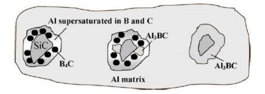
Figure 2.11. The infiltration mechanism of  $B_4C$  – SiC - Al composite [15]
