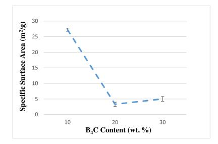
Figure 5.8. Variation of specific surface area values with respect to B<sub>4</sub>C content
