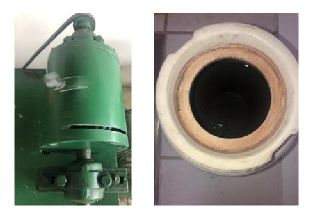
Figure 4.2. Ball milling machine and jar filled with ingredients
