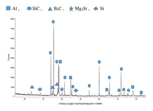
Figure 5.14. XRD analysis of Al alloy infiltrated 70S30B composite
