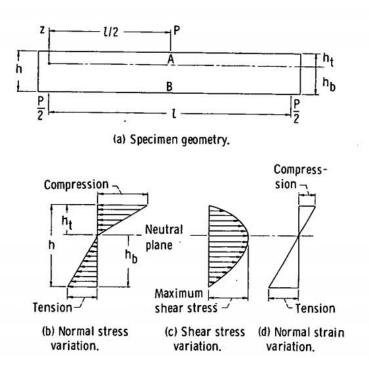
Figure 4.8. (a) Specimen geometry, (b) Normal stress variation, (c) Shear stress variation, (d) Normal strain variation [31]
