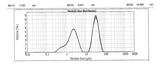
Figure 5.6. Particle size and distribution analysis of 70S30B
