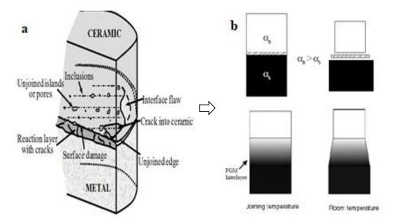
Figure 2.3. (a) Some problems due to joining of ceramic and metal, (b) The role of gradient for interlayer [2]
