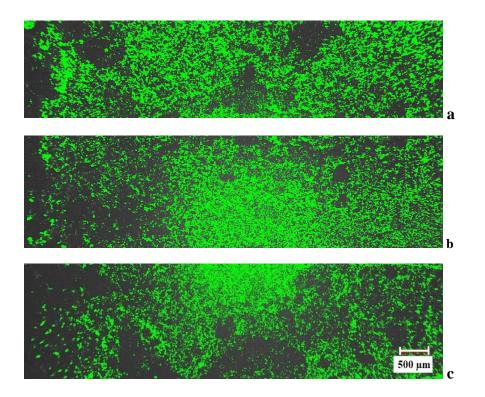
Figure 5.20. Phase analysis of FGM's layers which are (a) 90S10B, (b) 80S20B, (c) 70S30B
