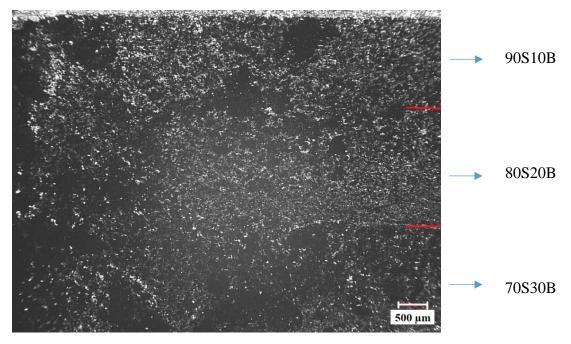
Figure 5.19. Microstructure of FGM
