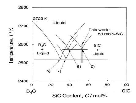
**Figure 2.7.** The phase diagram of the B<sub>4</sub>C – SiC system [17]
