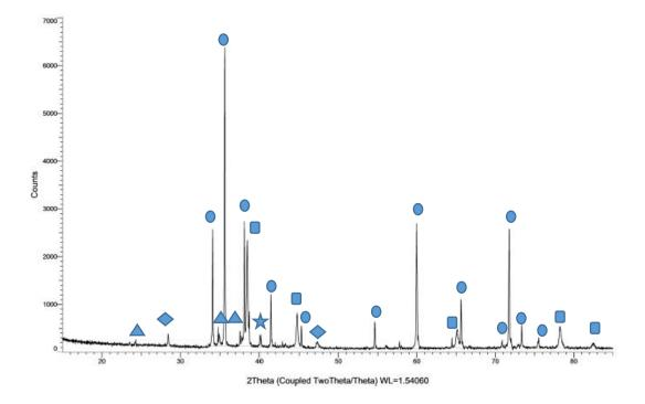
Figure 5.16. XRD analysis of Al alloy infiltrated 90S10B composite
