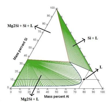
Figure 5.3. Ternary phase diagram of Al, Mg and Si elements at 700 °C
