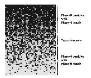
Figure 2.1. The schematic view of the FGM structure [5]
