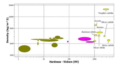
Figure 2.5. Image of CES Edupack program that shows density and hardness of ceramic materials
