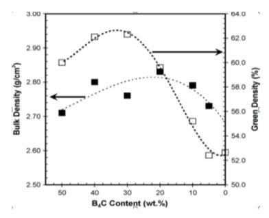
Figure 2.10. Green density vs B<sub>4</sub>C content [15]
