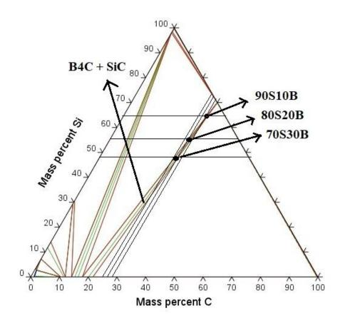
Figure 5.1. Ternary phase diagram of B, C and Si elements at 1400 °C
