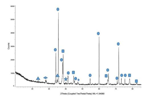
Figure 5.17. XRD analysis of Al alloy infiltrated FGM
