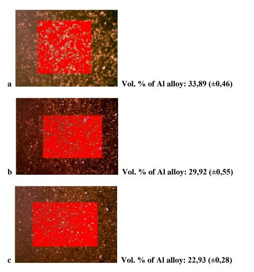
Figure 5.21. Phase analyses of Al alloy infiltrated (a) 90S10B, (b) 80S20B and (c)70S30B layers
