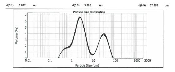
Figure 5.5. Particle size and distribution analysis of 80S20B
