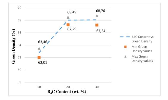
Figure 5.9. Green density variation with B<sub>4</sub>C content
