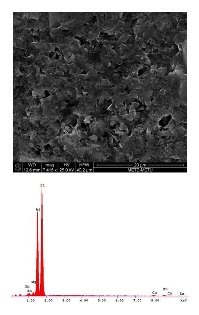
Figure 5.25. SEM-EDX analysis of Al alloy / B4C region of Al alloy infiltrated 80S20B composite
