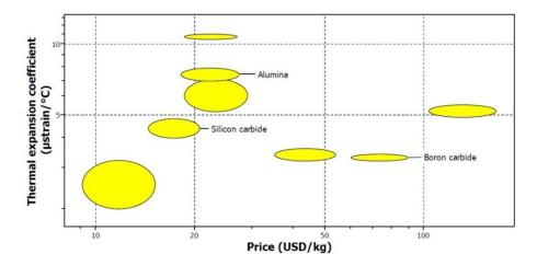
Figure 2.6. Image of CES Edupack program that shows price and thermal expansion coefficient of ceramic materials
