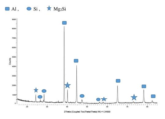
Figure 5.13. XRD analysis of Al alloy
