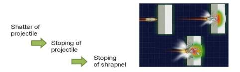
Figure 2.4. Projectile – Armor interaction in FGM [1]
