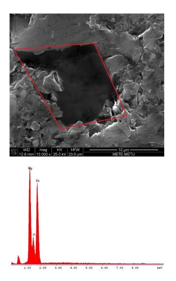
Figure 5.26. SEM-EDX analysis of Mg<sub>2</sub>Si region of Al alloy infiltrated 80S20B composite
