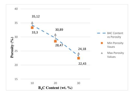
Figure 5.10. Porosity % variation with B<sub>4</sub>C content
