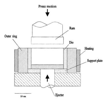
Figure 2.12. Illustration of the pressure melt infiltration [26]
