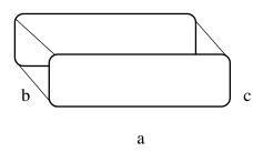
$V_{obtained} = a \cdot b \cdot c$   $V_{theoretical} = (m_{B4C} / d_{B4C}) + (m_{SiC} / d_{SiC})$ % dgreen = (V\_{theoretical} / V\_{obtained}) .100
