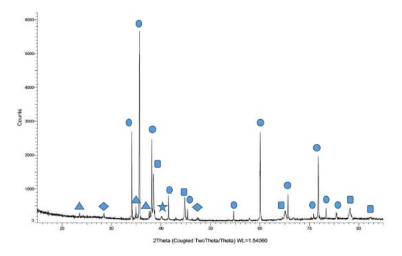
Figure 5.15. XRD analysis of Al alloy infiltrated 80S20B composite
