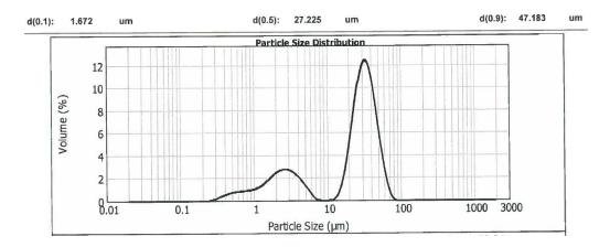
Figure 5.4. Particle size and distribution analysis of 90S10B
