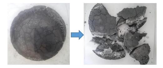
Figure 5.12. 80S10B10A sample was put into water and crashed
