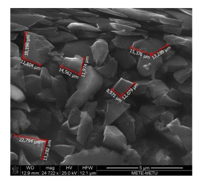
Figure 5.22. SEM analysis of B<sub>4</sub>C powder
