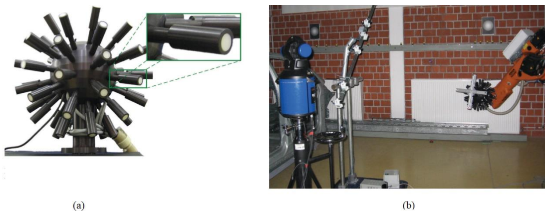
Figure 2.21. An innovative LEDs target for the TCP pose estimation purposes [66]
