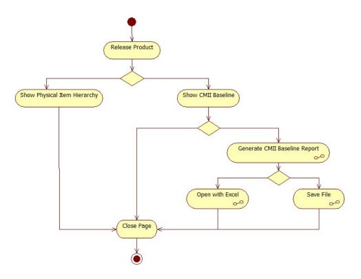
Figure 4.8: Activity diagram of customization functions
