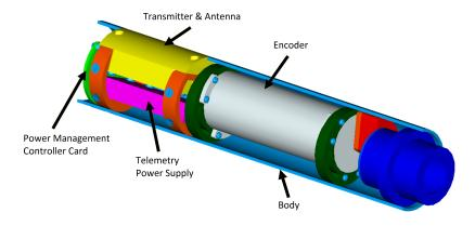
Figure 5.2: Missile telemetry system
