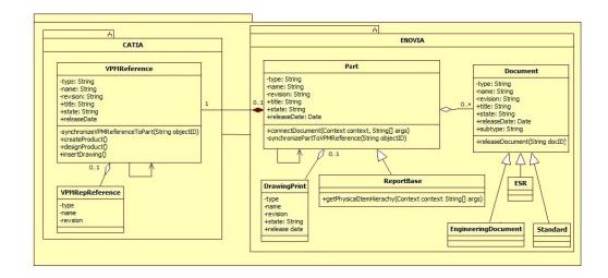
Figure 4.7: Class diagram
