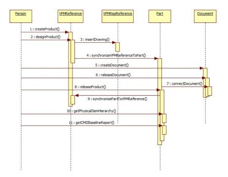
Figure 4.14: Sequence diagram for tool extension functions
