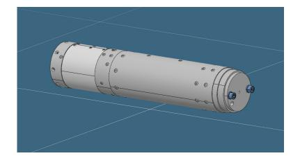
Figure 5.3: CAD model of the telemetry system
