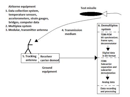
Figure 5.1: Missile test example of telemetry system overview [14]
