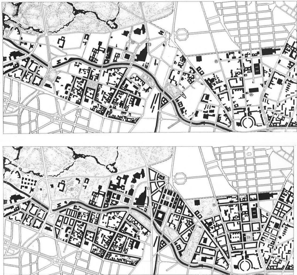
Figure 3.6. Kleihues' master plan - above the current state, below the proposed design. Through block-edge development, the IBA rehabilitated historical roads and invented some new in the vicinity of the wall.
