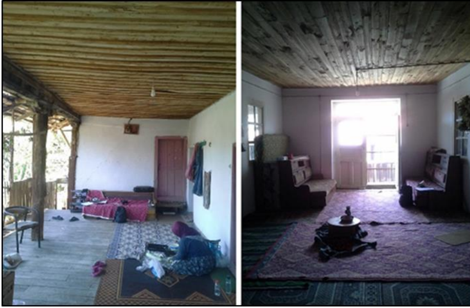
Figure 38: The first photo, taken from the H16, shows the open ‘sofa’ with rooms located on one side of it; the second photo, taken from the H8, shows the closed ‘sofa’ located in between the rooms.
