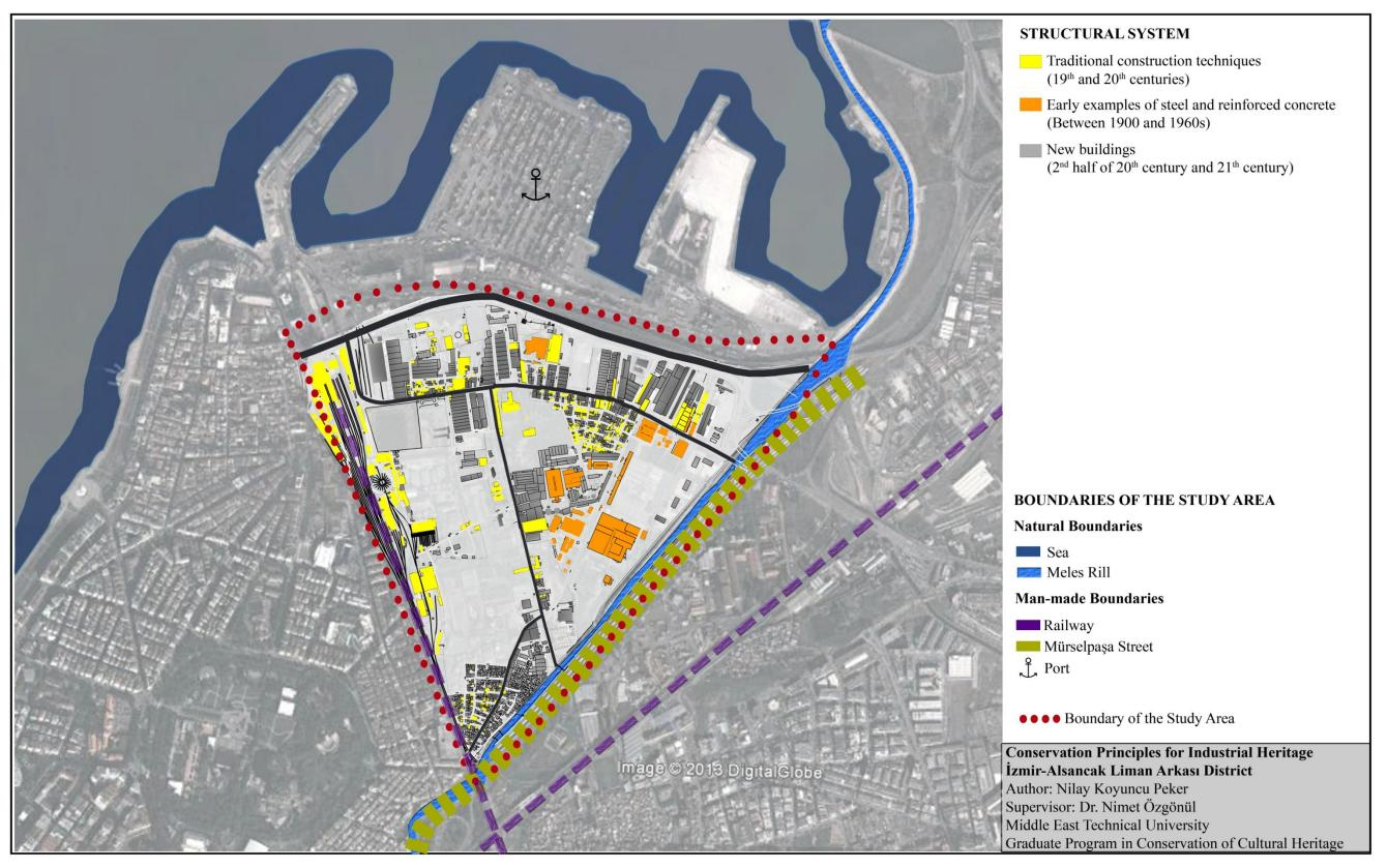
Figure 3-9: Structural System in the Study Area.
