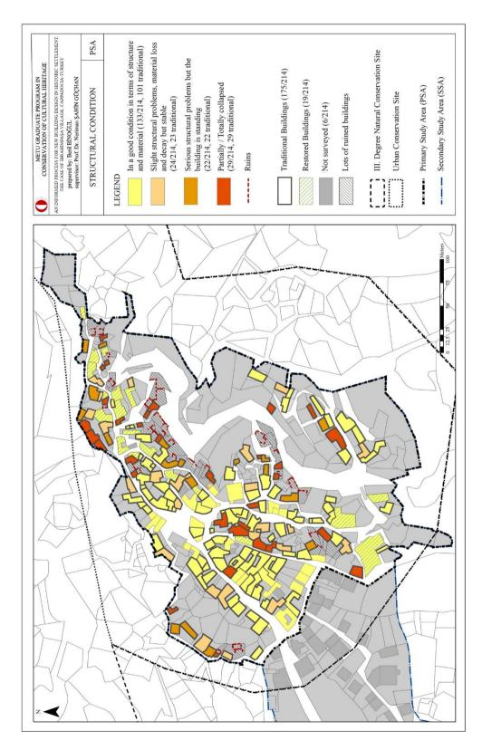
Figure 4.49. Structural condition
