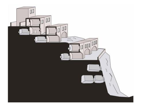
Figure 4.28. Schematic section of the village showing the placement of the buildings on the slopes
