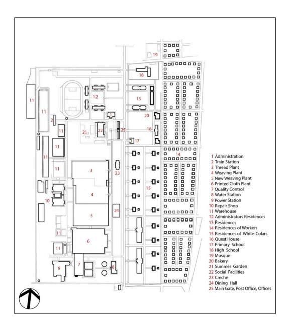
Figure 3.12. Site Plan of Sümerbank Nazilli Textile Factory (Adapted from Uzunoğlu, 2008, 95)
