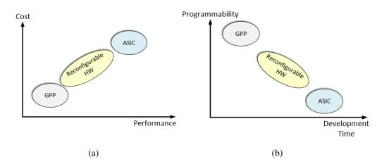
Figure 1.1: GPP, ASIC and Reconfigurable Hardware Comparison in terms of Performance, Cost, Development Time and Programmability [1, 2].
