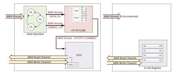
Figure 4.6: Reconfigurable Module Connections
