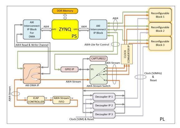
Figure 4.3: Complete Architecture for Context-Switchable PR System on Zynq SoC
