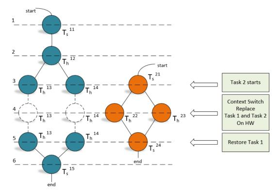
Figure 3.3: Task Model for Context Switching
