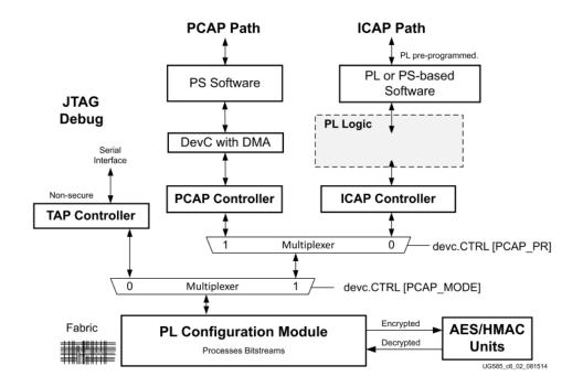
Figure 3.10: PCAP and ICAP Configuration Paths
