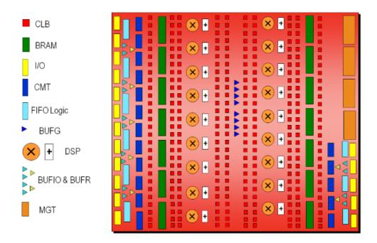
Figure 2.4: A Small Representation of Xilinx 7-Series Architecture
