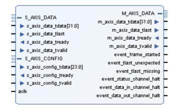
Figure 4.5: FFT IP Core I/O Structure
