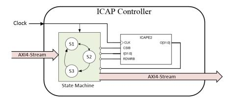
Figure 3.9: ICAP Controller and ICAPE2 Primitive
