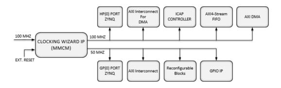
Figure 4.4: Clock Distribution for Overall Design
