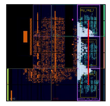
Figure 4.10: Floorplanning For The Example Application
