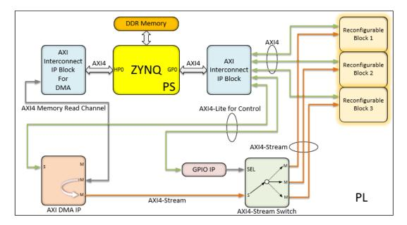
Figure 4.2: Base System for HW Tasks Without ICAP Controller
