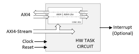
Figure 3.5: AXI4-based Reconfigurable Block Model
