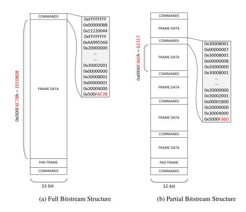
Figure 2.10: A Full and Partial Bitstream Structure of Xilinx 7-Series FPGAs [24]
