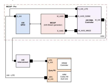
Figure 2.13: MiCAP-Pro Readback and Reconfiguration Model [32]
