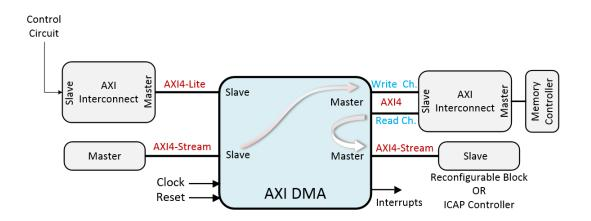
Figure 3.8: AXI DMA I/O structure
