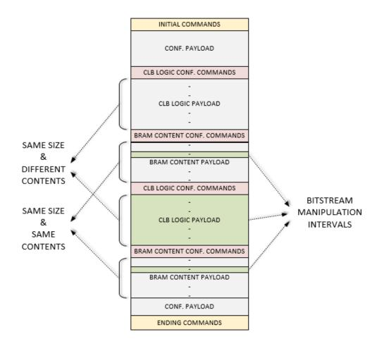
Figure 3.12: A general partial bitstream structure and manipulation intervals
