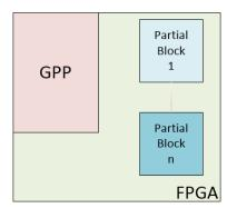
Figure 1.2: General Partially Reconfigurable SoC Hardware Architecture
