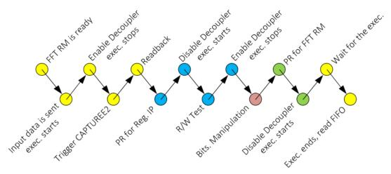
Figure 4.7: Example Application Context Switching Flow
