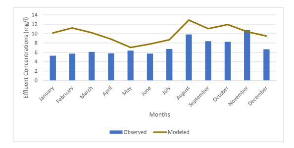
Figure 5-11 Effluent TSS concentrations for 2017 Validation
