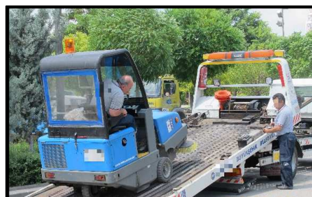
Figure 4.27. Loading of Sweeping Machine
