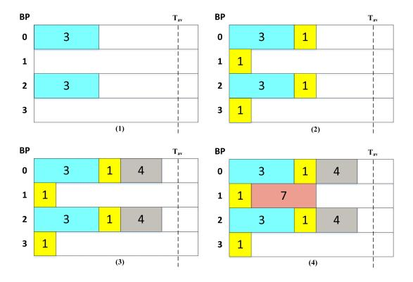
Figure 3.10: Placement of the First Three Telegrams in SAB
