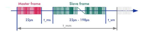
Figure 2.3: Telegram Structure and Timing
