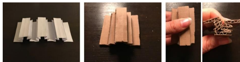
Figure 3.5. Left: Origami Model; Right: Top View and Cross Section of Rigid Folding
