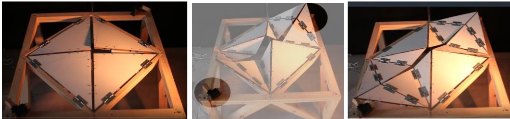
Figure 3.18. Prototyping with Arduino and Servo Motor (developed by the author)
