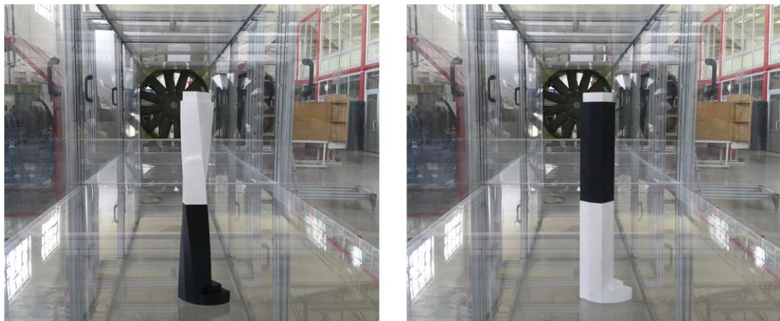
Figure 3.10. Twisting (left panel) and prismatic (right panel) models of HFBB tests
