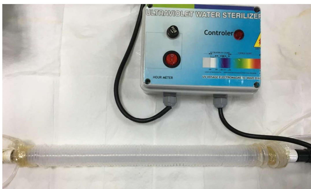
Figure 2.3. Photograph of UV lamp-Photochemical Reactor used in the study
