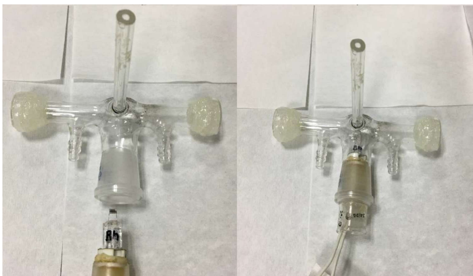
Figure 2.5. A laboratory made tungsten-coil atomizer used in this thesis study
