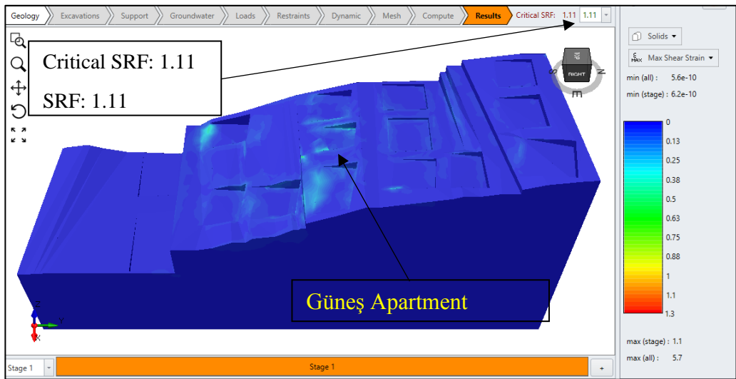
Figure 5.25. Strain accumulation zones at the critical SRF.
