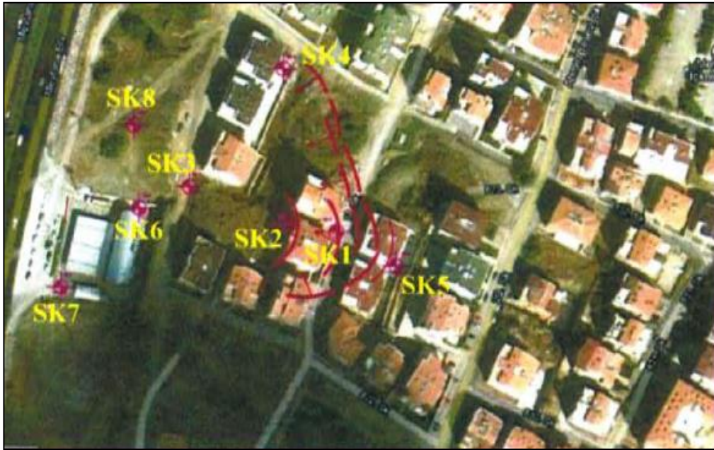
Figure 4.6. Locations of the boreholes installed by Kiper Co. (Çokça et al., 2011).
