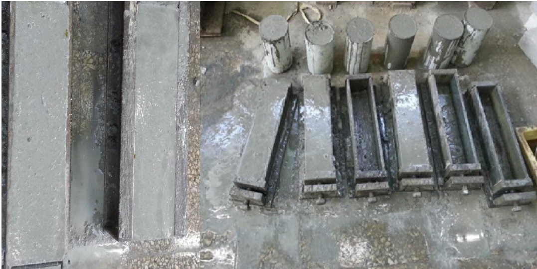
Figure 3.3 Placing of Concrete into Big Beams and Small Beams
