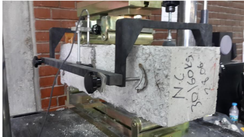
Figure 3.5 Testing of Big Beams
