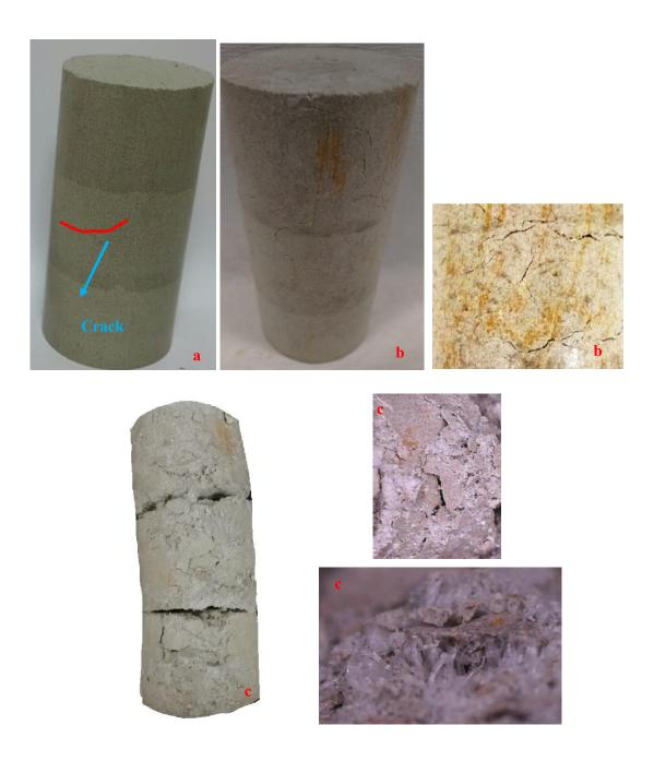
*Figure 6.11.* 40000ppm NS added 10% KFA treated specimen cured at 10°C for a- 28 days, b- 3 months, c- 9 months
