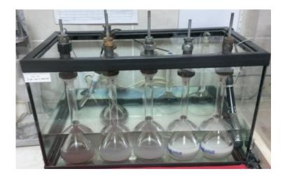
Figure 4.34. G<sub>s</sub> samples in water tank
