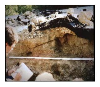
*Figure 3.2.* Evidence of accumulation of considerable lateral strain resulting in shear failure in lime-treated high sulfate soil layer (Little and Nair, 2009)
