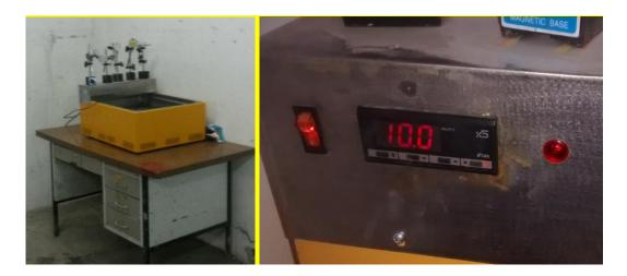
Figure 4.17. Water bath for 10°C tests
