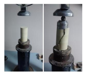
Figure 4.22. Views from UCS tests (Specimen A)
