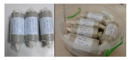
Figure 4.23. Curing for UCS test
