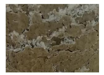
*Figure 5.56.* Crystal formed within the 40000ppm NS added 15% SFA treated sample cured for 6 months at 10°C
