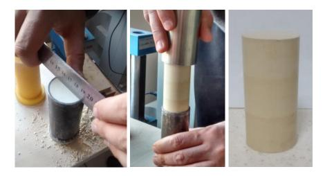
Figure 4.20. View from specimen compaction
