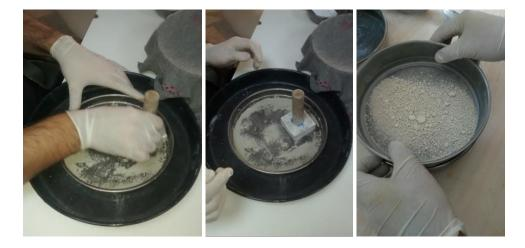
Figure 4.8. Crushing particles that sticked to each other with wooden blocks and sieving
