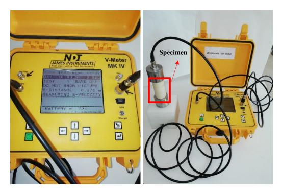
Figure 4.24. Measurement of Vs with V-meter Mark IV
