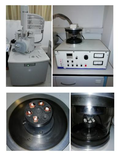
Figure 4.27. Scanning electron microscope and vacuum device
