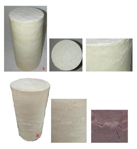
Figure 6.12. 40000ppm NS added 4% L treated specimen cured at 10°C for a- 4 months, b- 9 months
