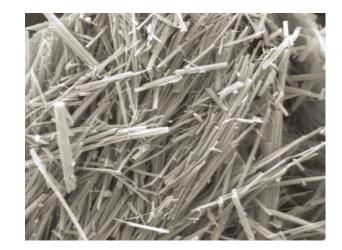
Figure 4.26. SEM view of purified thaumasite (Mittermayr et al., 2012)
