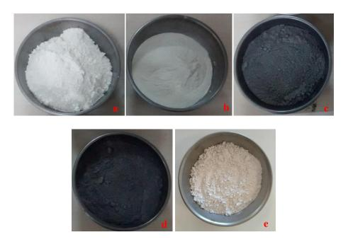
Figure 4.1. Materials (a-kaolinite, b-bentonite, c-soma fly ash, d-sivas-kangal fly ash, e-lime)
