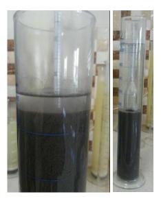
Figure 5.25. Hydrometer test for KFA
