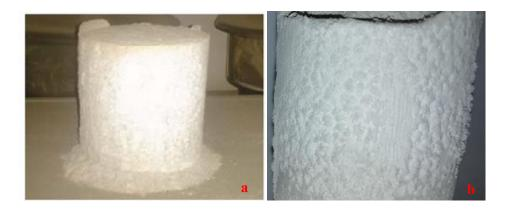
*Figure 6.15.* Views form powdered of NS, a- study of Xusheng et al., 2017, b- this study (dry form of 40000ppm NS Added 10% KFA treated specimen cured at 40°C for 28 days.)
