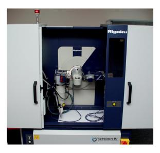
Figure 4.29. Rigaku Ultimate-IV brand X-ray diffractometer
