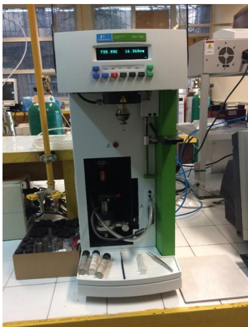
Figure 3.3. PerkinElmer Pyris-1 TGA apparatus
