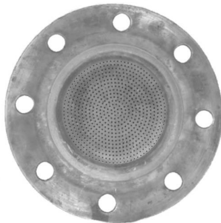
Figure 3.10. Distributor plate used in the combustor.
