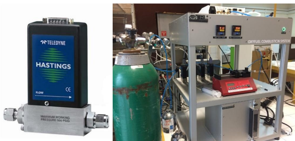
Figure 3.4. Teledyne HFC 202 mass flow controller ( left ) and the gas mixing unit ( right )
