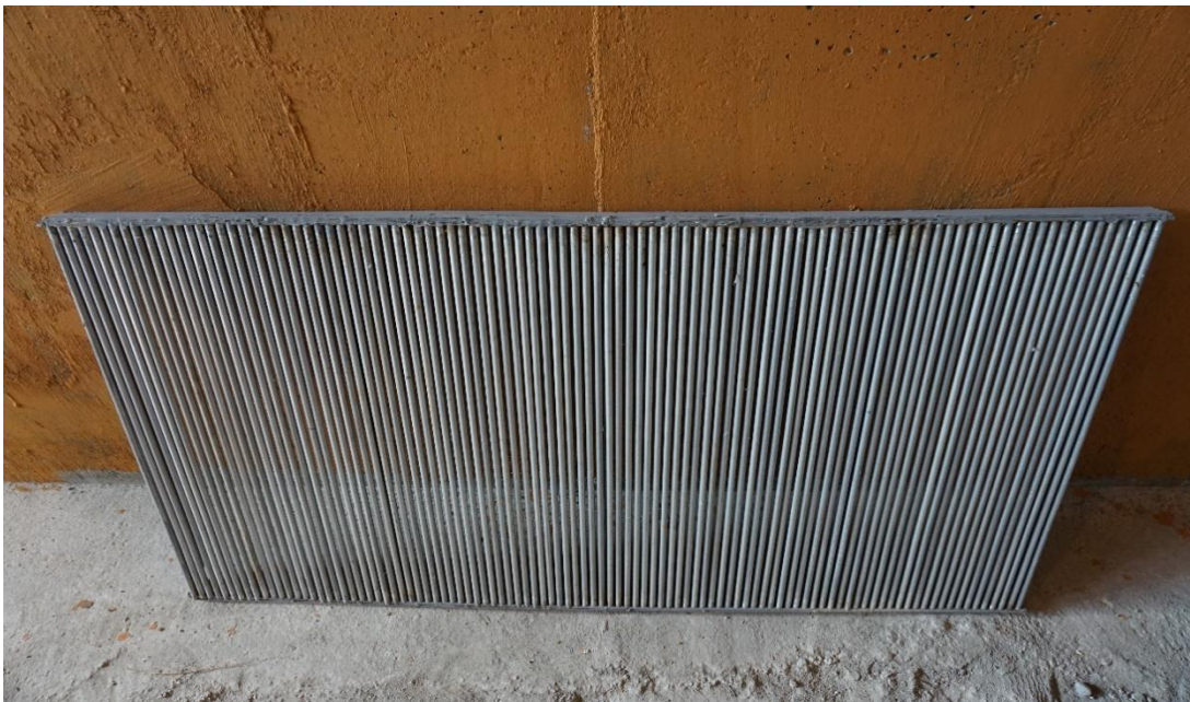
Figure 3.8. View of the rack with clear bar spacing of e_1=3 mm
