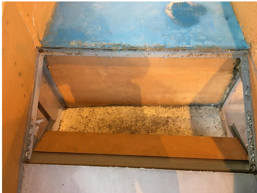
Figure 3.18. Accumulation of sediment (A-2 Group Experiments) within the “Collection Channel-1” ( e_1=3 mm, Z_1= 10 cm, Z_2= 25 cm, \alpha=20^\circ )
