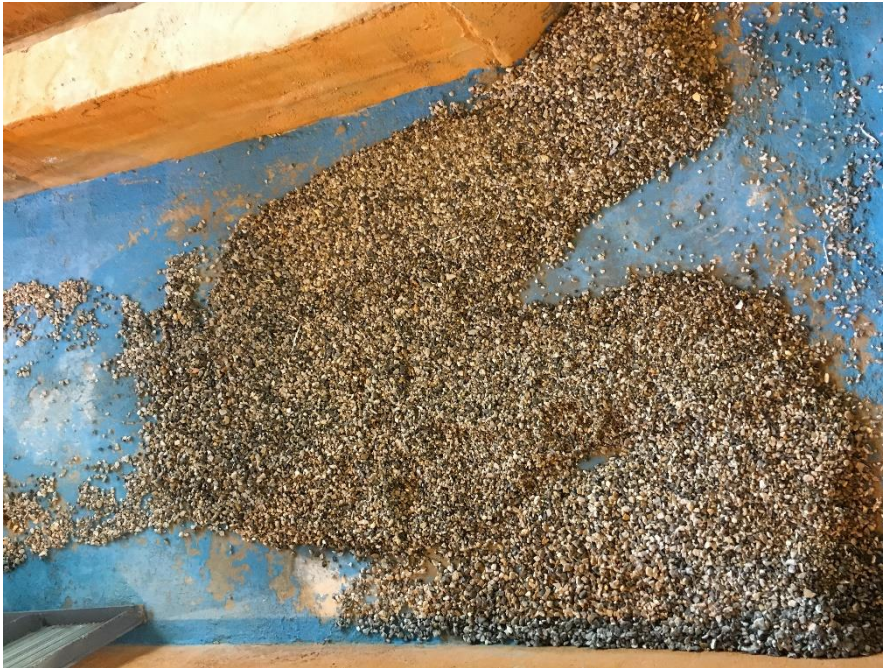
Figure 3.19. Accumulation of sediment (A-2 Group Experiments) at the downstream of the main channel ( e_1=3 mm, Z_1= 10 cm, Z_2= 25 cm, \alpha=20^\circ )
