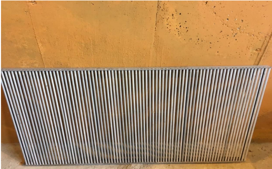
Figure 3.9. View of the rack with clear bar spacing of e_2=6 mm
