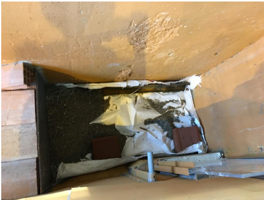
Figure 3.20. Accumulation of sediment (A-2 Group Experiments) within the “Sediment Collection Channel” ( e_1=3 mm, Z_1= 10 cm, Z_2= 25 cm, \alpha=20^\circ )
