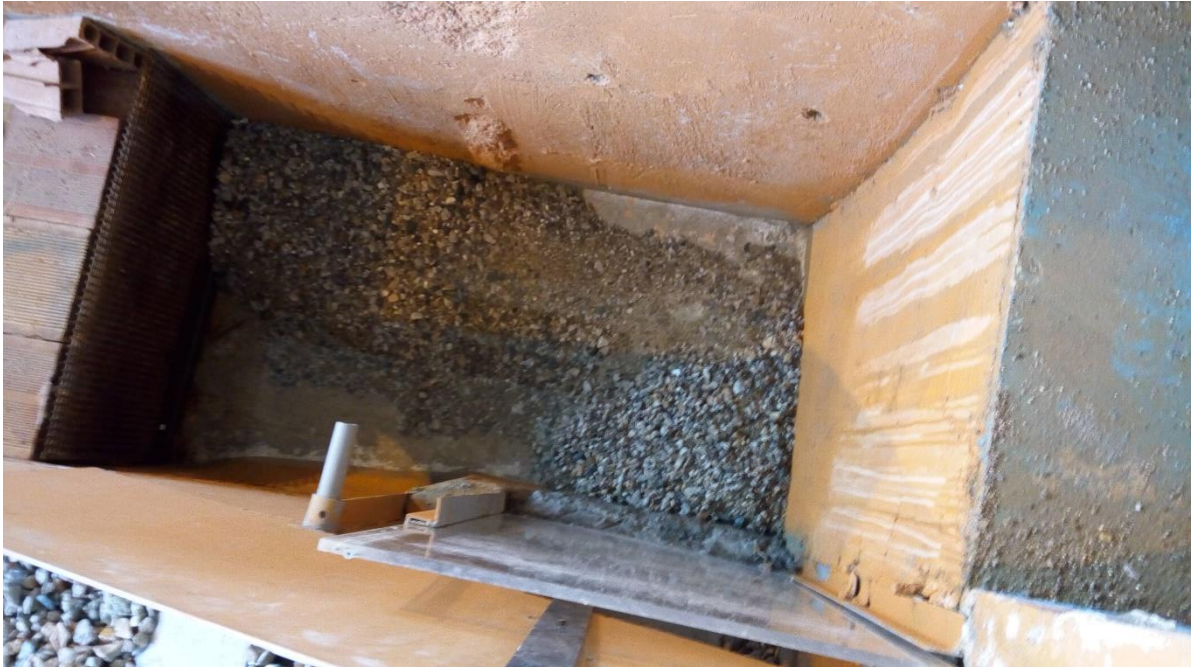
Figure 3.23. Accumulation of sediment (D Group Experiments) within the “Sediment Collection Channel” ( e_4=15 mm, Z_1= 10 cm, Z_2= 20 cm, \alpha=30^\circ )
