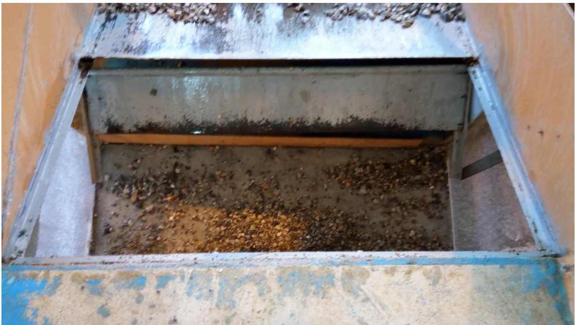
Figure 3.24. Accumulation of sediment (D Group Experiments) within the “Collection Channel-1” ( e_4=15 mm, Z_1= 10 cm, Z_2= 20 cm, \alpha=30^\circ )
