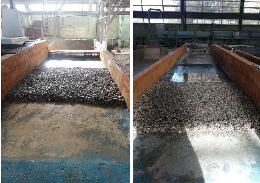
Figure 3.16. A view of the spreaded sediment at the upstream of the main channel before experiments started
