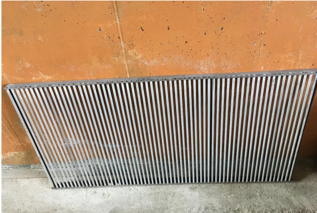
Figure 3.11. View of the rack with clear bar spacing of e_4=15 mm
