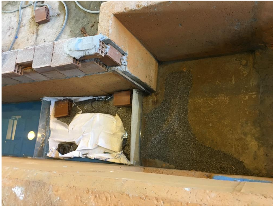
Figure 3.17. Accumulation of sediment (A-2 Group Experiments) at the upstream of the “Intake Channel” ( e_1=3 mm, Z_1= 10 cm, Z_2= 25 cm, \alpha=20^\circ )
