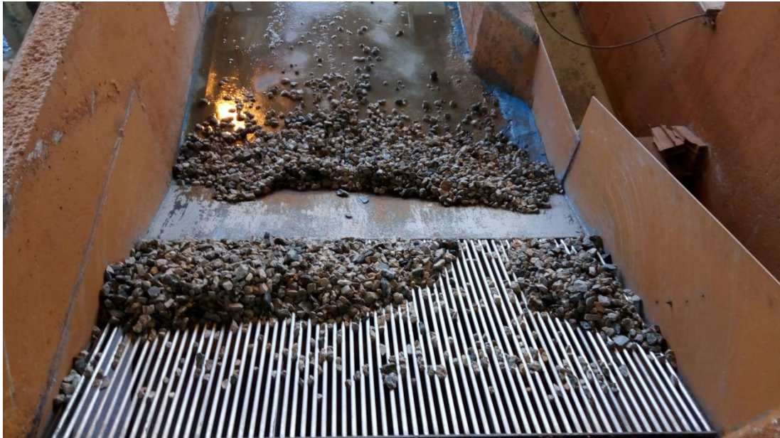
Figure 3.21. Accumulation of sediment (D Group Experiments) within the rack ( e_4=15 mm, Z_1= 10 cm, Z_2= 20 cm, \alpha=30^\circ )
