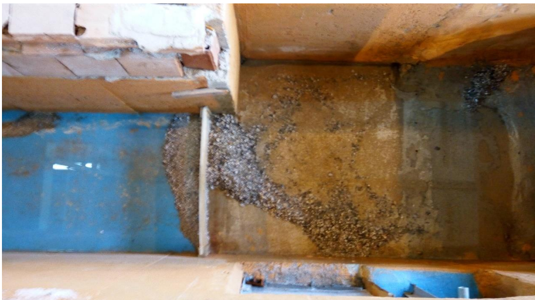
Figure 3.22. Accumulation of sediment (D Group Experiments) at the upstream of the "Intake Channel" ( e_4=15 mm, Z_1= 10 cm, Z_2= 20 cm, \alpha=30^\circ )
