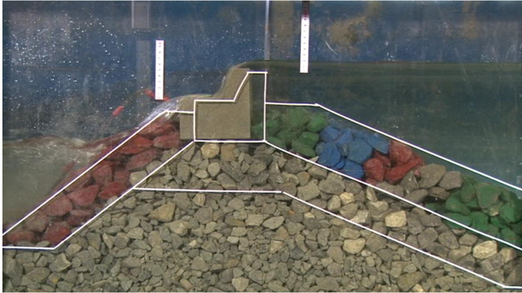
Figure 3.4. Sliding of the Crown-Wall in the Tsunami Overflow Experiment on the Original Cross-Section ( h=1.9 cm)
