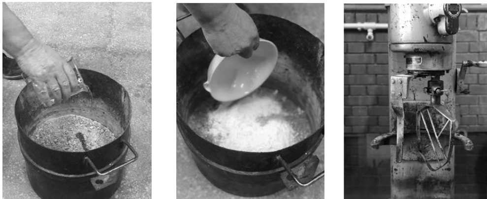
Figure 3.6. Addition of lime to aggregate
