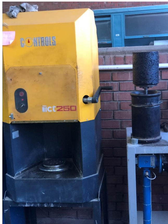
Figure 3.4. Superpave gyratory compactor used in this study
