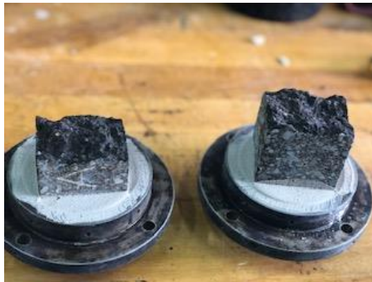
Figure 2.24. Fractured DTT specimen
