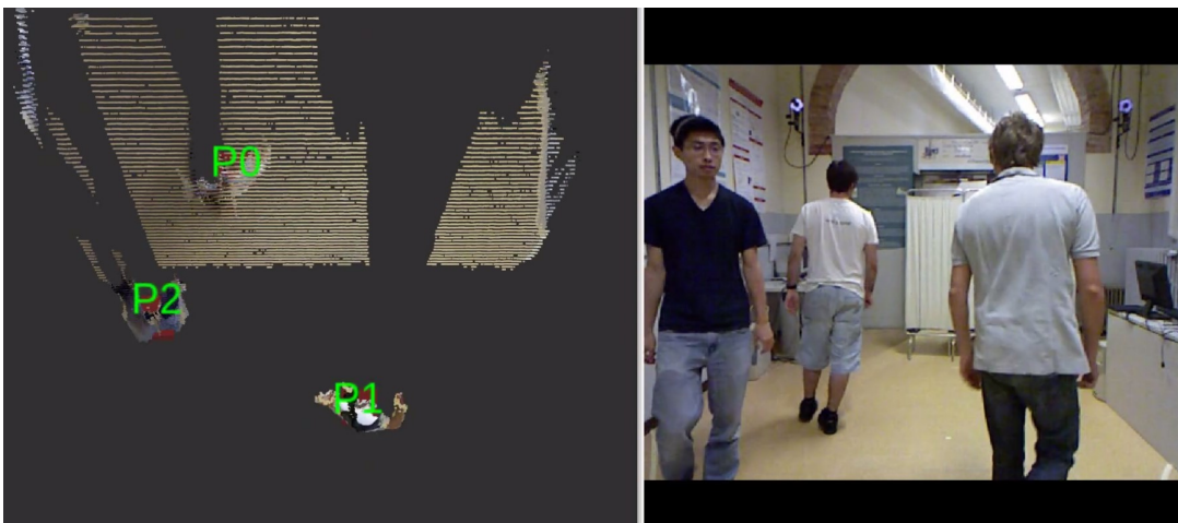
Figure 3.5: Tracker in action. It detects and tracks three people in the scene. Top view and labels are provided on the left.
