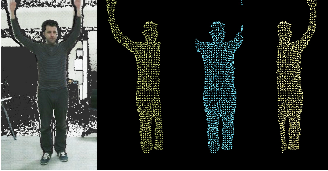
Figure 2.4: Cluster slicing stage with two hands raised (left) and bent (right) cases.
