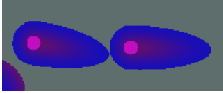
Figure 4.12: Two people moving one after another with defined cost functions. Note the lethal cost circles at human positions.
