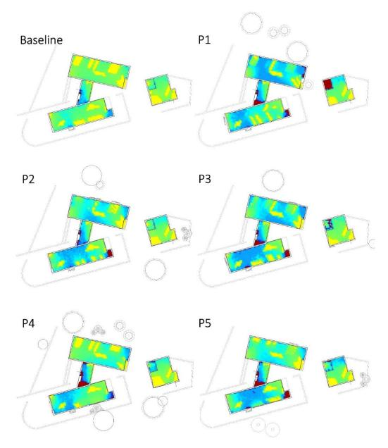
*Figure 5.17.* Daylighting analysis results of the design outputs (where yellow represents high lux values)
