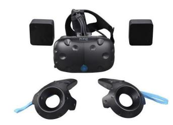
Figure 3.3. HTC Vive components<sup>79</sup>
