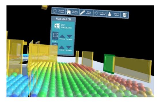
Figure 3.18. Resizing windows according to daylighting simulations
