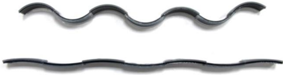
Figure 1.1. 4D Printed expanding strip material to create a sinusoidal strip (Tibbits et al., 2014)
