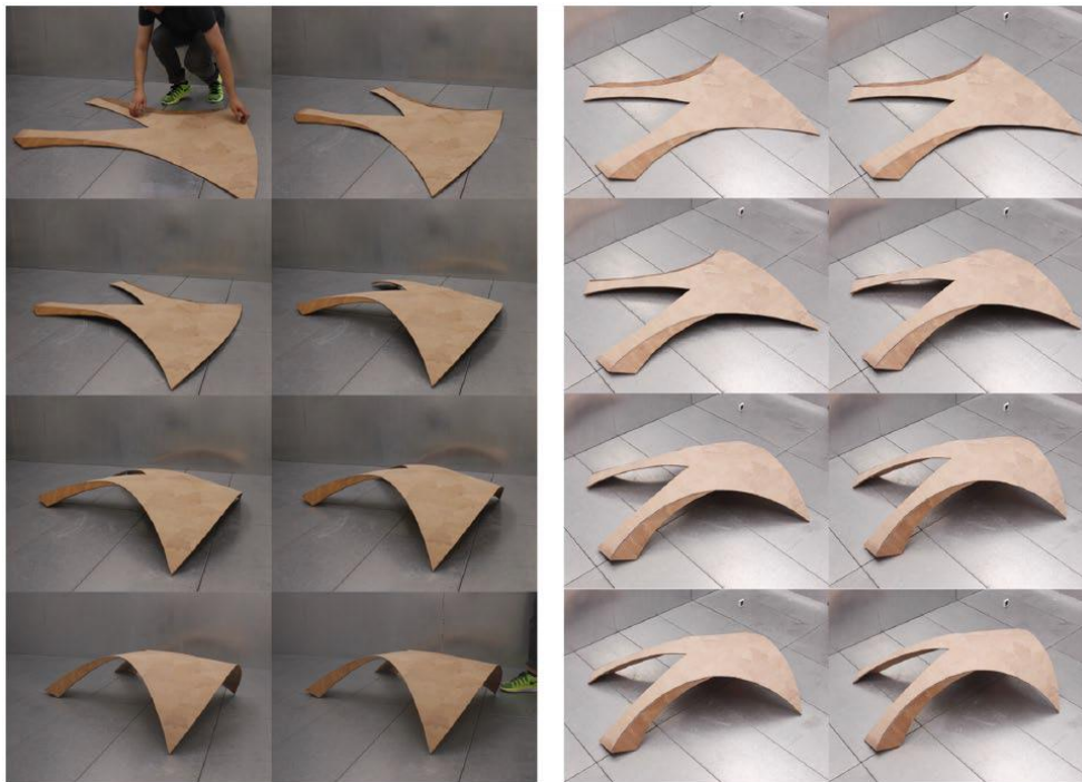
Figure 2.30. Responsive composite timber
