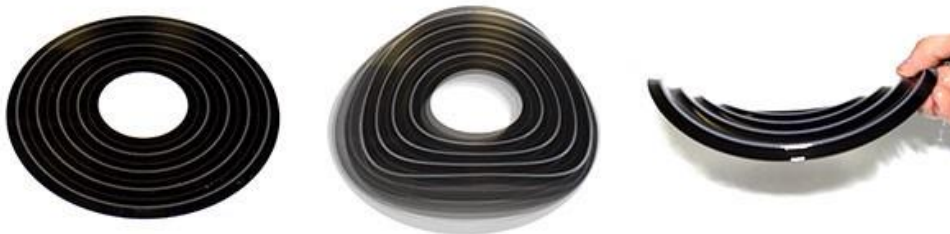
Figure 2.10. 4D Printed Curve-Crease Hyperbolic Paraboloid
