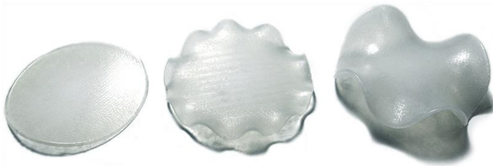
Figure 1.3. 4D printed object with different water submersion phases (Tibbits, McKnelly, Olguin, Dikovsky, & Hirsch, 2014).
