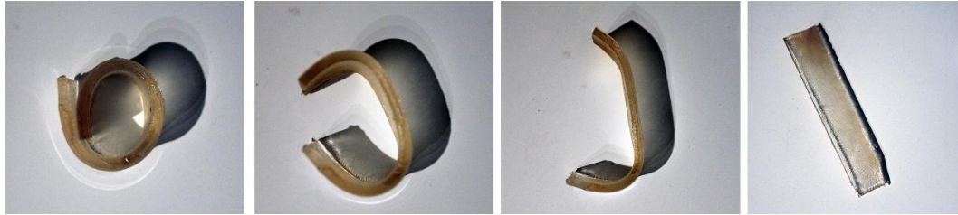
Figure 2.33. Initial test of SMP responsiveness
