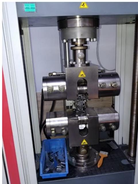
*Figure 3.9. INSTRON tensile test machine.*
