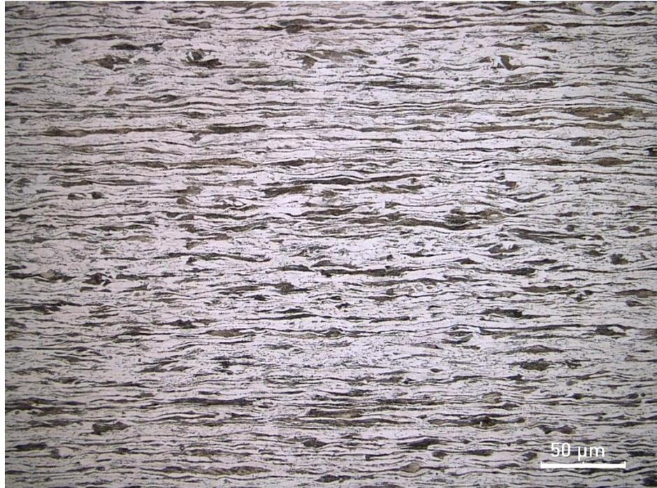
*Figure 4.9. 60% CR specimen before heat treatment.*
