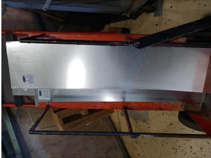
Figure 3.4. Flat samples taken after cold rolling.
