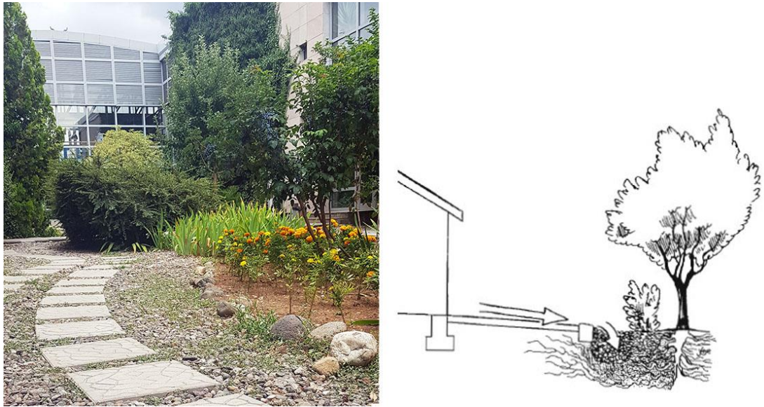
Figure 4.12. An example of french drain with gravel- ODTU Teknokent (Personal Archive,2019) (left) French drain infiltrating intercepted runoff from a roof and patio (Lancaster,2006) (right)
