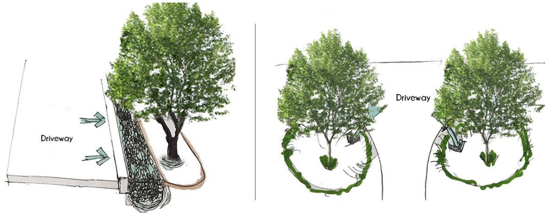
Figure 4.33. A pipeless french drain beside a driveway (left) and tree pits (right) (Illustrated by author,2019)
