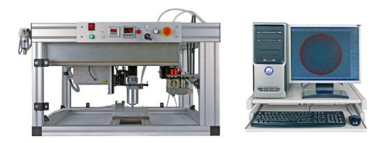
Figure 3.11. Bioscaffolder® 3D printing system.
