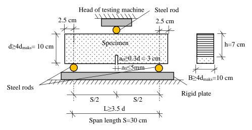
*Figure 3.24* Geometry of three-point bending fracture test specimen and loading apparatus (JCI-S-001-2003)
