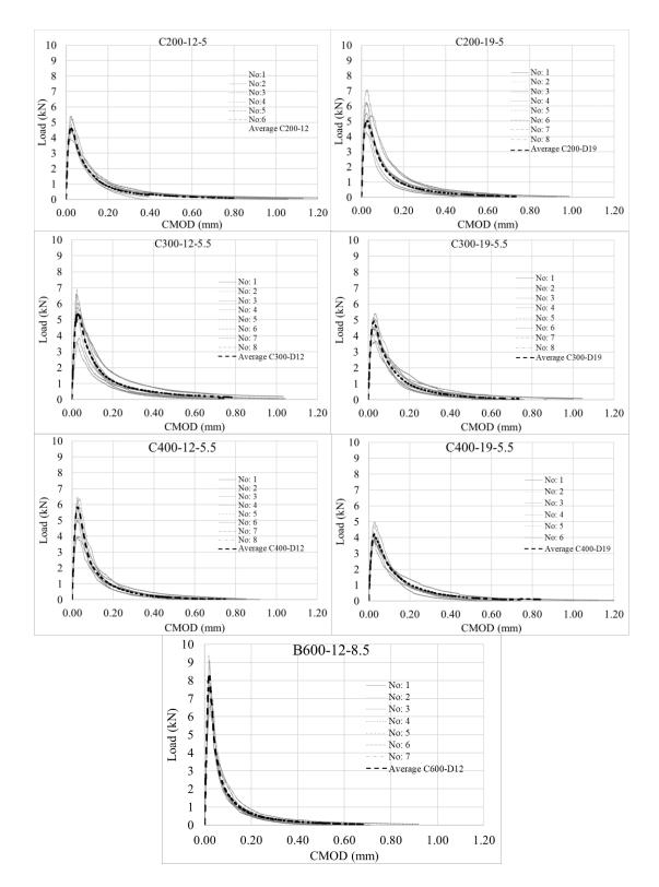
Figure 4.29. Load-CMOD curves for each RCC mixtures obtained by JCI procedure.
