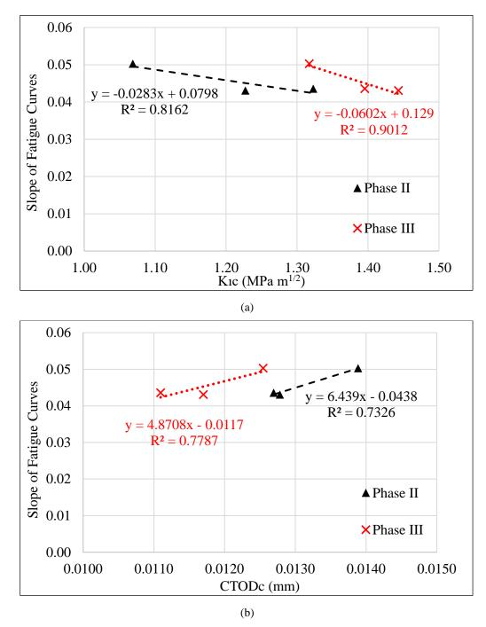
Figure 4.44. The relations between slopes of fatigue curves and fracture parameters (a)  $K_{IC}$  (b) CTOD<sub>c</sub> obtained from Phase II and Phase III
