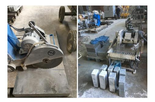
*Figure 3.30.* RCC plate prepared for fatigue test and test specimens of 10x15x35 cm<sup>3</sup>cut from plate (C400-D12-W5.5)
