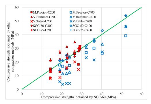
*Figure 4.11.* Comparison of compressive strengths obtained from the first four compaction methods with reference to SGC (60 gyrations) (red 200 kg/m<sup>3</sup> - blue 400 kg/m<sup>3</sup>)
