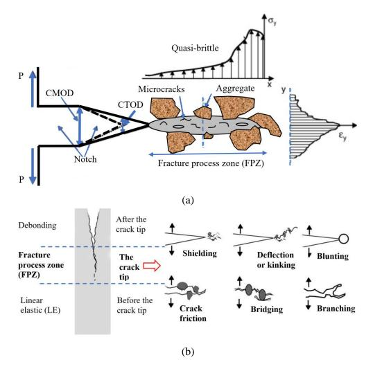
*Figure 2.4.* a) Concept of FPZ (Kim & Buttlar, 2009), b) Mechanisms of crack propagation for concrete (Akkaya et al., 2003; Jimenez Pique, 2002)
