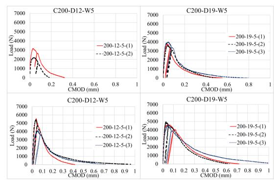
(a) 200 kg/m<sup>3</sup> binder dosage RCC mixture (tests were repeated with new mixture due to damage of the sample before the test)
