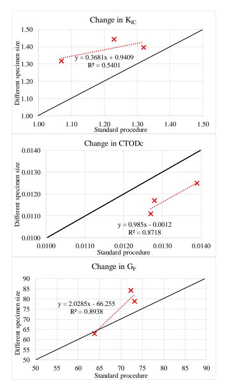
*Figure 4.43.* Comparison of fracture parameters obtained by standard specimen sizes and fatigue specimen sizes for the same mixtures
