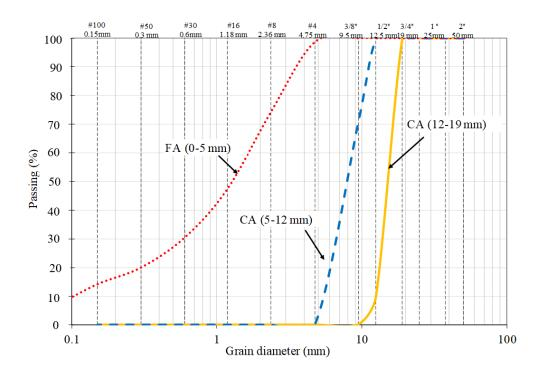
Figure 3.1. Fine and coarse aggregates gradation
