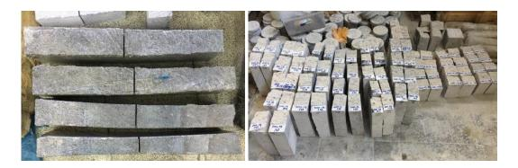
*Figure 3.28.* Some RILEM beam samples that could not be adequately obtained due to difficulties encountered during cutting and sample views after the test
