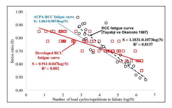
*Figure 4.37.* A comparison between the fatigue curve developed in this study and the fatigue curve obtained by Tayabji & Okamoto, (1987) and ACPA (Roden, 2013)
