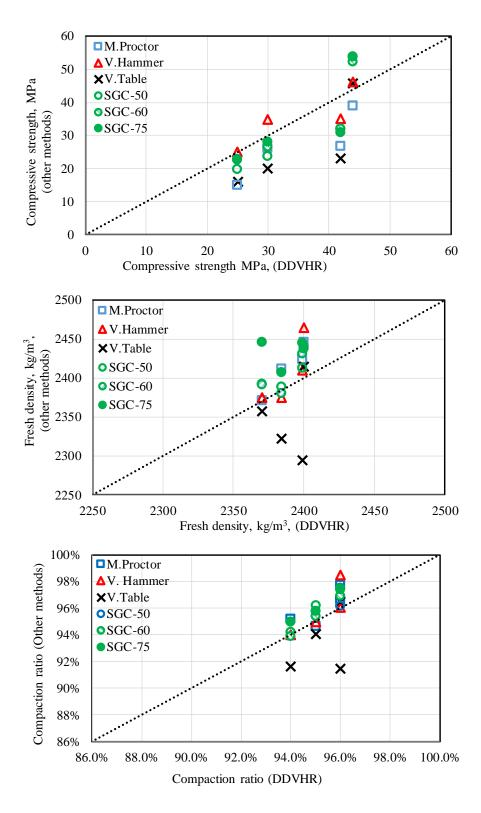
*Figure 4.16.* Comparison of the results obtained from the DDVHR with the other four laboratory compaction methods a) 28-day compressive strength b) density c) compaction ratio
