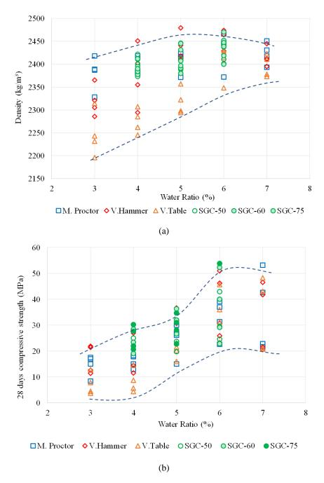
*Figure 3.12.* (a) Density- water ratio (b) 28-day compressive strength- water ratio relationships for RCC design mixtures.
