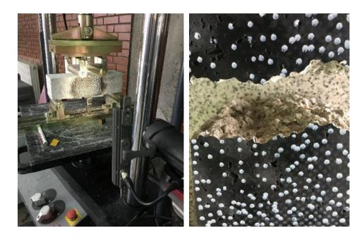
Figure 4.20. Determination of flexural strength of RCC mixtures according to ASTM C78.
