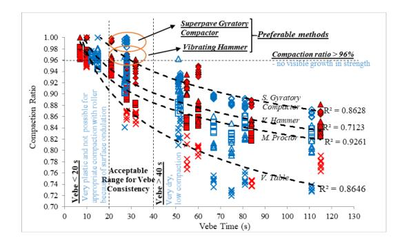
*Figure 4.15.* Vebe time and compaction ratio relationship (red 200 kg/m<sup>3</sup> - blue 400 kg/m<sup>3</sup>).
