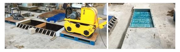
Figure 3.15. Wood and steel molds used for DDVHR
