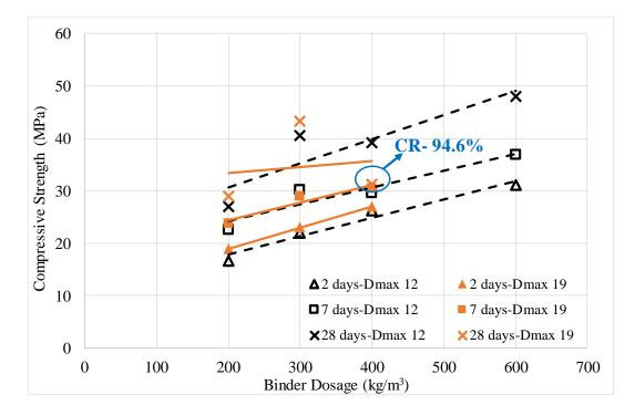
*Figure 4.18.* Relationship between cement dosage and compressive strength of 2, 7 and 28 days for DDVHR.
