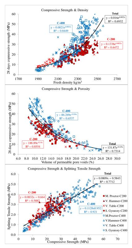
*Figure 4.1.* Relationship between 28-day compressive strength and density, porosity, 28-day splitting tensile strength (red 200 kg/m<sup>3</sup> - blue 400 kg/m<sup>3</sup>)
