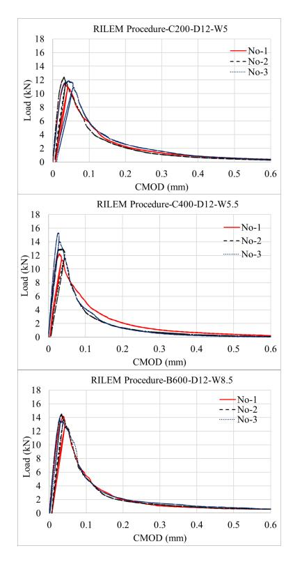
*Figure 4.42.* Load-CMOD graphs obtained by three-point bending beam specimens with dimension of 10x15x35 cm<sup>3</sup> for each mixture according to the RILEM procedure (RILEM TC-89 FMT 1990)
