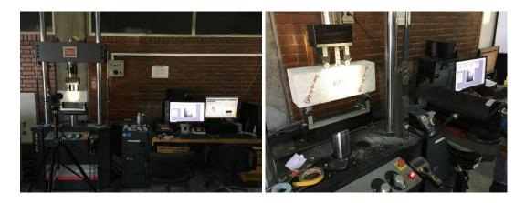
Figure 3.31. Photos from four-point flexural beam fatigue testing (C200-D12-W5).
