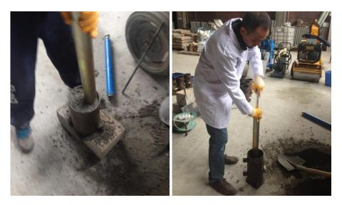
Figure 3.5. Compaction of RCC mixtures by modified proctor method (ASTM D1557)
