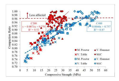
Figure 4.13. Relationship between compressive strength and compaction ratio for RCC mixtures (red  $200 \text{ kg/m}^3$  - blue  $400 \text{ kg/m}^3$ )
