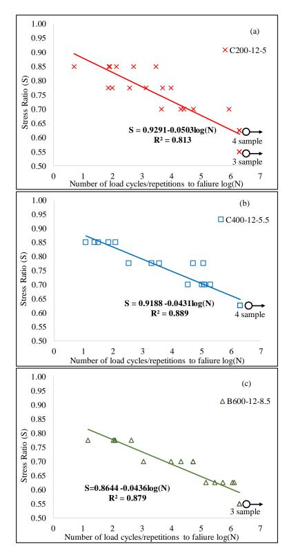
*Figure 4.35.* S-N curve for each RCC mixture under flexural fatigue loading (a) 200 kg/m<sup>3</sup> binder dosage (b) 400 kg/m<sup>3</sup> binder dosage (c) 600 kg/m<sup>3</sup> binder dosage
