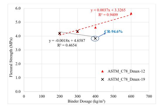
Figure 4.21. Relationship between binder dosage and flexural strength.
