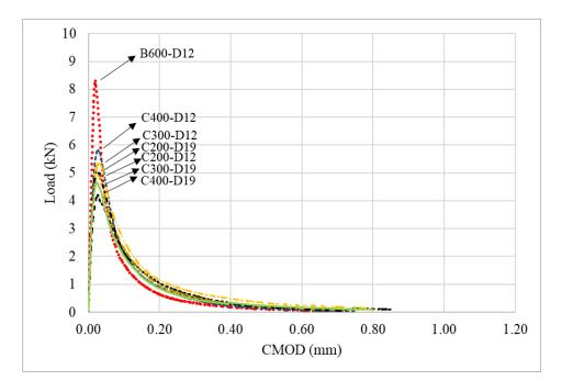
Figure 4.30. Average Load-CMOD curves for RCC mixtures.
