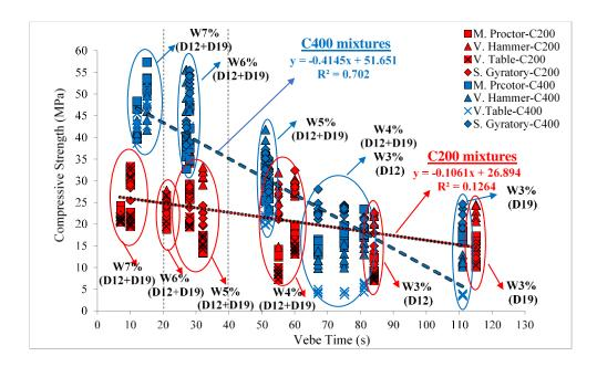
Figure 4.12. The relations between the compressive strength and Vebe time of all RCC mixtures. (red  $200 \text{ kg/m}^3$  - blue  $400 \text{ kg/m}^3$ )
