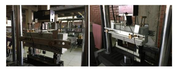
Figure 4.40. Determination of fracture parameters in the third phase of the experimental study
