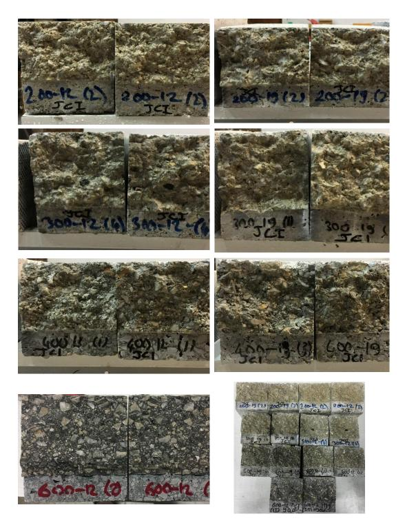
Figure 4.32. Typical fractured surface of the samples at the end of the JCI test procedure.
