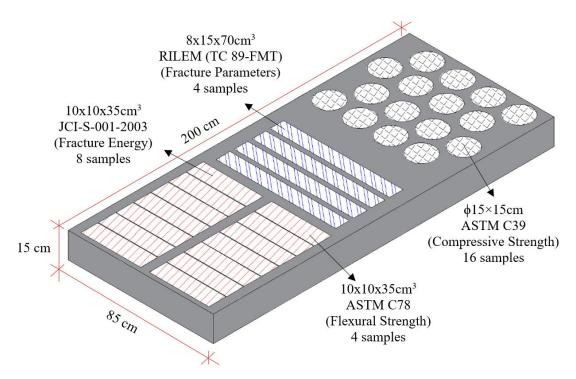
*Figure 3.22.* Cutting plan of core and beam samples on the plate to determine compressive and flexural strength and fracture parameters of each RCC mixture
