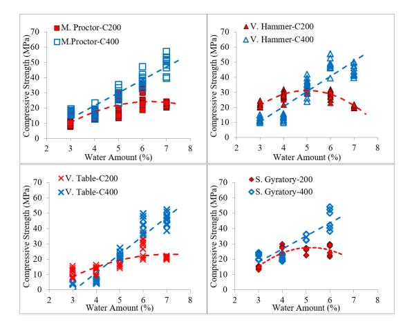
*Figure 4.5.* Relationship between water amount and compressive strength at 28 days for each compaction method
