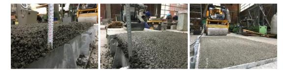
*Figure 3.21*. Application of VPC and DDVHR for RCC mixtures in the second phase of experimental study
