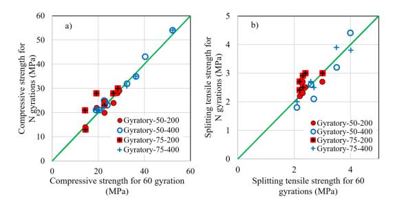
*Figure 4.7.* a) Compressive strength comparison with respect to gyration numbers, b) Splitting tensile strength comparison with respect to gyration numbers (red 200 kg/m<sup>3</sup> - blue 400 kg/m<sup>3</sup>)
