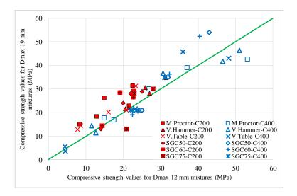
*Figure 4.2.* A comparison between the compressive test results based on the maximum aggregate sizes for the same RCC mixtures (red 200 kg/m<sup>3</sup> - blue 400 kg/m<sup>3</sup>)
