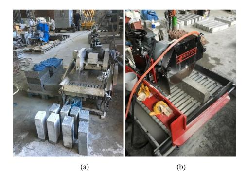
*Figure 3.27.* Preparation of beam specimens and notching, the example of (a) the cutting of JCI-S-001 beam specimen (b) the notching of the RILEM TC 89-FMT beam specimen
