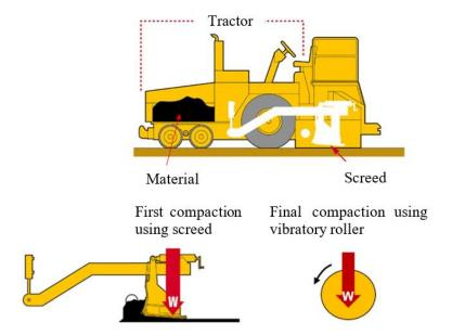
Figure 3.14. Typical compaction process for asphalt paver
