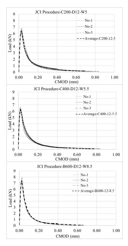
*Figure 4.41.* Load-CMOD graphs obtained by three-point bending beam specimens with the dimension of 10x15x35 cm<sup>3</sup> for each mixture according to the JCI procedure (JCI-S-001 2003).
