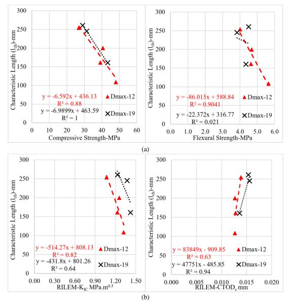
*Figure 4.34.* The relationship between characteristic length and (a) strengths, (b) RILEM fracture parameters in RCC mixtures.
