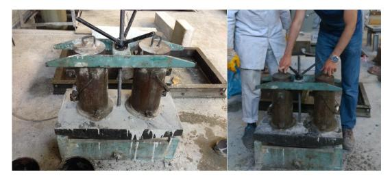
Figure 3.7. Compaction of RCC mixtures by vibrating table method (ASTM C1176).
