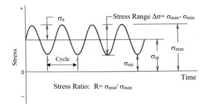
Figure 2.5. Typical sinusoidal constant amplitude fatigue load
