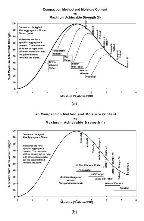
*Figure 2.2.* The maximum allowable strength vs. moisture content curve with respect to compaction techniques (Schrader, 2003)
