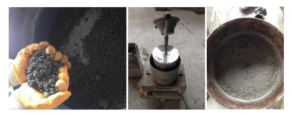
Figure 3.4. RCC mixture consistency and applied Vebe test
