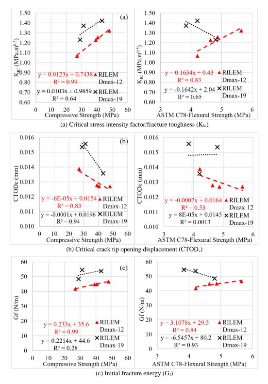
*Figure 4.26.* Relationship between strengths and fracture parameters, (a) critical stress intensity factor, (b) critical crack tip opening displacement, (c) initial fracture energy
