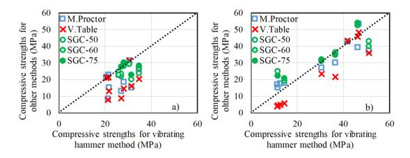
*Figure 4.10.* Comparison of compressive strengths obtained from the first four compaction methods w.r.t vibrating hammer a) 200 kg/m<sup>3</sup> cement dosage b) 400 kg/m<sup>3</sup> cement dosage
