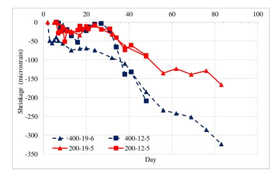
Figure 4.17. The shrinkage results obtained from RCC specimens.
