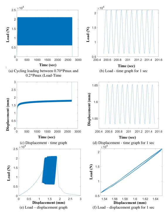
Figure 3.32. Typical results from fatigue test (between  $0.70^*P_{max}$  and  $0.20^*P_{max}$ ) applied on a specimen 10 times per second. (Number of cycles to failure =26776).
