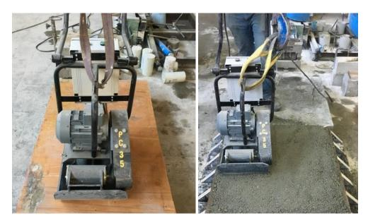
*Figure 3.16.* Vibratory plate compactor (VPC) application representing field paver compaction process prior to DDVHR application for RCC mixtures
