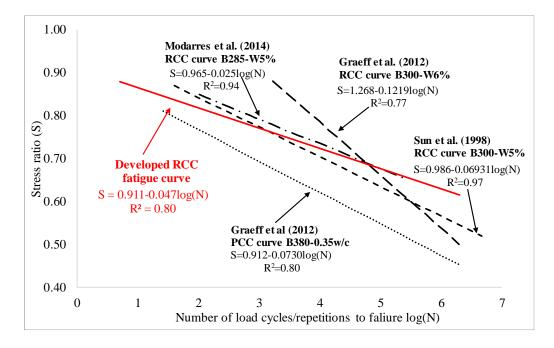
*Figure 4.38.* Comparison of developed RCC fatigue curve with current RCC fatigue curves in the literature (B: binder content (kg/m<sup>3</sup>; W: water ratio by weight, w/c: water to cement ratio)
