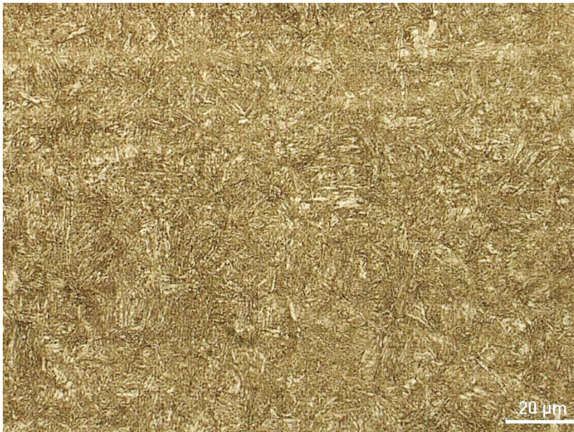
Figure 4.9. The optical micrograph of tempered martensite. (450°C, 1,5hr)
