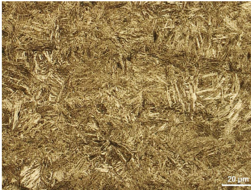
Figure 4.19. Optical micrograph of isothermally treated sample at M_{50} 270°C for 3 hrs
