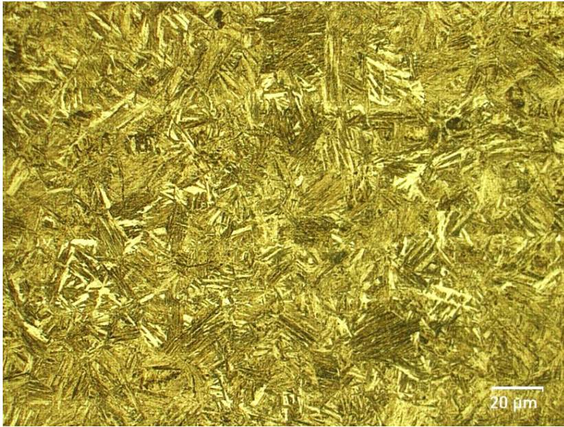
Figure 4.15. Optical micrograph of isothermally held sample at 270°C for 80 min.
