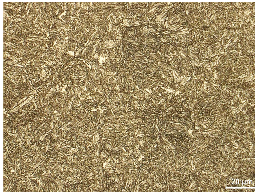
Figure 4.11. The optical micrograph of tempered martensite. (550°C, 1,5hrs)
