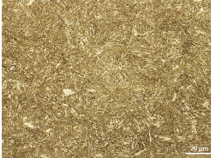
Figure 4.10. The optical micrograph of tempered martensite. (500°C, 1,5hr)
