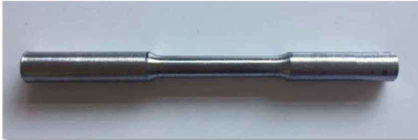
Figure 3.3. Tensile test specimen machined from 55Cr3 according to ASTM E8/E8M-16a
