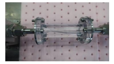
Figure 3.1: Venturi made from Plexiglass
