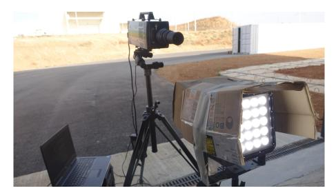
Figure 3.8: Light Source and High Speed Camera
