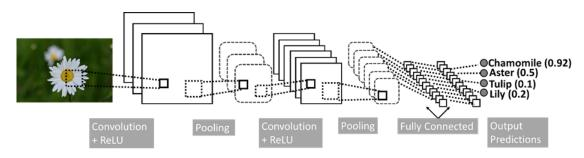
Figure 42: A simple CNN model. The output is one of the four flowering plants, image adapted from LeCun et al., 1998
