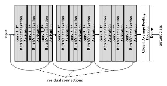
Figure 49: Simplified ResNet architecture with batch normalization, regularization, and pooling. There is a convolution between blocks and a residual connection between the last item of the previous block and the current one, which means the training in between layers is omitted. \* L2 kernel and L2 bias regularizers are applied.
