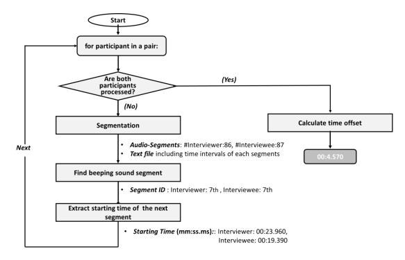
Figure 5: The flow chart of the synchronization process. Values of first pair are presented.
