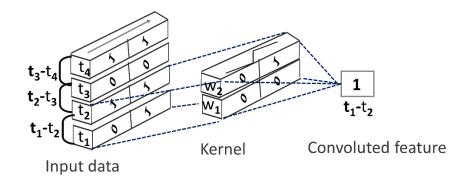
Figure 44: Illustration of the convolution operation for time series data. Input shape is (1,4,2), i.e., one sample of four time points, each item having two channels. The kernel shape is (2,2).
