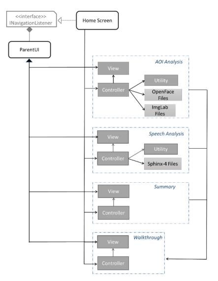
Figure 18: The Software architecture of MAGiC.
