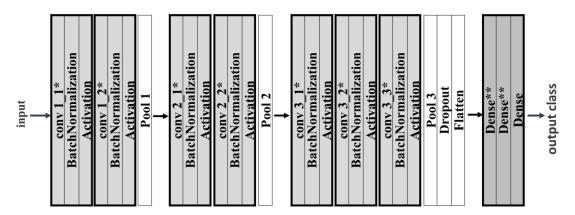
Figure 48: GazeVGG architecture with batch normalization, regularization and pooling. \* L2 kernel and L2 bias regularizers were applied. \*\*L2 kernel regularizer was applied.
