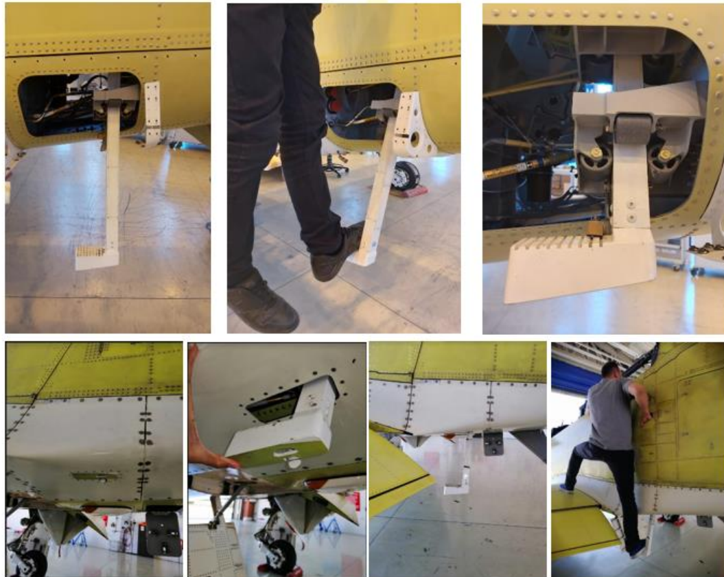
Figure 4.2. An example of boarding step without/with body fairing on aircraft
