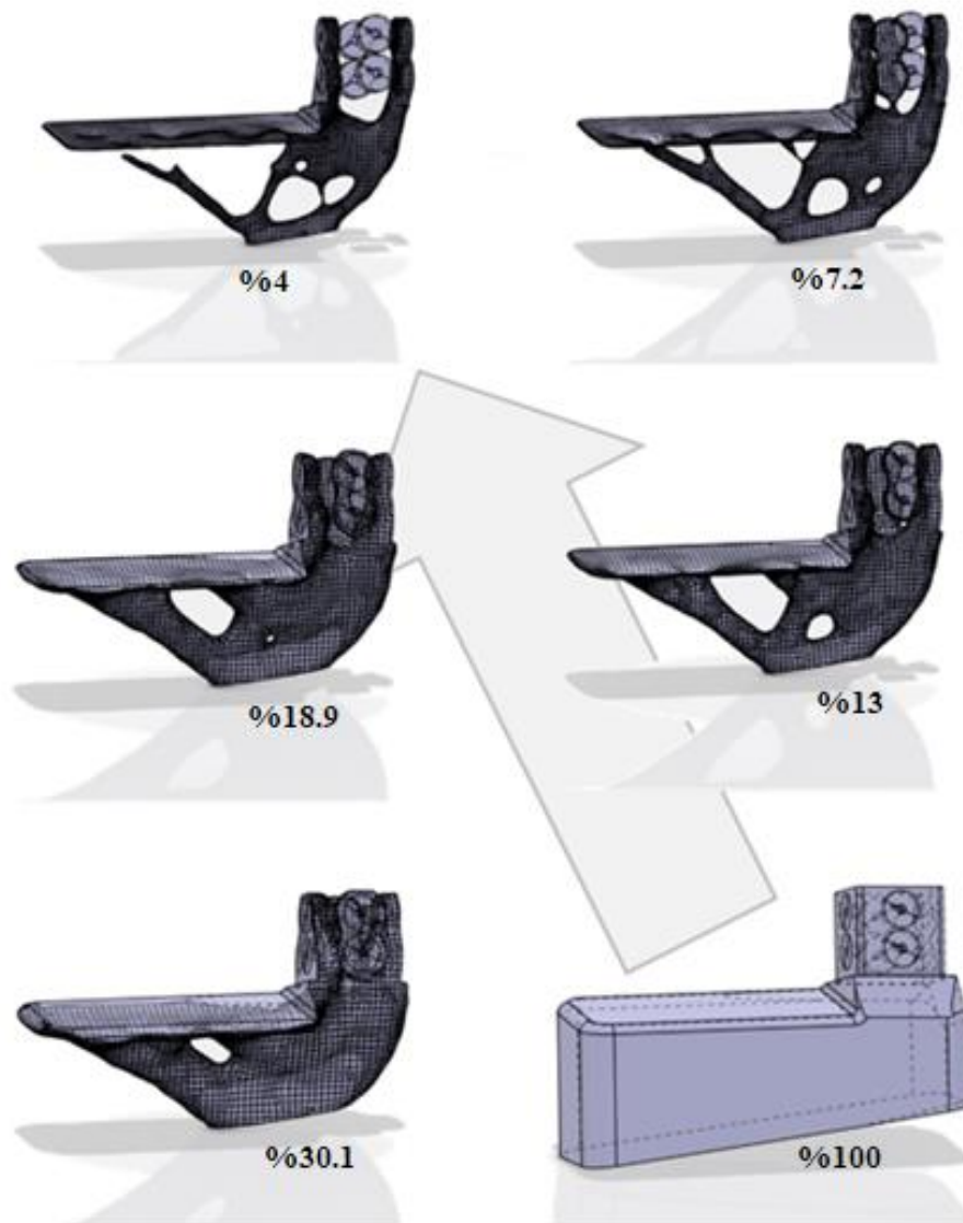
Figure 4.19. Main load carrying elements after smoothing operation. Residual volumes are %4, %7.2, %13, %18.9, %30.1 and %100 from left to right; above to below
