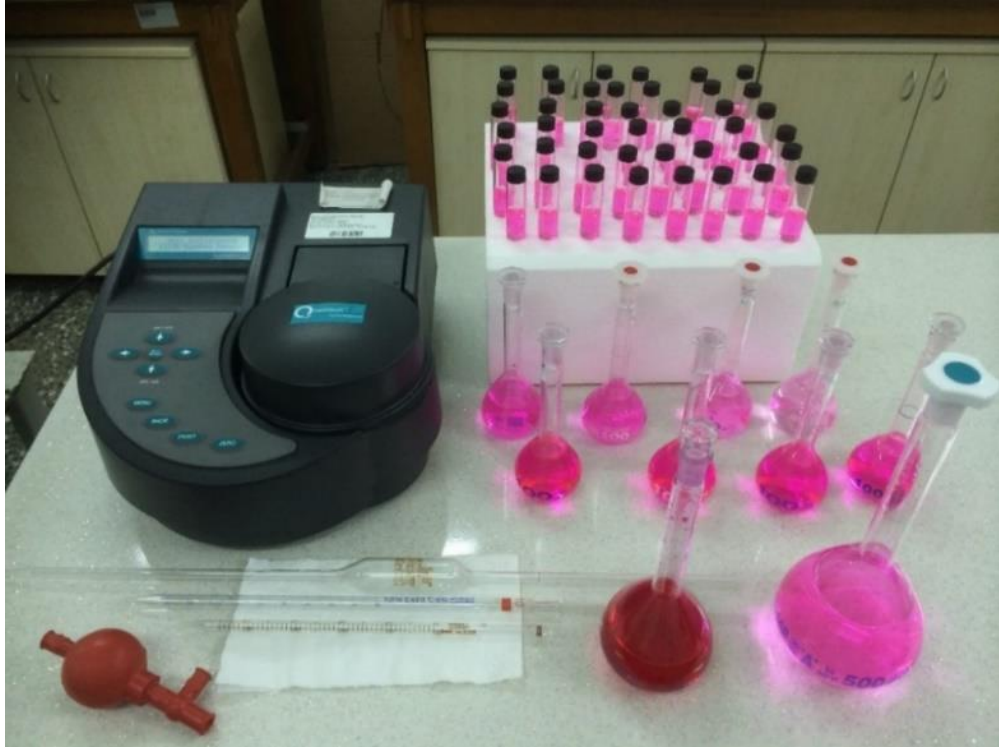
Figure 6.8. Rhodamine B solutions and the fluorescence spectrometry
