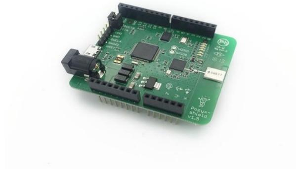
*Figure 6.13 Indoor UWB Localization System Unit Pozyx Tag [60]*
