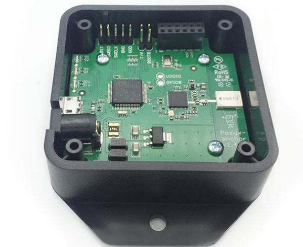
*Figure 6.14 Indoor UWB Localization System Unit Pozyx Anchor [60]*
