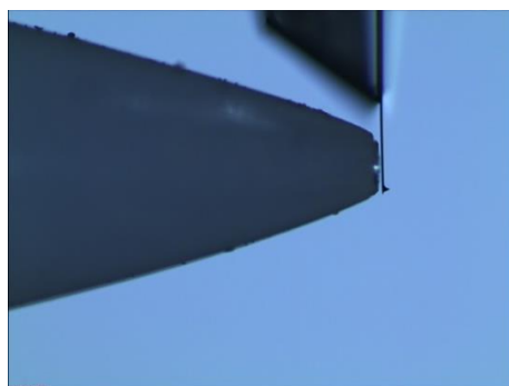
Figure 3. 15 Alignment holder of the cantilever in front of the fiber tubing
