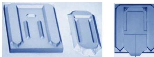
Figure 3. 14 Cantilever Alignment holder chip and cantilever.
