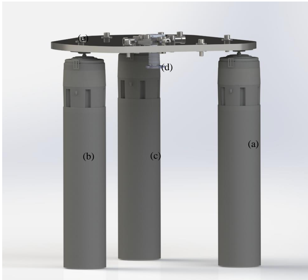
Figure 5. 7 The vibration isolation table schematic design. (a), (b), and (c) are air damping isolation legs, (d) is an edge welded bellows, (e) platform.
