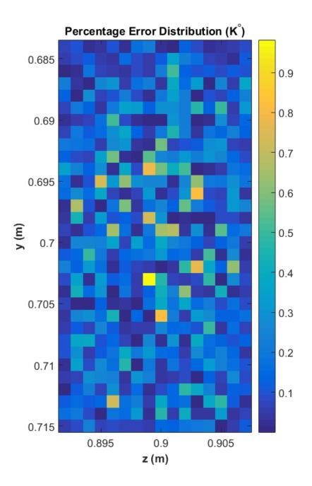
Figure 3.20: Error Distribution between the original temperature distribution and the estimated temperature distribution when SNR is 60 dB.
