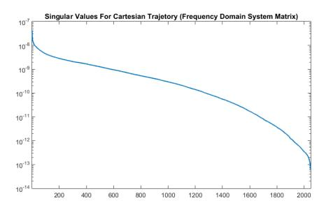
Figure 2.22: Sorted singular values for the system matrix that obtained from Cartesian Trajectory. Maximum and minimum values are  $4.196 \times 10^{-8}$  and  $6.121 \times 10^{-14}$  respectively. The condition number is then found to be approximately  $6.855 \times 10^{5}$ .
