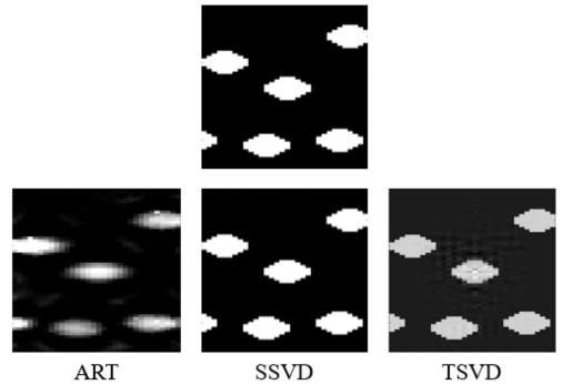
Figure 2.32: Results for Lissajous Scanning Trajectory, without any additional noise. PSNR values for ART, SSVD and TSVD are 8.38, 283.55, 57.95 respectively.
