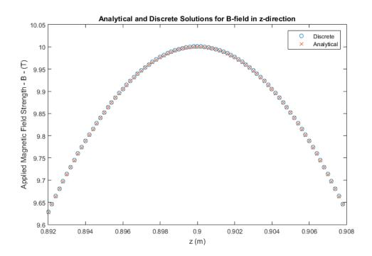
Figure 2.9: Compared B-field values for analytical and discrete computations. As the coil center was set to be at z = 0.9 meter, the B field reaches its maximum value around z = 0.9. The maximum relative error calculated between the analytical and the discrete solutions was approximately 0.6 percent.
