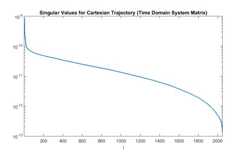
Figure 2.15: Sorted singular values for the system matrix that obtained from Cartesian Trajectory. Maximum and minimum values are  $8.588 \times 10^{-10}$  and  $1.342 \times 10^{-13}$  respectively. The condition number is then found to be  $6.3979 \times 10^3$ .
