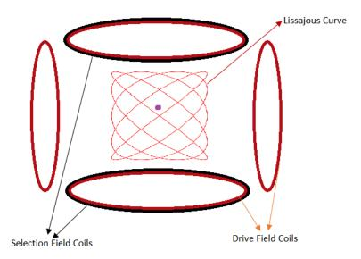
Figure 2.7: Field generating coils. Selection Field coil pair (black) is placed in the z-direction and Drive Field coir pairs (red) are placed in both y and z directions. Small circle in the middle represents a volume of nanoparticles. The shape of the scanning trajectory is represented with the Lissajous Curve lines. The dimensions in this schematic is only for visualization, not reflecting the actual size.
