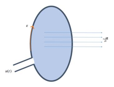
Figure 2.11: Visualization of the concepts that was described in equations (2.11), (2.12) and (2.13). E is the Electric Field through the circular coil,  $\frac{\partial B}{\partial t}$  is the Magnetic Flux Density and u(t) is the voltage signal induced at the ends of the coil.
