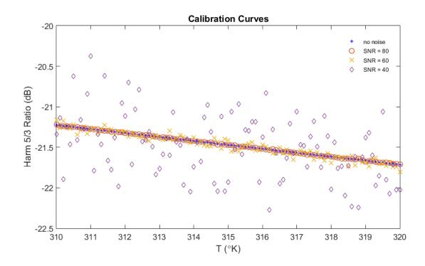
Figure 3.11: Four different calibration curve data, obtained for noise free case and noise added cases when SNR is 80, 60 and 40 dB, respectively. It can be seen that as SNR decreases, data become more dispersed and lose the linear structure. For this reason, one can conclude that the error in temperature estimation would increase as SNR decreases.
