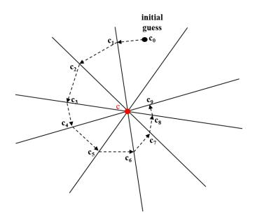
Figure 2.29: Illustrative explanation for the idea behind ART.  $c_0$  is the initial guess and  $c_i$  are the projections on the line equations of the system, which are updated by using equation (2.50). c is the actual particle distribution that is aimed to be approximated by using this method.
