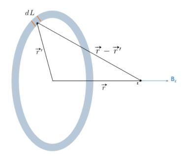
Figure 2.6: Schematic illustration for single circular coil, showing the parameters used in Biot Savart equation that calculates the magnetic field.
