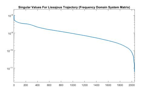
Figure 2.21: Sorted singular values for the system matrix that obtained from Lissajous Trajectory. Maximum and minimum values are  $1.057 \times 10^{-8}$  and  $6.24 \times 10^{-12}$  respectively. The condition number is then found to be approximately  $1.69 \times 10^3$ .
