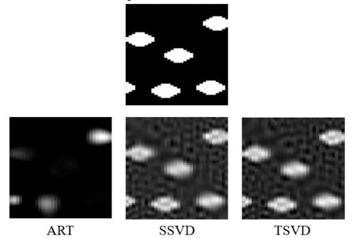
Figure 2.37: Results for Lissajous Scanning Trajectory, with  $SNR = 34 \, dB$  additional noise. PSNR values for ART, SSVD and TSVD are 8.07, 17.2133, 17.4243 respectively.
