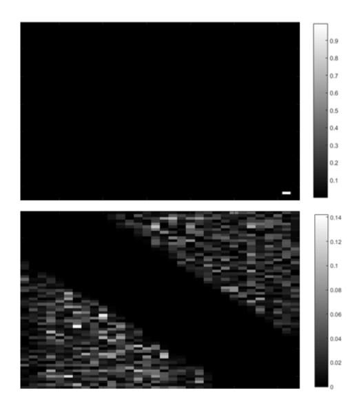
Figure 2.16: Image basis vectors transformed to 2D image that correspond maximum (upper) and minimum (lower) singular values that are obtained from Lissajous Scanning.
