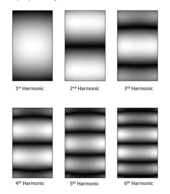
Figure 2.27: Spatial Frequencies for y-channel System Matrix that is obtained from Cartesian Trajectory scan.
