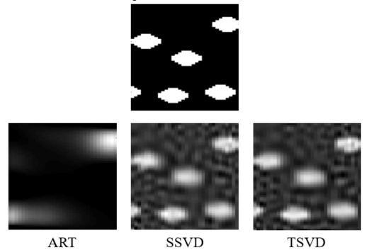
Figure 2.36: Results for Cartesian Scanning Trajectory, with  $SNR = 34 \ dB$  additional noise. PSNR values for ART, SSVD and TSVD are 7.13, 17.2133, 16.0055 respectively.
