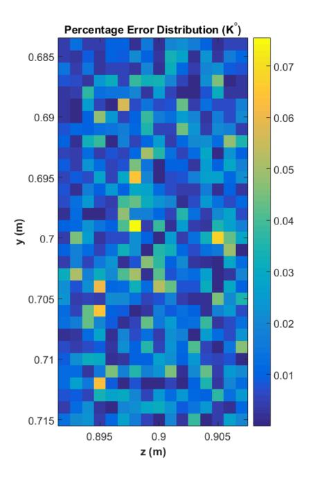
Figure 3.19: Error Distribution between the original temperature distribution and the estimated temperature distribution when SNR is 80 dB.
