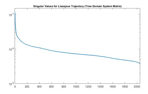
Figure 2.14: Sorted singular values for the system matrix that obtained from Lissajous Trajectory. Maximum and minimum values are  $1.133 \times 10^{-7}$  and  $3.729 \times 10^{-9}$  respectively. The condition number is then found to be approximately 30.38.
