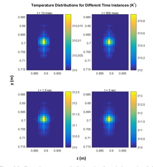
Figure 3.5: Change in temperature distribution when focused ultrasound applied in the imaging area fordifferent durations between 10 ms and 2 seconds, along y-direction.
