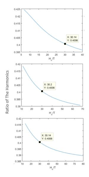
Figure 3.6: Plots showing changes in the Ratio of Harmonics with respect to  $H_0/T$ . All of the three plots were obtained from 0-D simulations with only one excitation field with frequency 1470Hz. From upper to the lower graphs, the amplitude of the applied field increases.
