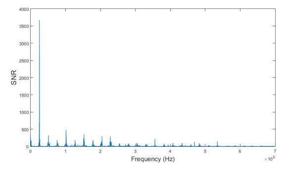
Figure 2.33: SNR values for different frequencies. Maximum SNR value is found to be approximately 34 dB and it can be seen that SNR value increases at signal harmonics. Comparing these results with experimental data given in [3], it can be concluded that 34 dB SNR level is acceptable as 40dB SNR was observed experimentally for 200 averages.
