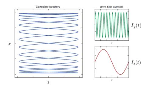
Figure 2.12: Schematic presentation for the Cartesian Trajectory [2].
