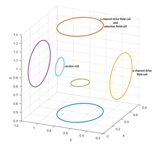
Figure 2.10: Complete coil configuration that was used in the MPI simulation. Drive and Selection field coils placed on the x-y plane have the same position, therefore they are not *visually* distinguishable, but the pairs are represented with dark blue and red circles in the figure. Drive Field coil pair of the y-channel is represented with purple and yellow circles. Lastly, the y-sensitive and z-sensitive Receive coils are represented with light blue and green circles, respectively.
