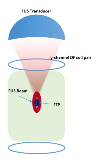
Figure 3.1: Schematical illustration for the setup that has been modelled in this study. Focused ultrasound was modelled to be applied in y-direction in the imaging plane.
