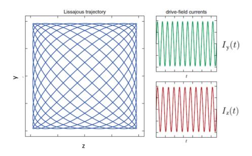
Figure 2.13: Schematic presentation for the Lissajous Trajectory [2].
