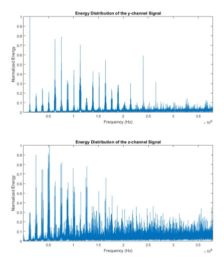
Figure 2.20: Energy distribution of y and z- channel system functions for frequencies between 0 to 4000 kHz, that was obtained from Cartesian Scanning. It can be seen that the energy is dominant at harmonic frequencies.
