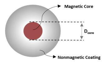
Figure 2.1: Schematic drawing of a typical magnetic nanoparticle. The diameter  $D_{core}$  of the magnetic core ranges between 1 - 100 nm. When the diameter of the nonmagnetic coating is thick enough, the nanoparticle shows 'superparamagnetic' behaviour, having single magnetic domain and a high magnetic moment. This provides a better tracking of magnetization of the MNPs.
