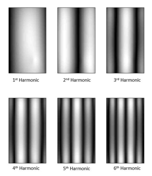
Figure 2.28: Spatial Frequencies for z-channel System Matrix that is obtained from Cartesian Trajectory scan.
