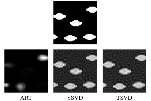
Figure 2.34: Results for Cartesian Scanning Trajectory, with  $SNR = 50 \ dB$  additional noise. PSNR values for ART, SSVD and TSVD are 8.07, 19.3686, 19.5740 respectively.
