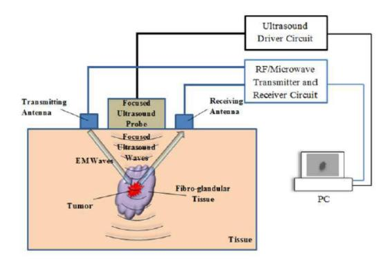
Figure 1.1: Illustration of the HMMDI system [1]. Local vibrations that cause the harmonic motion are generated by the focused ultrasound probe. RF/Microwave Transmitter and Receiver Circuit basically generates microwave signals and detects the backscattered signal amplitude at the Doppler frequency.
