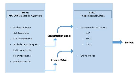
Figure 2.5: Steps for the realistic MPI simulation. Scheme shows the inputs and outputs of the first and second step blocks. The outputs for the first step is a realistic Magnetization signal data and a System Matrix that will both be used in the second step, while reconstructing the image.
