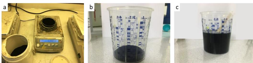
Figure 6: Suspension preparation a) Measurement of MWCNT in dust condition, b) MWCNT in pouring container c) MWCNT hand mixed into epoxy in pouring container
