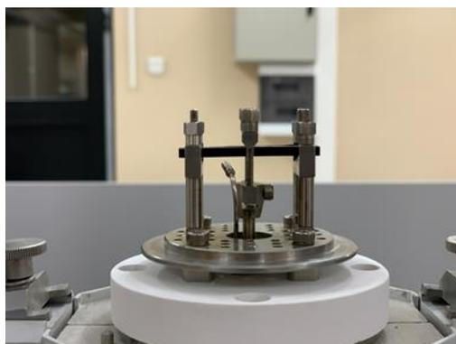
*Figure 23: 3-point bending test fixture with located specimen for DMA*
