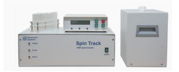
Figure 2. 4. Nuclear Magnetic Resonance (NMR) Relaxometry device
