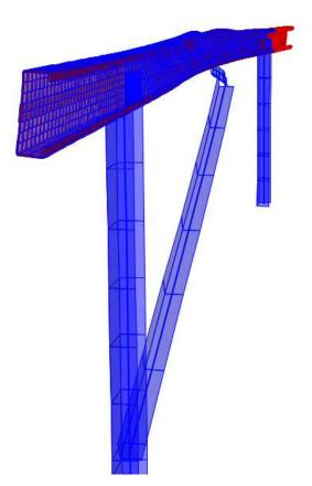
Figure 39- Buckling of Main Beam under Dead Load+Snow Load
