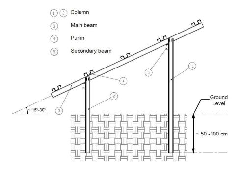
Figure 33- Typical View of PV Mounting Structures
