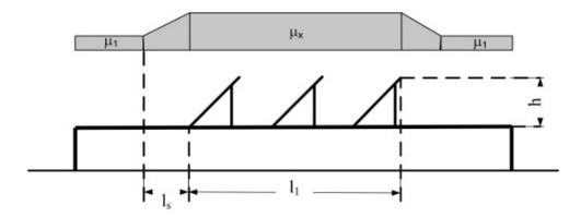
Figure 8- Shape Coefficient and Drift Length for Flat Roofs with PV Panels suggested by Formichi (2019)
