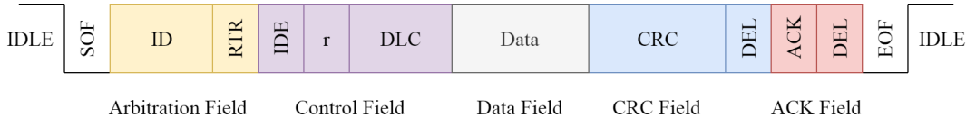
Figure 2.2: A Typical Controller Area Network Frame
