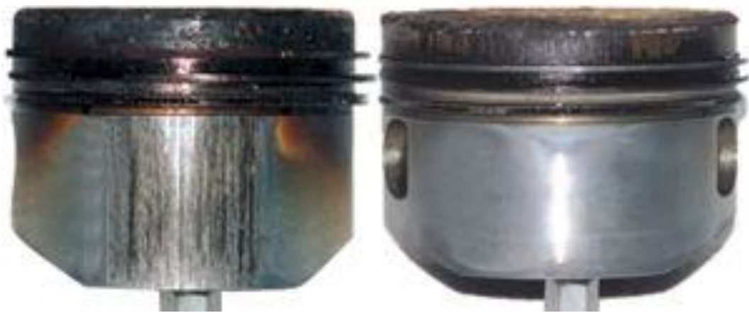
Figure 4.7. The example of damaged pistons [51].
