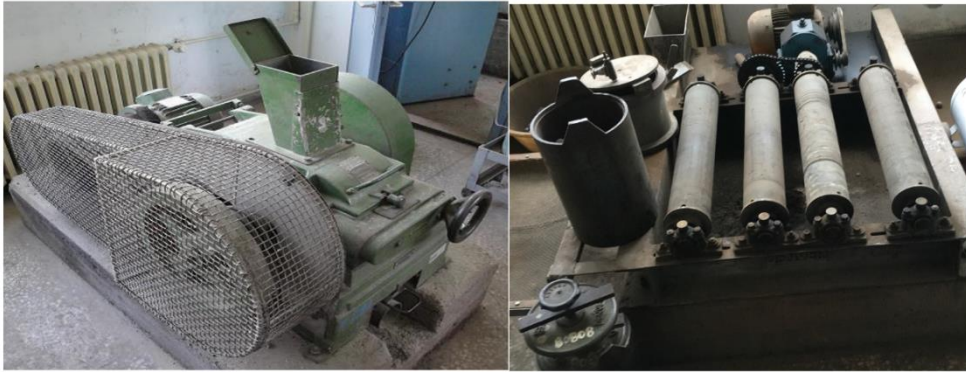
Figure 3.1. One roller crusher (Right) and ball-mill crusher (Left)
