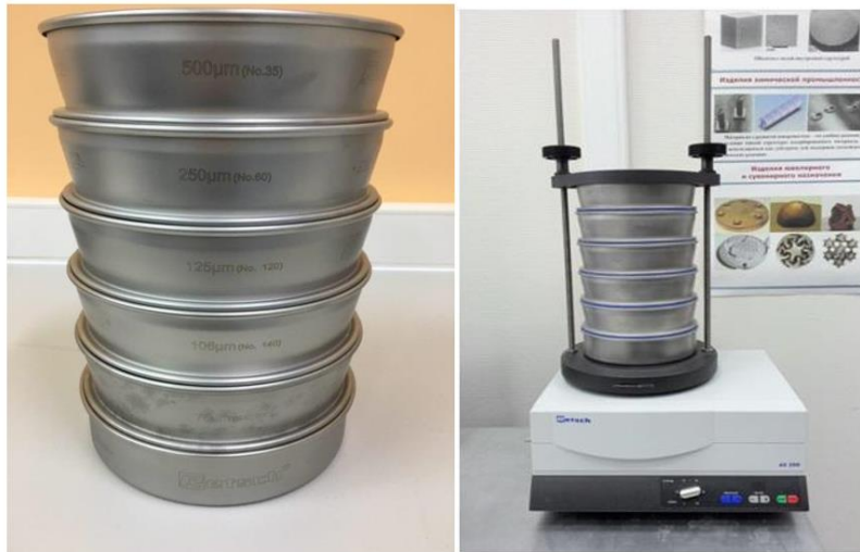
Figure 3.2. Retsch brand sieve set and sieve shaker which used for preparation of coal samples
