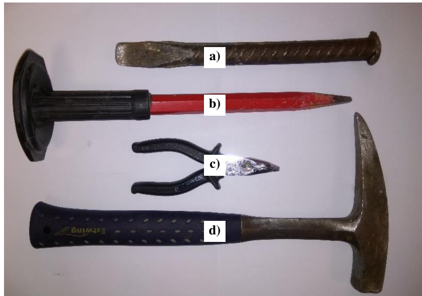
Figure 3.6. Sampling equipment; a) flat chisel b) pointed chisel c) bent nose pliers d) hammer
