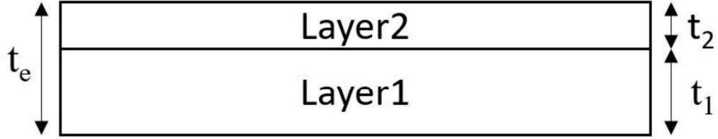
Figure 1.5. Bonded composite structure
