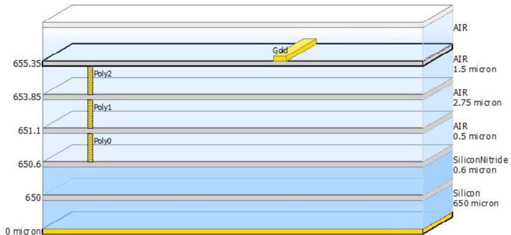
Figure 3.7. Constructed stack in ADS
