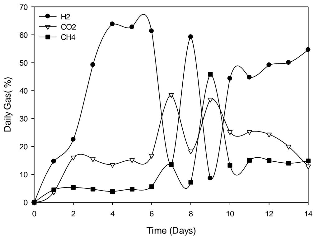
Figure I.1 Daily headspace gas composition change for 2% TP-test reactor
