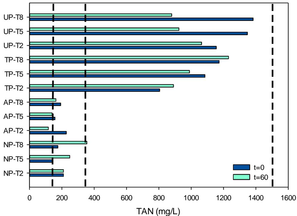
Figure 4.4 Initial and final TAN Concentrations of OSAD Test Reactors
