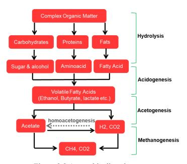
Figure 2.2 Anaerobic digestion steps
