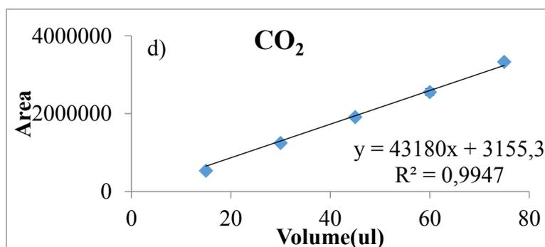
Figure C.1 Calibration Curves of a) H<sub>2</sub>, b) CH<sub>4</sub>, c) N<sub>2</sub>, d) CO<sub>2</sub>
