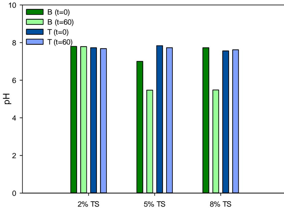
Figure 4.5 pH changes in NP-Blank (B) and NP-Test (T) Reactors
