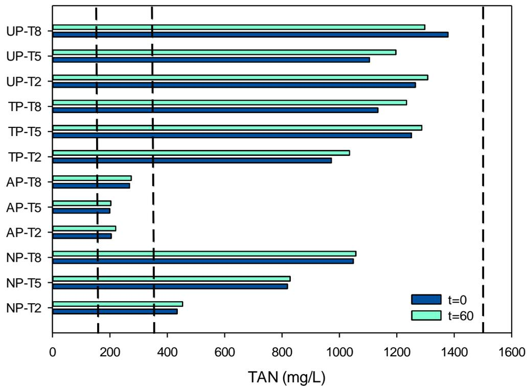
Figure 4.11 Initial and final TAN concentrations in the methanogenesis stage of TSAD test reactors
