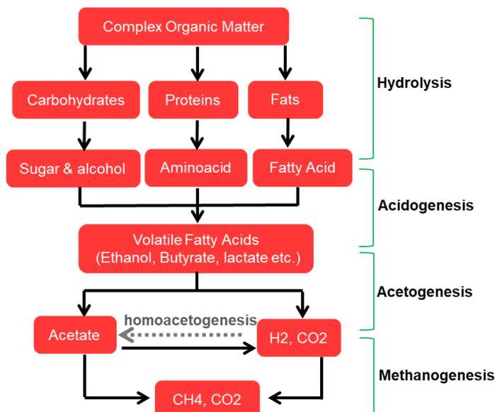
Figure 2.2 Anaerobic digestion steps
