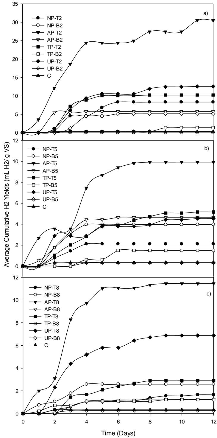
Figure 4.6 Average cumulative H<sub>2</sub> yields for a) 2% TS, b) 5% TS c) 8% TS content for test reactors in DF
