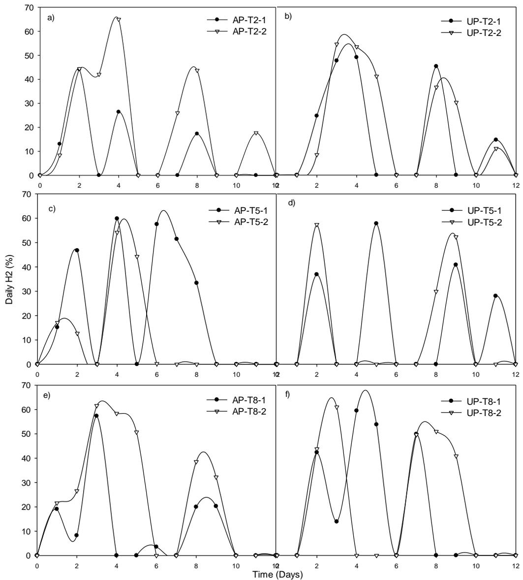
Figure 4.7 Daily H<sub>2</sub>% content in the headspace of 2% TS containing test reactors of AP-yard waste and UP-yard waste a) 2% TS AP, b) 2% TS UP, c) 5%TS AP, d) 5% TS UP, e) 8% TS AP, e) 8% TS UP (1 and 2 in the legends refer to the duplicate reactors)
