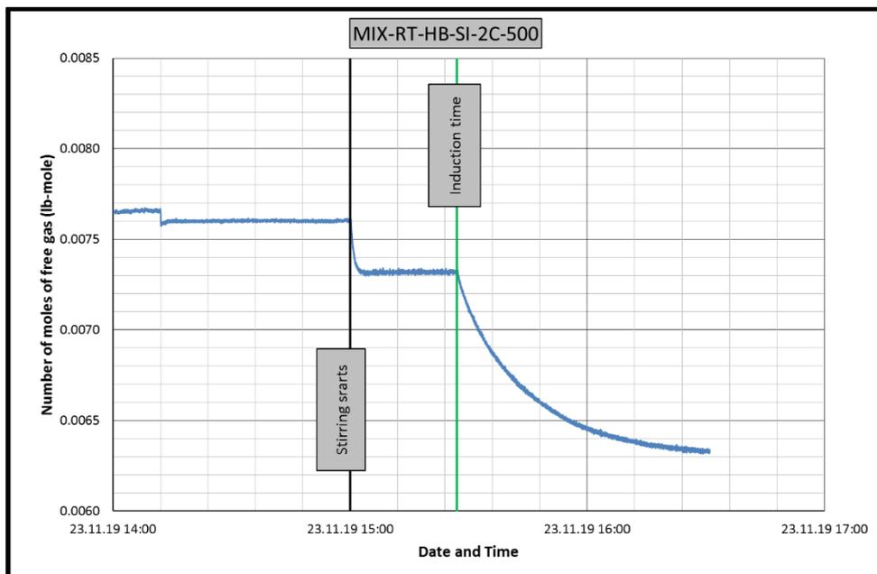
**Figure B.82** Change in number of moles of free gas in CH<sub>4</sub>-C<sub>3</sub>H<sub>8</sub>-RT-HB-SI-2C experiment
