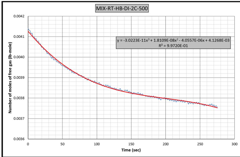
**Figure B.107** Gas consumption rate equation-1 for CH<sub>4</sub>-C<sub>3</sub>H<sub>8</sub>-RT-HB-DI-2C experiment
