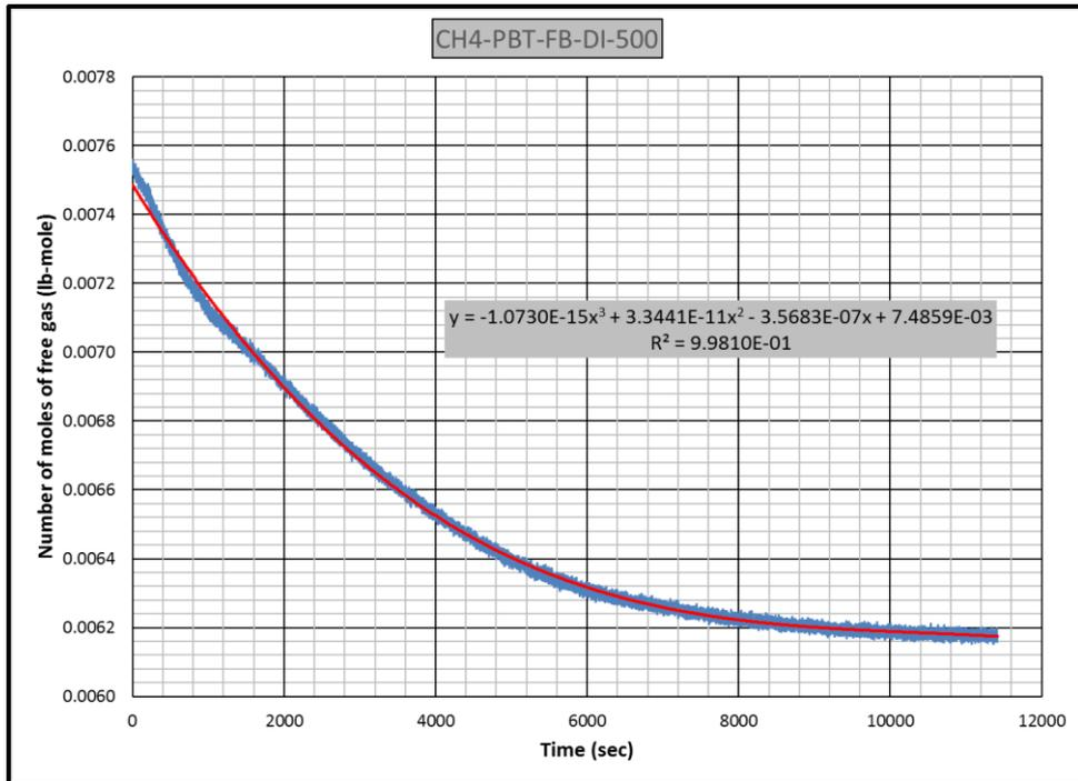
**Figure B.18** Gas consumption rate equation for CH4-PBT-FB-DI experiment
