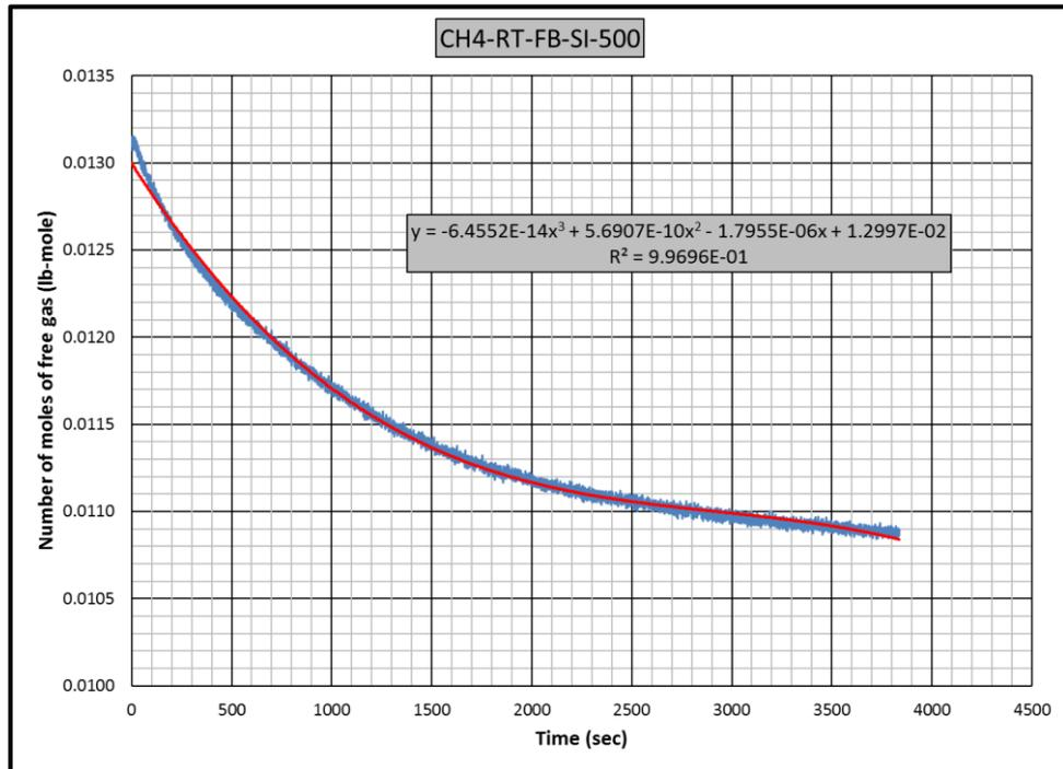
**Figure B.10** Gas consumption rate equation for CH4-RT-FB-SI experiment
