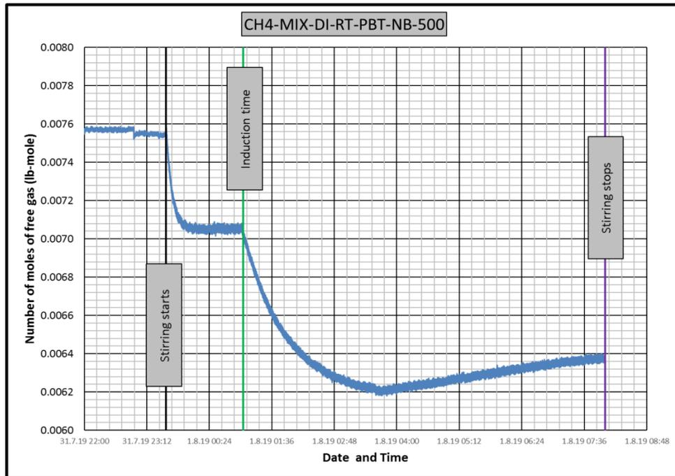
**Figure B.37** Change in number of moles of free gas in CH4-MIX-RT-PBT-NB-DI experiment
