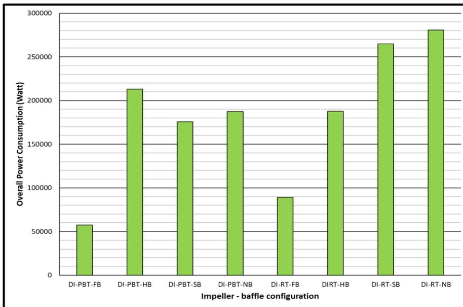
**Figure 6.11** Overall power consumption of dual impeller experiments
