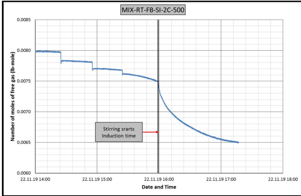
**Figure B.77** Change in number of moles of free gas in CH<sub>4</sub>-C<sub>3</sub>H<sub>8</sub>-RT-FB-SI-2C experiment
