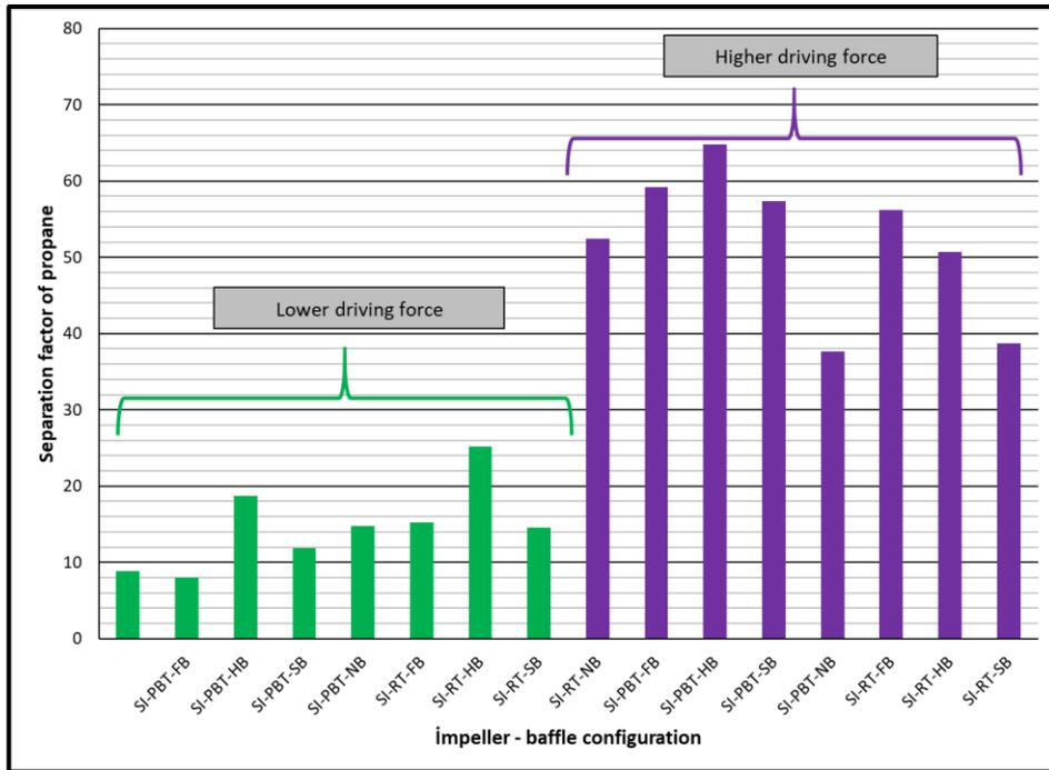
Figure 7.4 Separation factor of propane of single impeller mixture hydrate experiments
