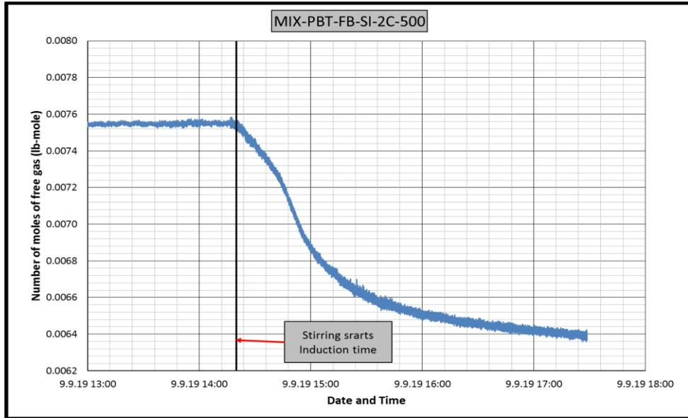
**Figure B.69** Change in number of moles of free gas in CH<sub>4</sub>-C<sub>3</sub>H<sub>8</sub>-PBT-FB-SI-2C experiment
