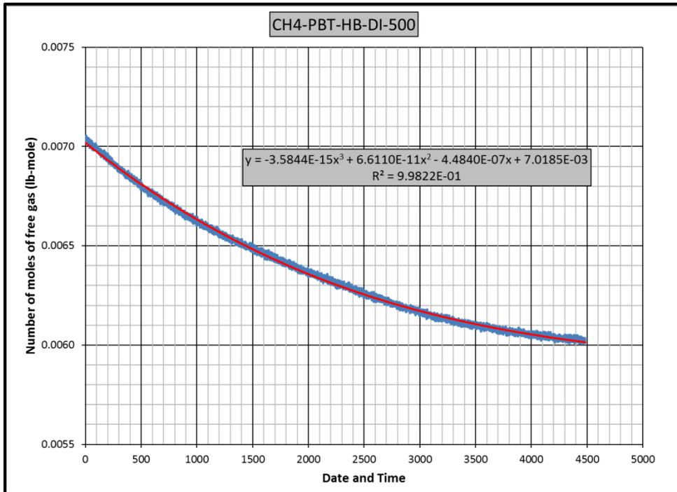
Figure B.20 Gas consumption rate equation for CH4-PBT-HB-DI experiment
