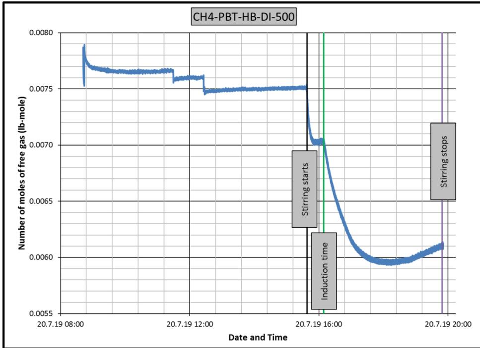
Figure B.19 Change in number of moles of free gas in CH4-PBT-HB-DI experiment
