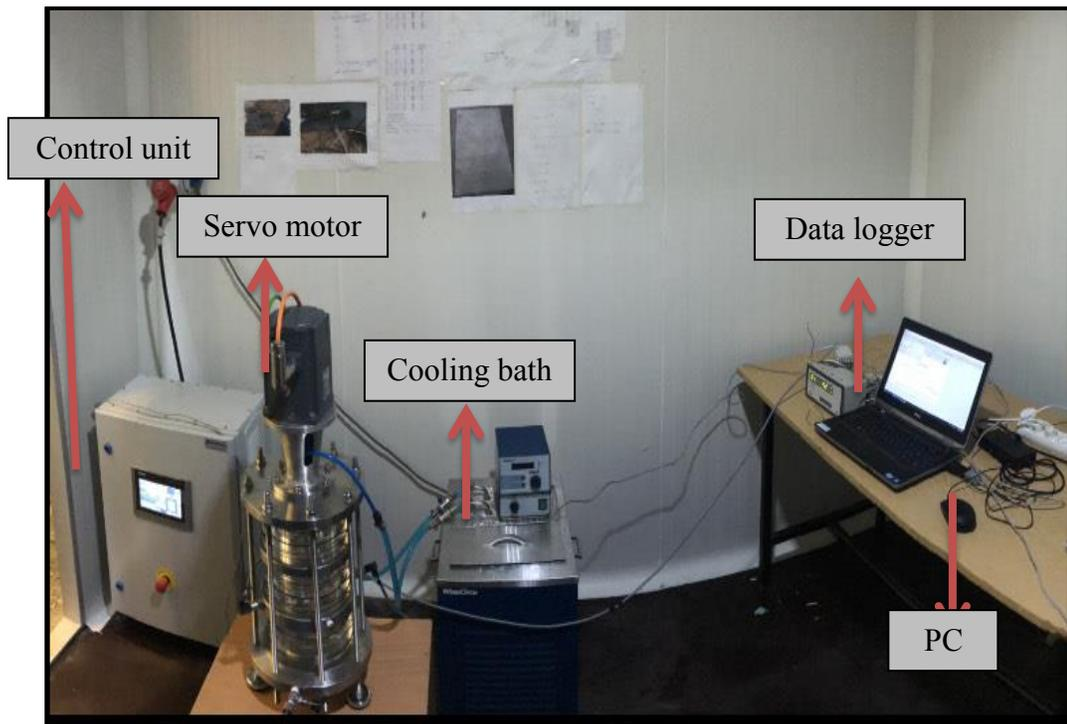
**Figure 5.9** Experimental setup of transparent reactor
