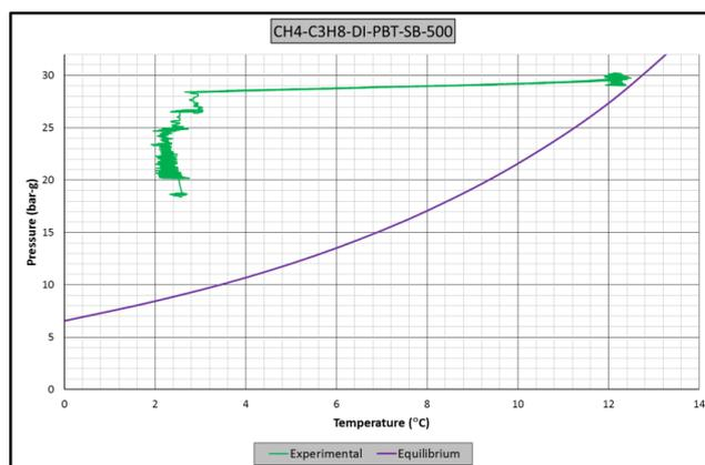
**Figure A.43** Raw data of experiment CH4-C3H8-PBT-SB-DI-500. A: Pressure – temperature vs. time graph, B: Pressure – torque vs. time graph, C: Pressure vs. temperature graph. (Driving force=16)
