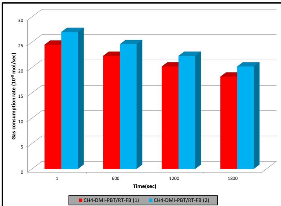
**Figure 6.18** Repeatability test of CH4-DMI-RT/PBT-FB in terms of gas consumption rate
