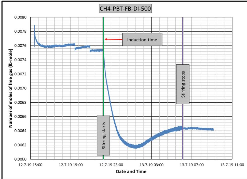
**Figure B.17** Change in number of moles of free gas in CH4-PBT-FB-DI experiment
