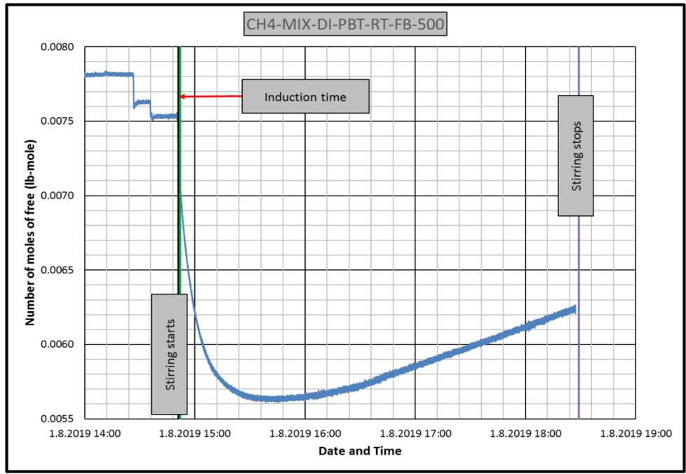
**Figure B.41** Change in number of moles of free gas in CH4-MIX-PBT-RT-FB-DI experiment
