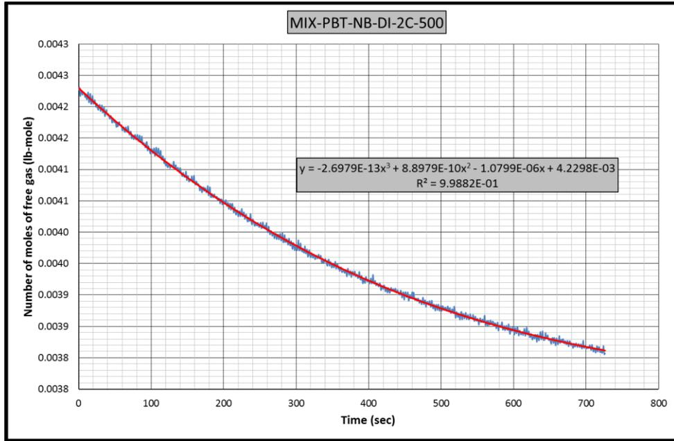
**Figure B.101** Gas consumption rate equation-1 for CH<sub>4</sub>-C<sub>3</sub>H<sub>8</sub>-PBT-NB-DI-2C experiment
