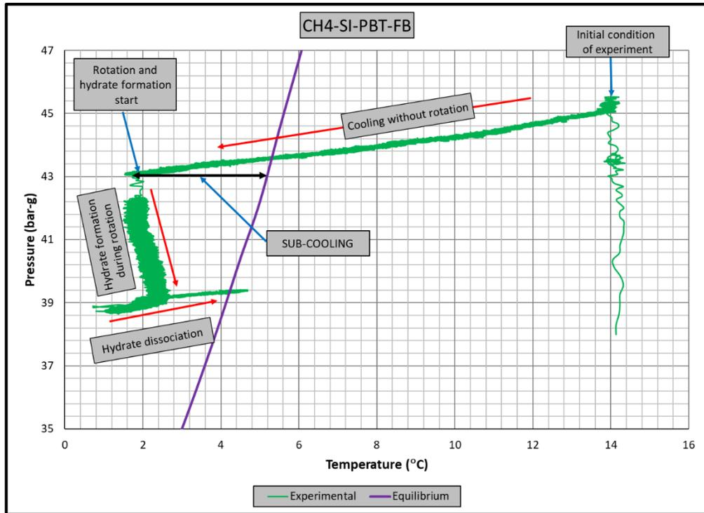
**Figure 6.3** Pressure vs. temperature graph of hydrate formation experiment
