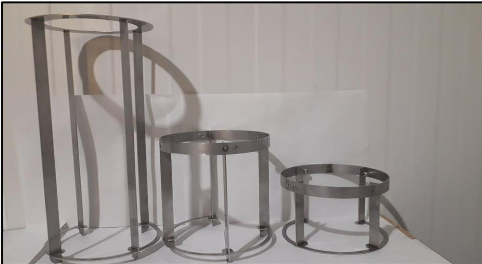
**Figure 5.6** Types of baffles used in this study, Left: FB, Middle: HB, Right: SB
