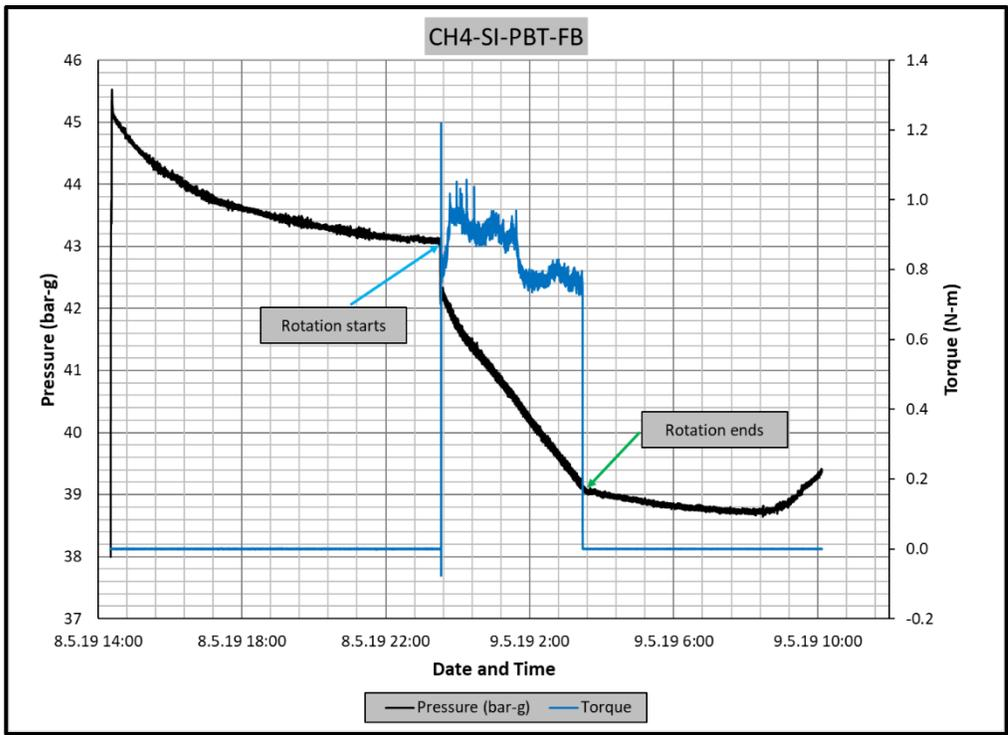
Figure 6.2 Pressure vs. torque graph of hydrate formation experiment
