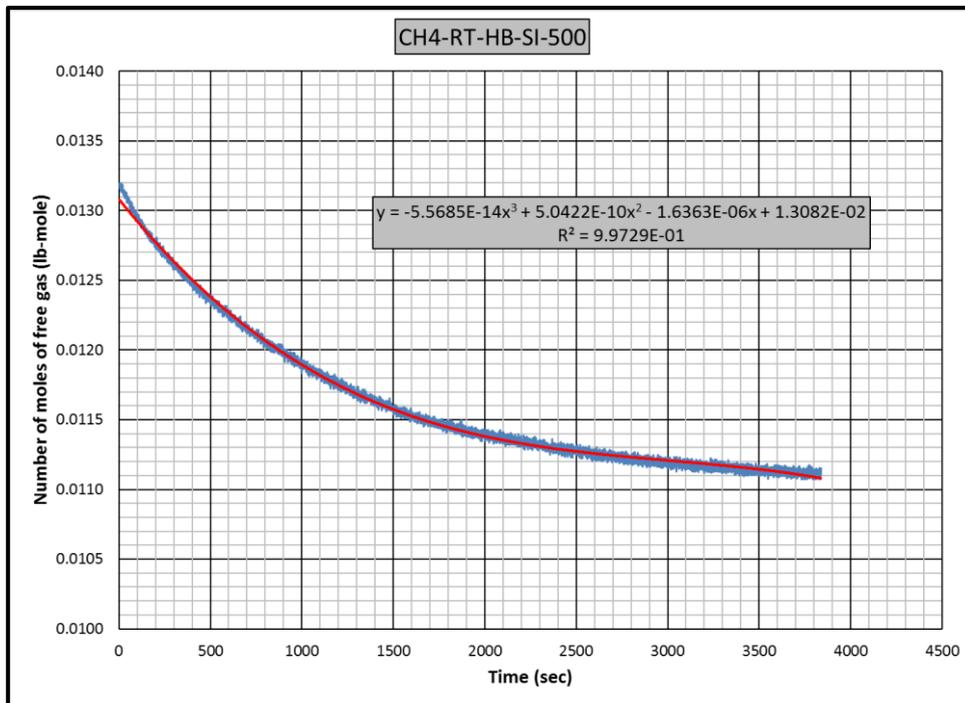
Figure B.12 Gas consumption rate equation for CH4-RT-HB-SI experiment
