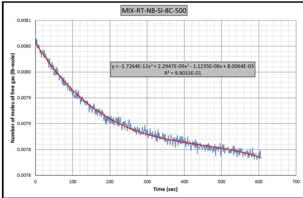
**Figure B.67** Gas consumption rate equation-1 for CH<sub>4</sub>-C<sub>3</sub>H<sub>8</sub>-RT-NB-SI-8C experiment
