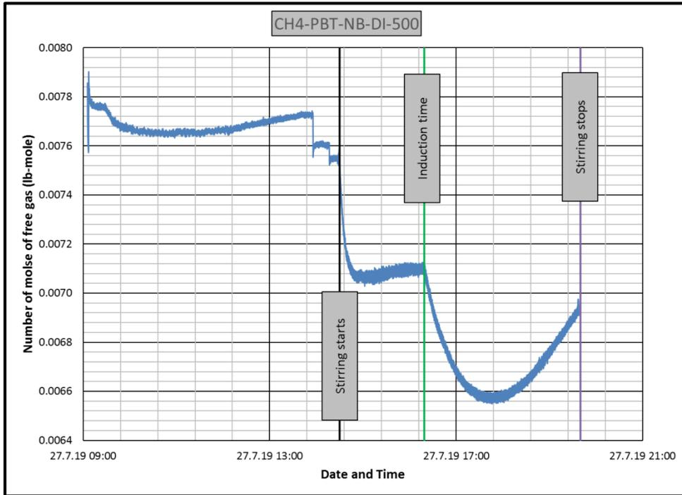
**Figure B.23** Change in number of moles of free gas in CH4-PBT-NB-DI experiment
