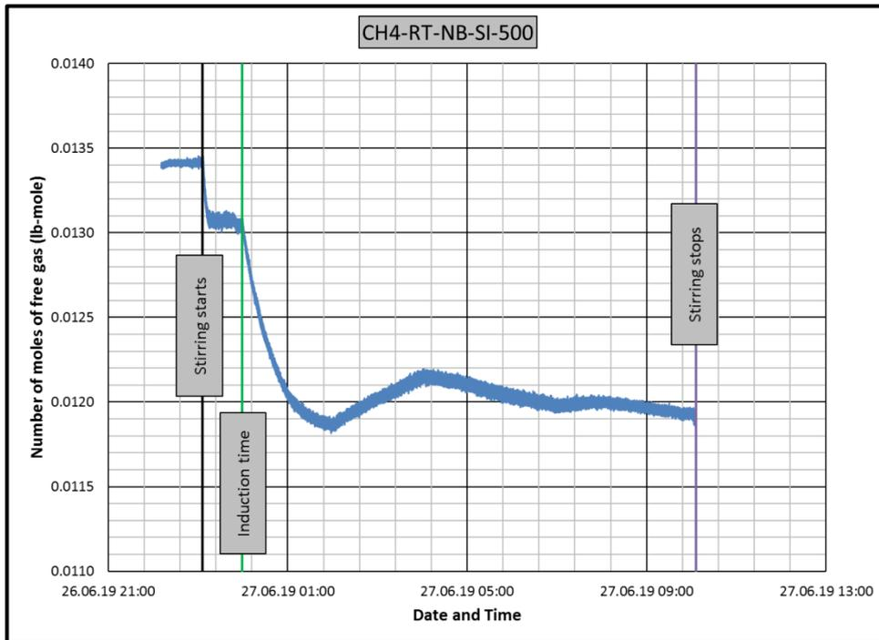
**Figure B.15** Change in number of moles of free gas in CH4-RT-NB-SI experiment
