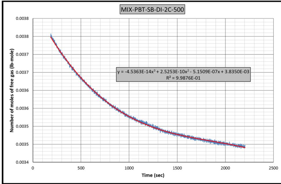
Figure B.99 Gas consumption rate equation-2 for CH<sub>4</sub>-C<sub>3</sub>H<sub>8</sub>-PBT-SB-DI-2C experiment
