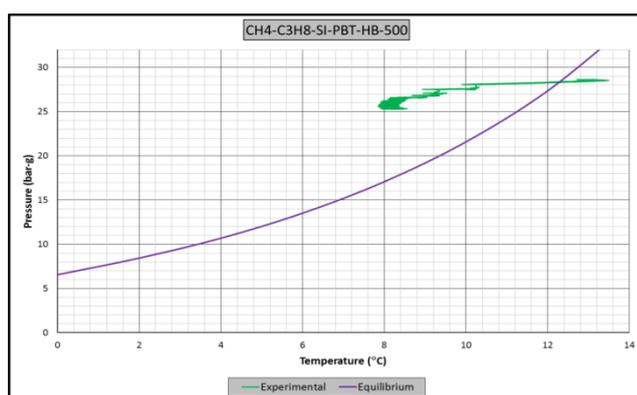
**Figure A.26** Raw data of experiment CH4-C3H8-PBT-HB-SI-500. A: Pressure – temperature vs. time graph, B: Pressure – torque vs. time graph, C: Pressure vs. temperature graph. (Driving force=8.5)
