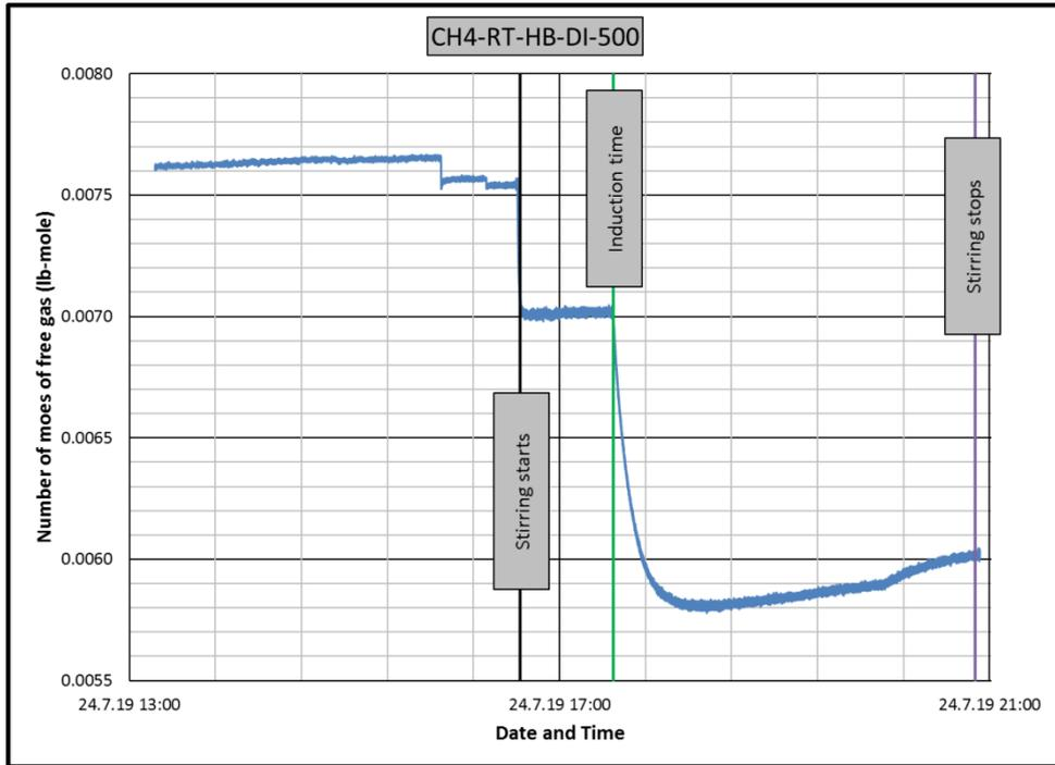
**Figure B.27** Change in number of moles of free gas in CH4-RT-HB-DI experiment
