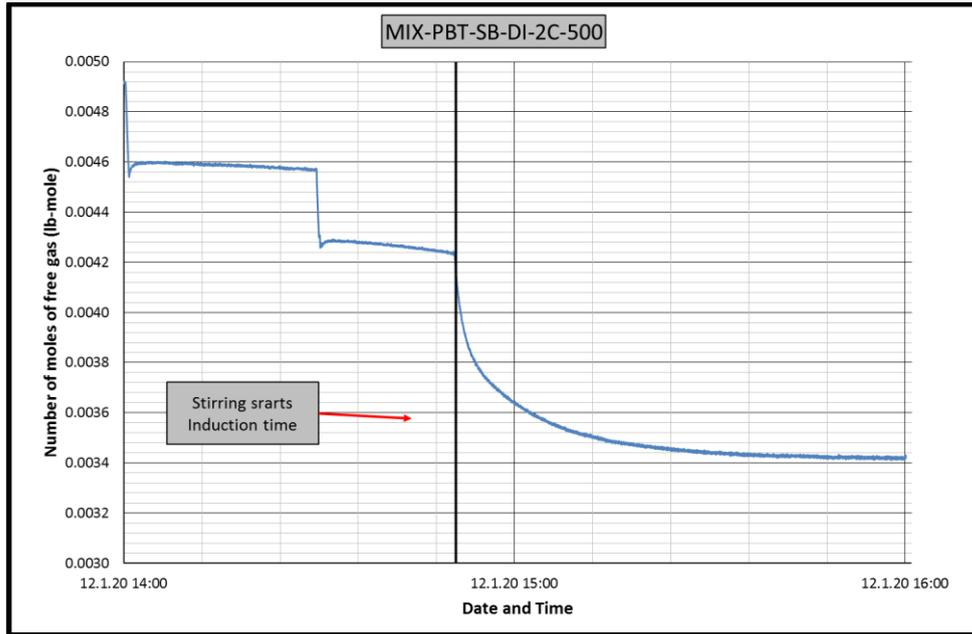
**Figure B.97** Change in number of moles of free gas in CH<sub>4</sub>-C<sub>3</sub>H<sub>8</sub>-PBT-SB-DI-2C experiment
