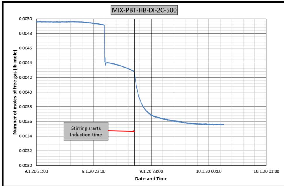
Figure B.94 Change in number of moles of free gas in CH<sub>4</sub>-C<sub>3</sub>H<sub>8</sub>-PBT-HB-DI-2C experiment
