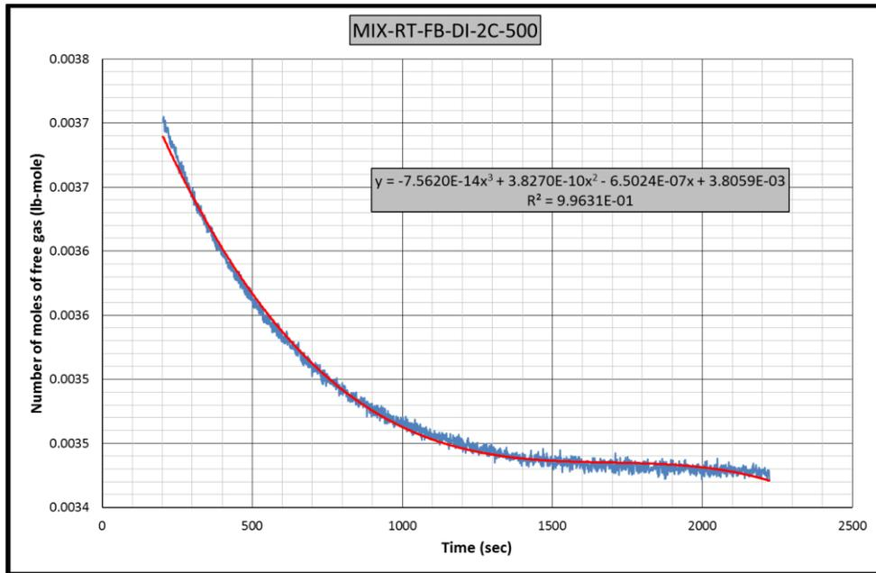
Figure B.105 Gas consumption rate equation-2 for CH<sub>4</sub>-C<sub>3</sub>H<sub>8</sub>-RT-FB-DI-2C experiment
