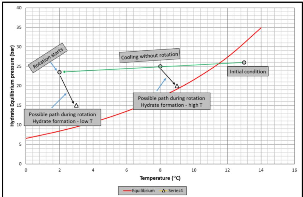
**Figure 5.13** Experimental conditions of gas mixture experiments
