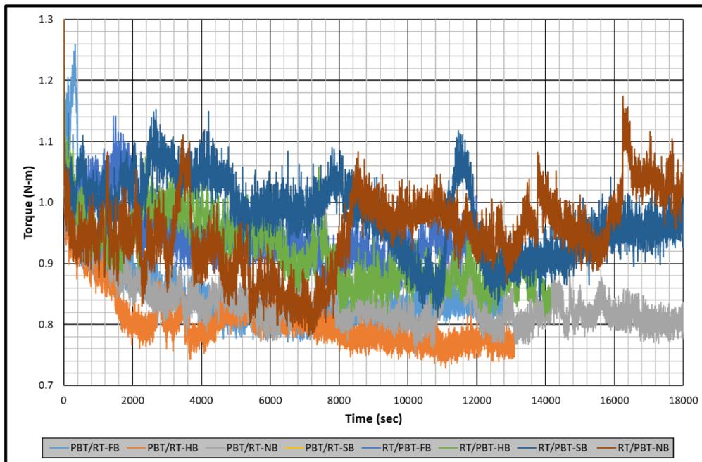
**Figure 6.15** Recorded torque values of dual-mixed impeller experiments
