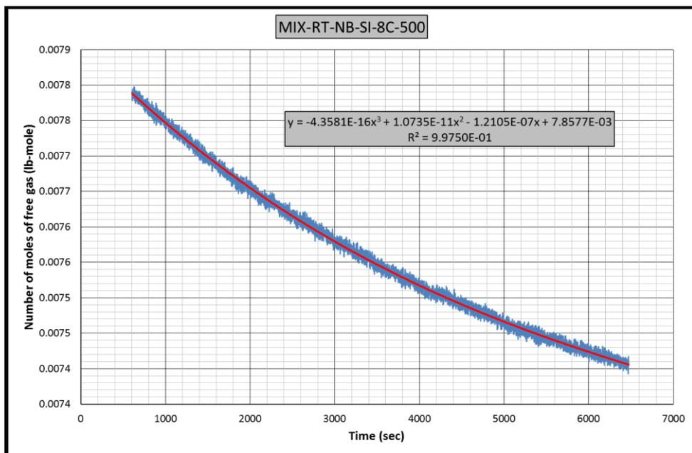
**Figure B.68** Gas consumption rate equation-2 for CH<sub>4</sub>-C<sub>3</sub>H<sub>8</sub>-RT-NB-SI-8C experiment
