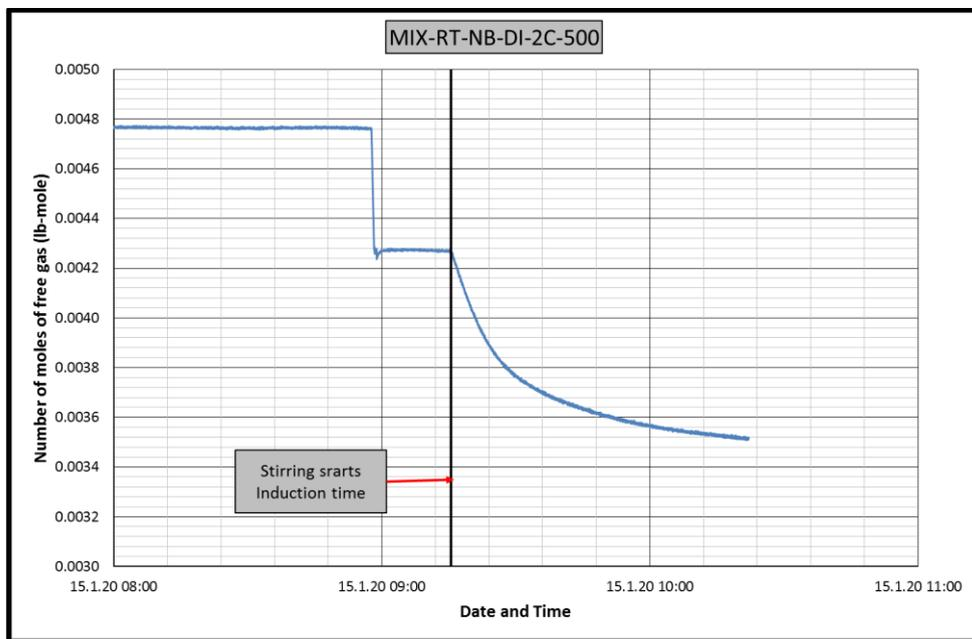
**Figure B.112** Change in number of moles of free gas in CH<sub>4</sub>-C<sub>3</sub>H<sub>8</sub>-RT-NB-DI-2C experiment
