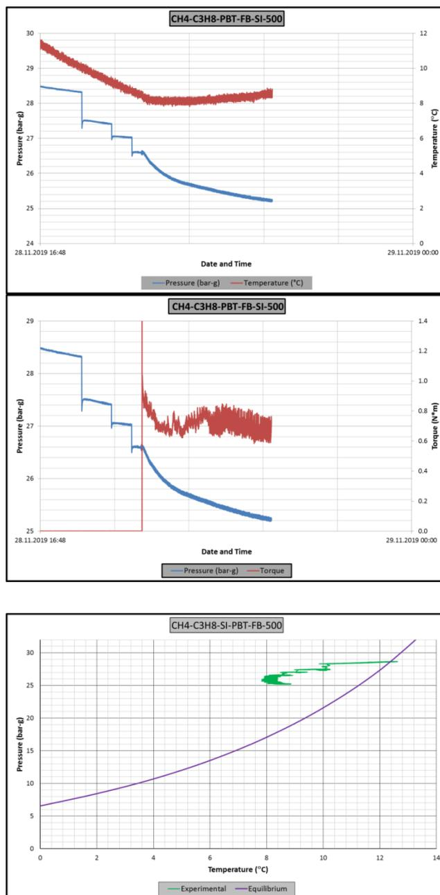
**Figure A.25** Raw data of experiment CH4-C3H8-PBT-FB-SI-500. A: Pressure – temperature vs. time graph, B: Pressure – torque vs. time graph, C: Pressure vs. temperature graph. (Driving force=8.5)
