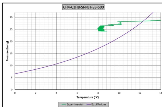
**Figure A.27** Raw data of experiment CH4-C3H8-PBT-SB-SI-500. A: Pressure – temperature vs. time graph, B: Pressure – torque vs. time graph, C: Pressure vs. temperature graph. (Driving force=8.5)
