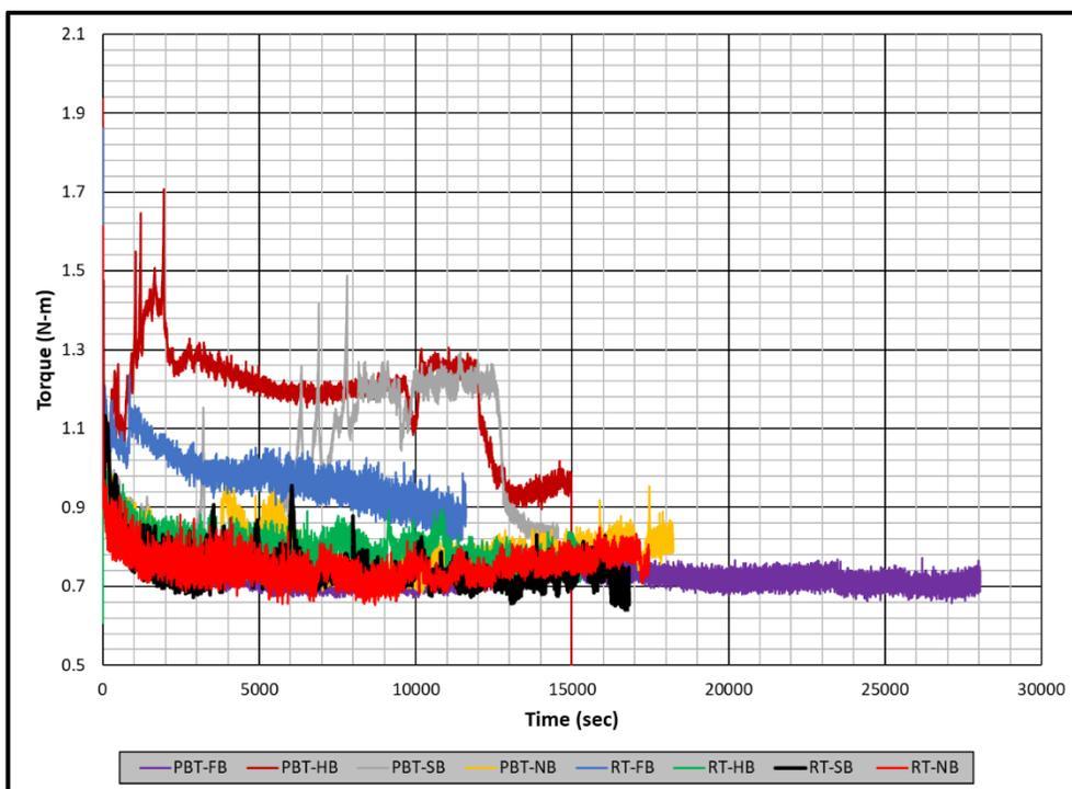
Figure 6.12 Recorded torque values of single impeller experiments
