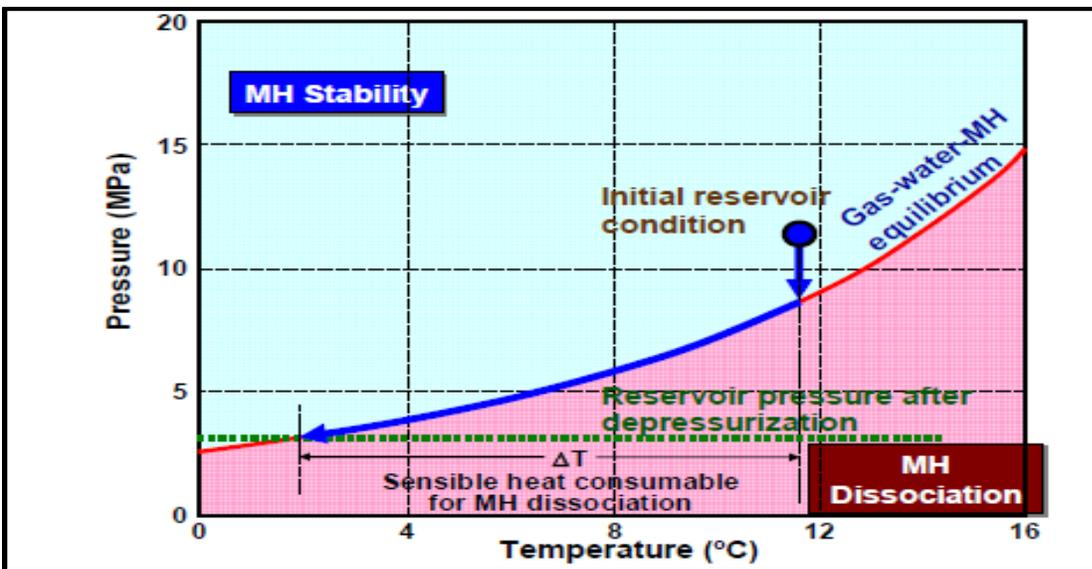
**Figure 2.1** Temperature reductions along with the MH dissociation in depressurization method [27].
