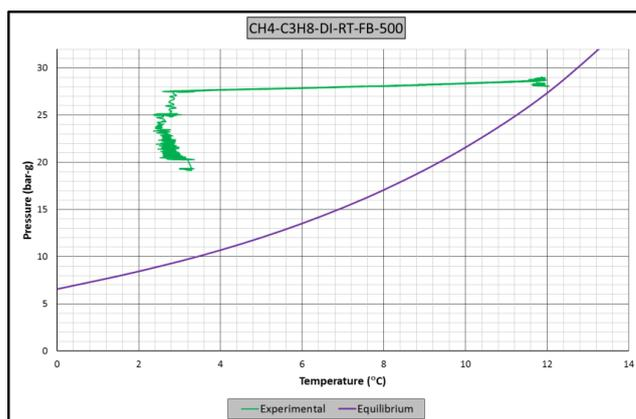
**Figure A.45** Raw data of experiment CH4-C3H8-RT-FB-DI-500. A: Pressure – temperature vs. time graph, B: Pressure – torque vs. time graph, C: Pressure vs. temperature graph. (Driving force=16)
