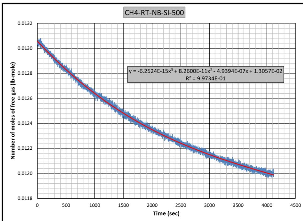
**Figure B.16** Gas consumption rate equation for CH4-RT-NB-SI experiment
