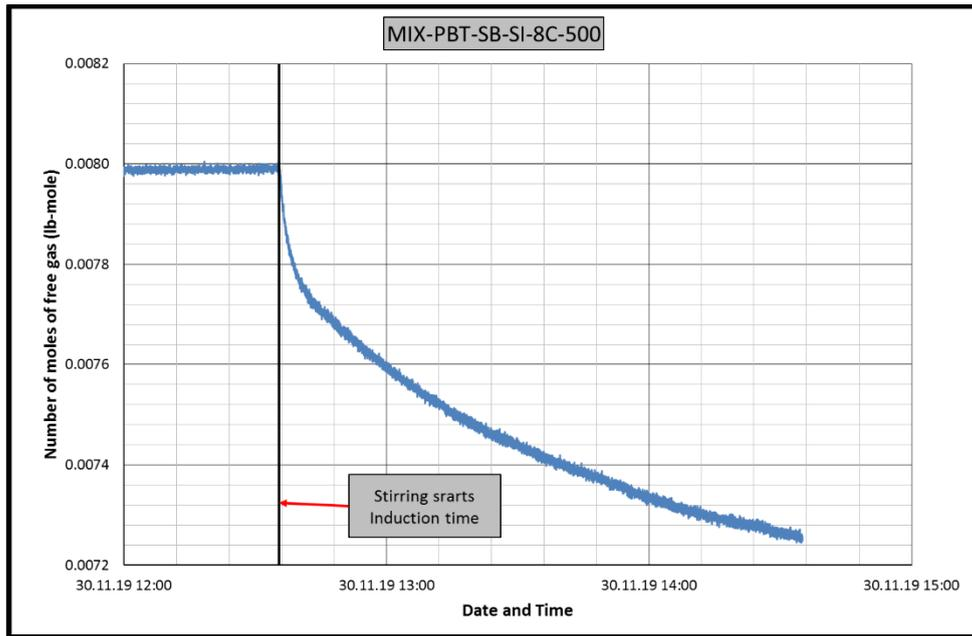
**Figure B.53** Change in number of moles of free gas in CH<sub>4</sub>-C<sub>3</sub>H<sub>8</sub>-PBT-SB-SI-8C experiment
