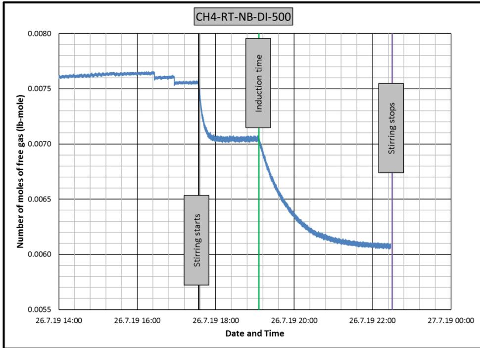
Figure B.31 Change in number of moles of free gas in CH4-RT-NB-DI experiment
