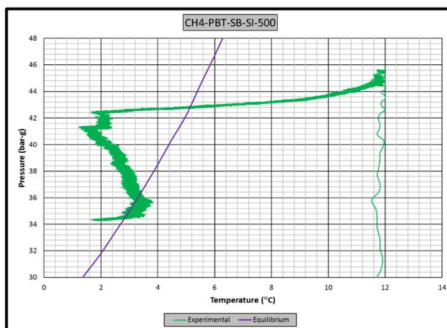
**Figure A.3** Raw data of experiment CH4-PBT-SB-SI-500. A: Pressure – temperature vs. time graph, B: Pressure – torque vs. time graph, C: Pressure vs. temperature graph
