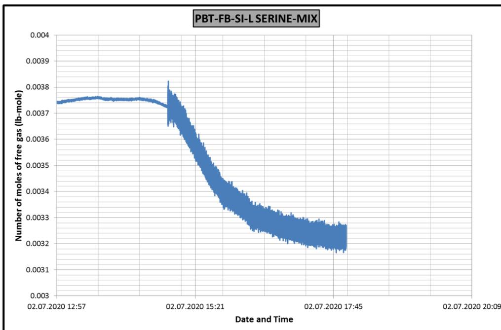
*Figure B.120* Change in number of moles of free gas in PBT-FB-SI-L SERINE-MIX experiment
