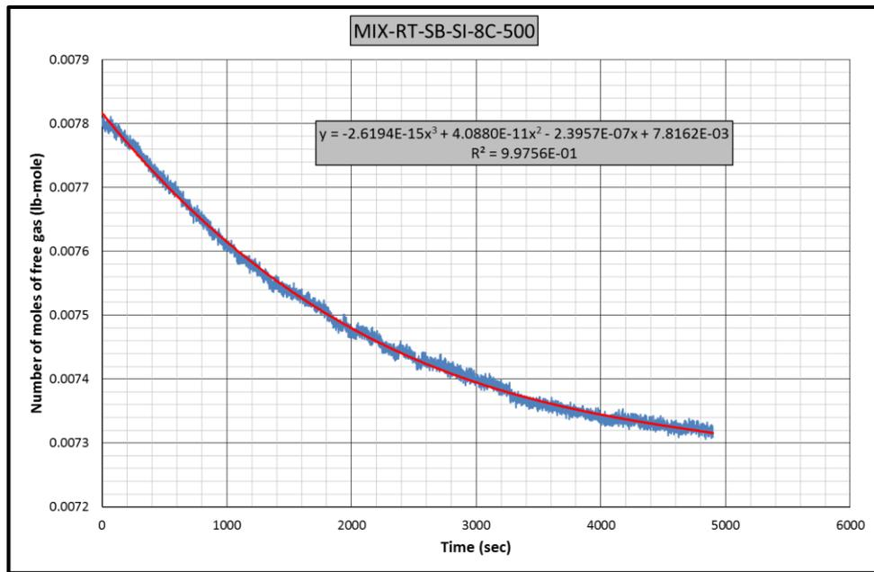
**Figure B.56** Gas consumption rate equation-1 for CH<sub>4</sub>-C<sub>3</sub>H<sub>8</sub>-PBT-NB-SI-8C experiment
