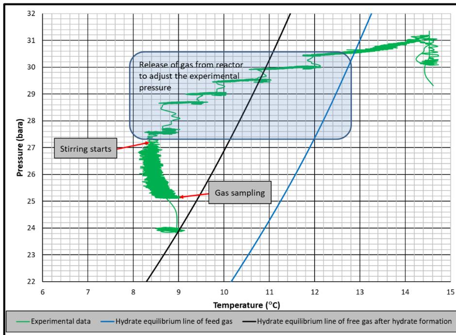
**Figure 7.7** Pressure – temperature diagram of mixture gas of SI-RT-FB (lower driving force)
