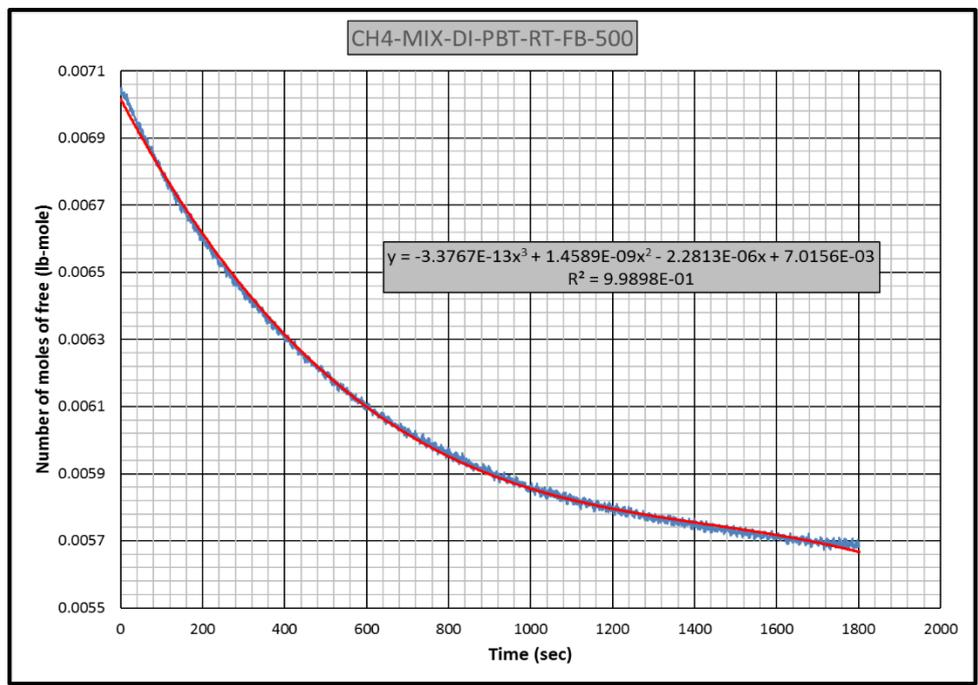
**Figure B.42** Gas consumption rate equation for CH4-MIX-PBT-RT-FB-DI experiment
