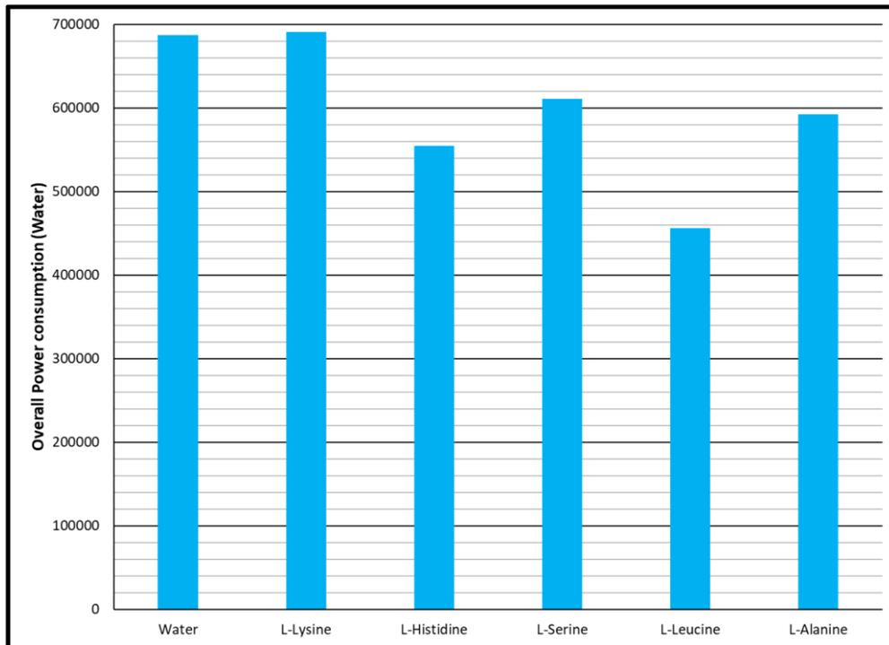
**Figure 8.3** Overall power consumption of water and 5 amino acids during hydrate formation process
