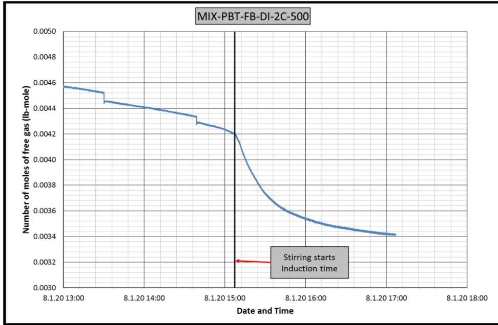
Figure B.91 Change in number of moles of free gas in CH<sub>4</sub>-C<sub>3</sub>H<sub>8</sub>-PBT-FB-DI-2C experiment
