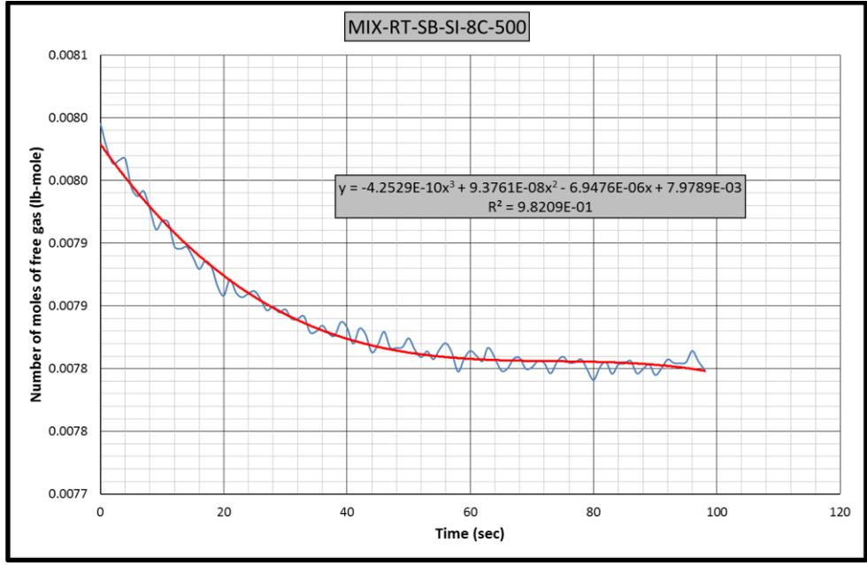
Figure B.64 Gas consumption rate equation-1 for CH<sub>4</sub>-C<sub>3</sub>H<sub>8</sub>-RT-SB-SI-8C experiment
