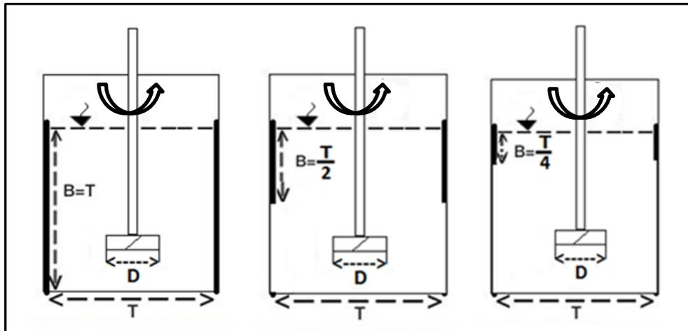
**Figure 5.7** Placement of baffles. Left: FB, Middle: HB and Right: SB
