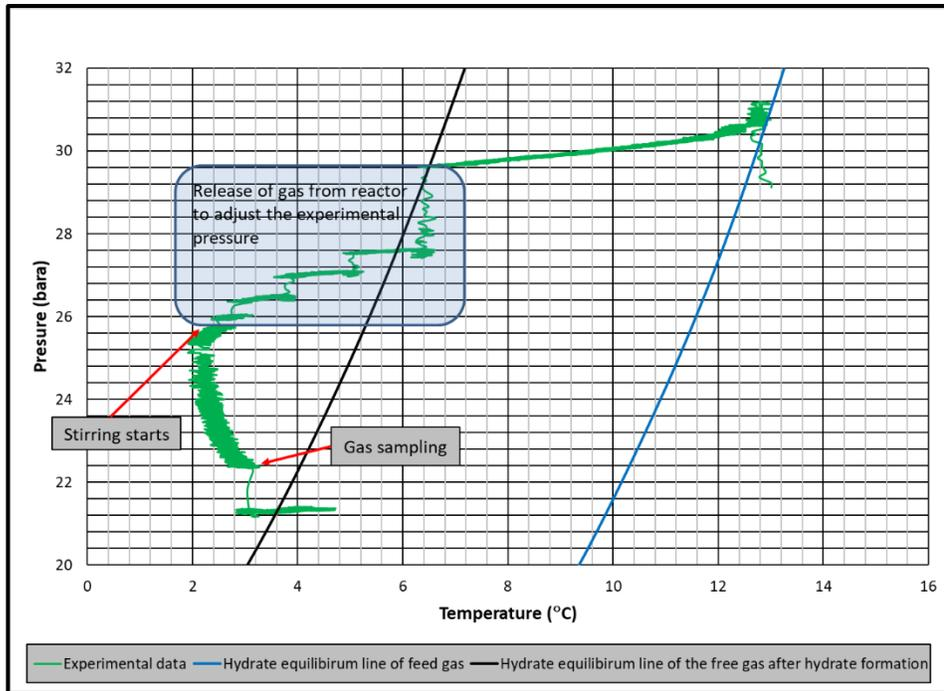
**Figure 7.8** Pressure – temperature diagram of mixture gas of SI-RT-FB (higher driving force)
