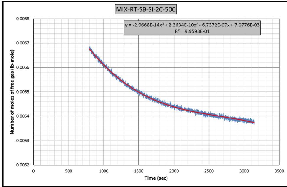
**Figure B.87** Gas consumption rate equation-2 for CH<sub>4</sub>-C<sub>3</sub>H<sub>8</sub>-RT-SB-SI-2C experiment
