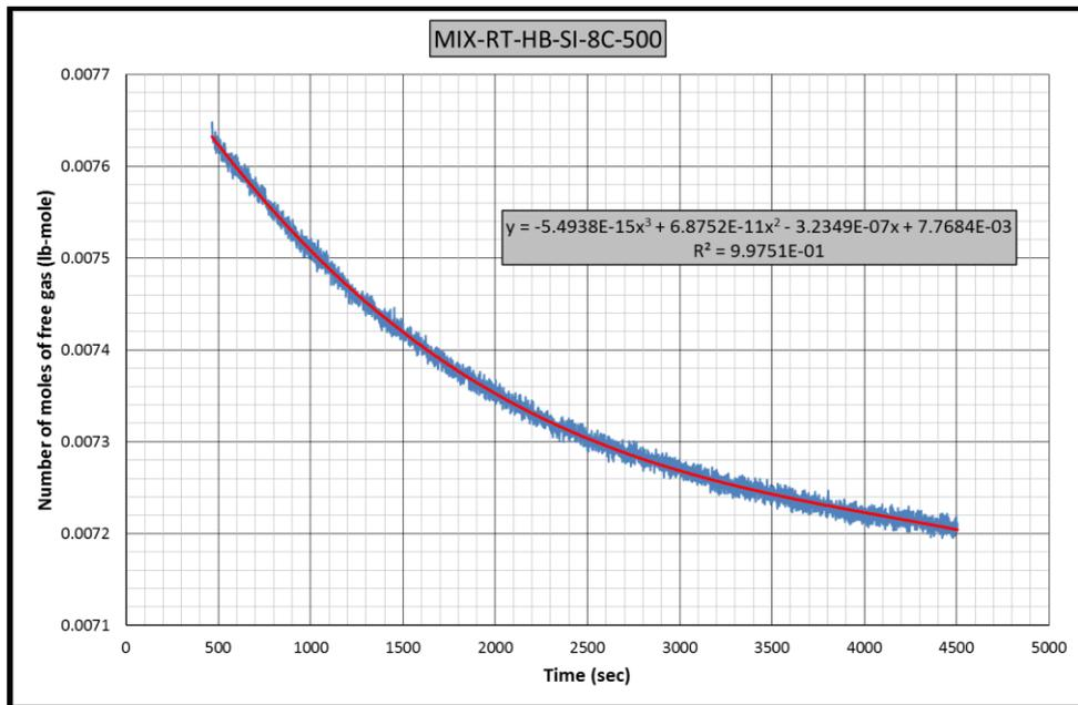
**Figure B.62** Gas consumption rate equation-2 for CH<sub>4</sub>-C<sub>3</sub>H<sub>8</sub>-RT-HB-SI-8C experiment
