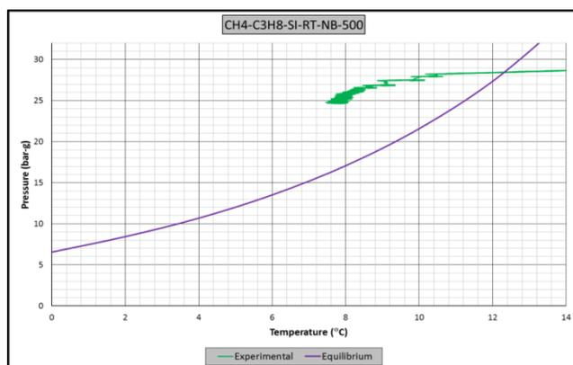
**Figure A.32** Raw data of experiment CH4-C3H8-RT-NB-SI-500. A: Pressure – temperature vs. time graph, B: Pressure – torque vs. time graph, C: Pressure vs. temperature graph. (Driving force=8.5)
