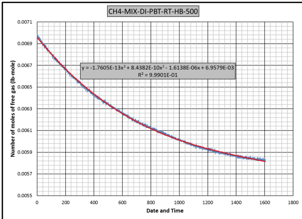
Figure B.44 Gas consumption rate equation for CH4-MIX-PBT-RT-HB-DI experiment
