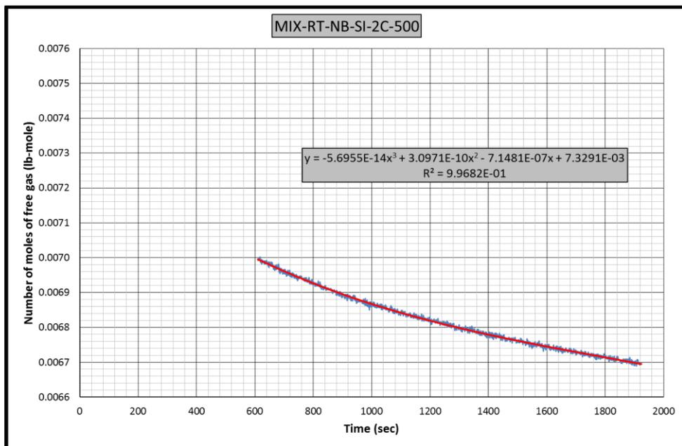
**Figure B.90** Gas consumption rate equation-2 for CH<sub>4</sub>-C<sub>3</sub>H<sub>8</sub>-RT-NB-SI-2C experiment
