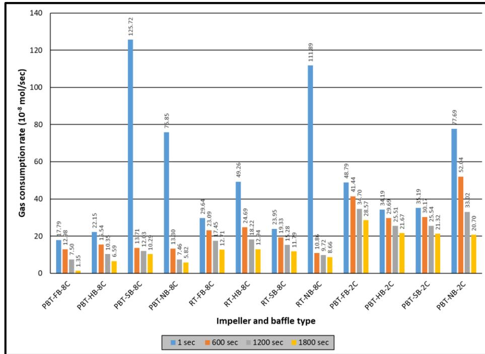
**Figure 7.9** Rate of hydrate formation of mixture gas with single impeller and lower driving force (experimental temperature 8.5 °C)
