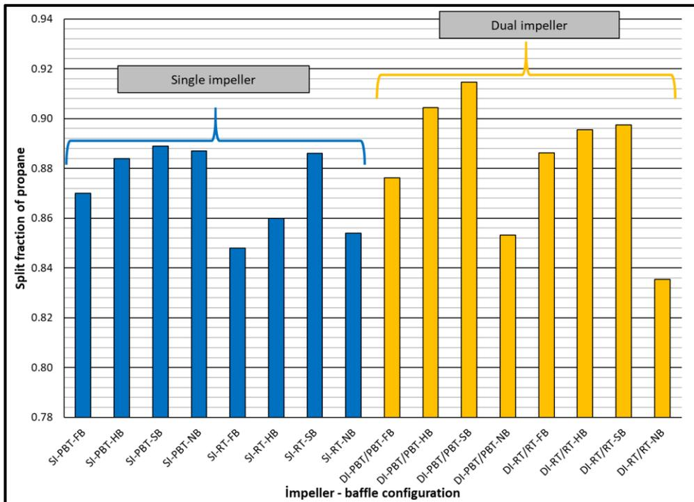
**Figure 7.12** Split fraction of propane for single and dual impeller experiments (experimental temperature 2 °C)
