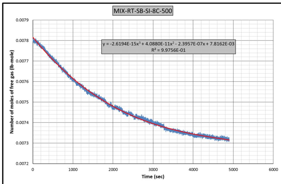
**Figure B.54** Gas consumption rate equation for CH<sub>4</sub>-C<sub>3</sub>H<sub>8</sub>-PBT-SB-SI-8C experiment
