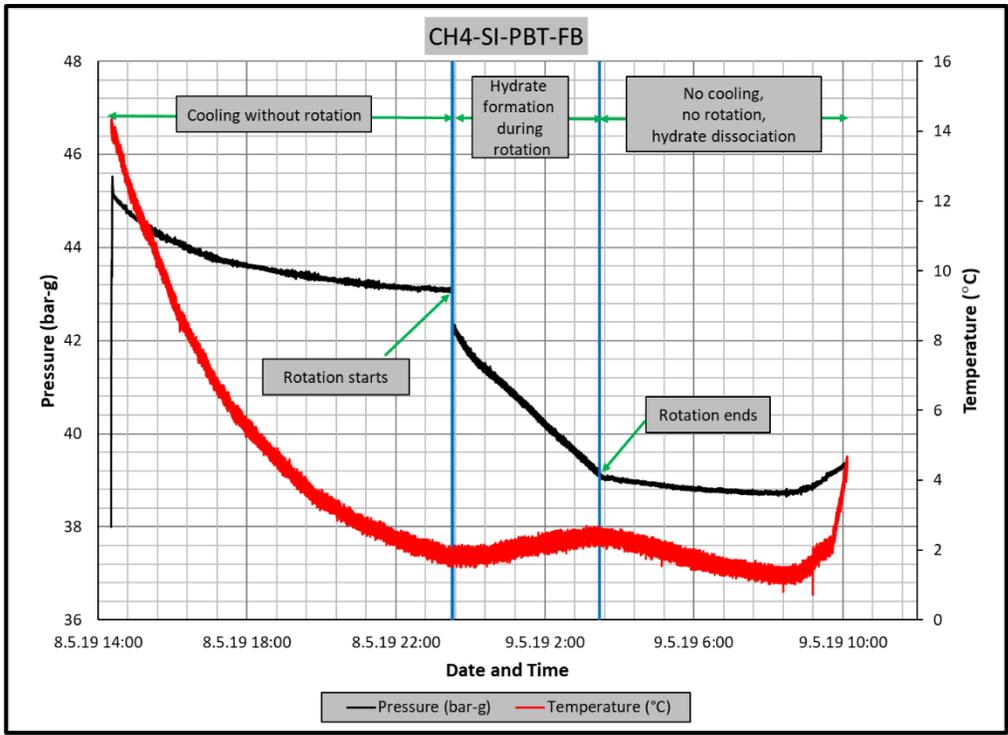
Figure 6.1 Pressure – temperature vs. time graph of hydrate formation experiment
