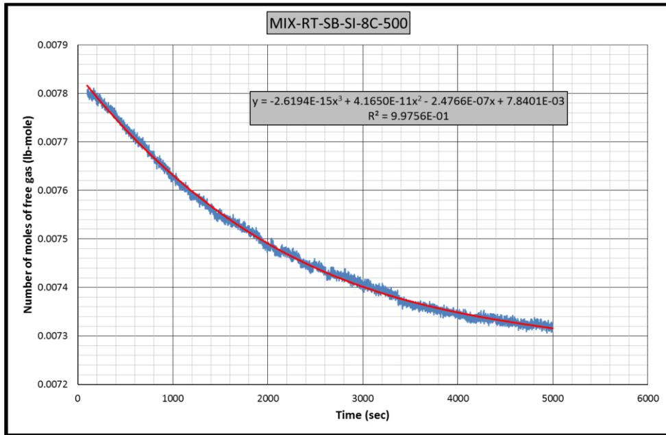
**Figure B.65** Gas consumption rate equation-2 for CH<sub>4</sub>-C<sub>3</sub>H<sub>8</sub>-RT-SB-SI-8C experiment
