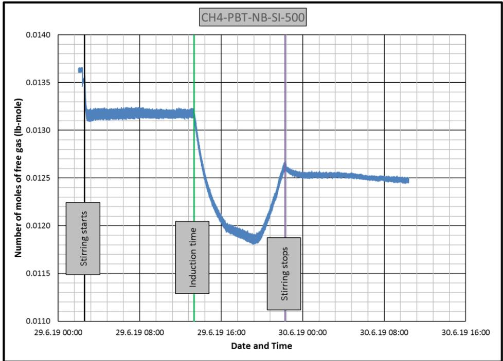
**Figure B.7** Change in number of moles of free gas in CH4-PBT-NB-SI experiment
