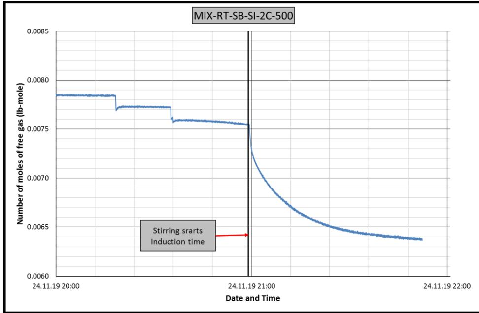
Figure B.85 Change in number of moles of free gas in CH<sub>4</sub>-C<sub>3</sub>H<sub>8</sub>-RT-SB-SI-2C experiment
