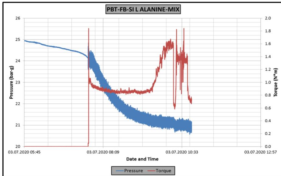
**Figure A.53** Raw data experiment PBT-FB-SI-L ALANINE-MIX, A: Pressure, temperature vs time graph, B: Pressure, torque vs time graph
