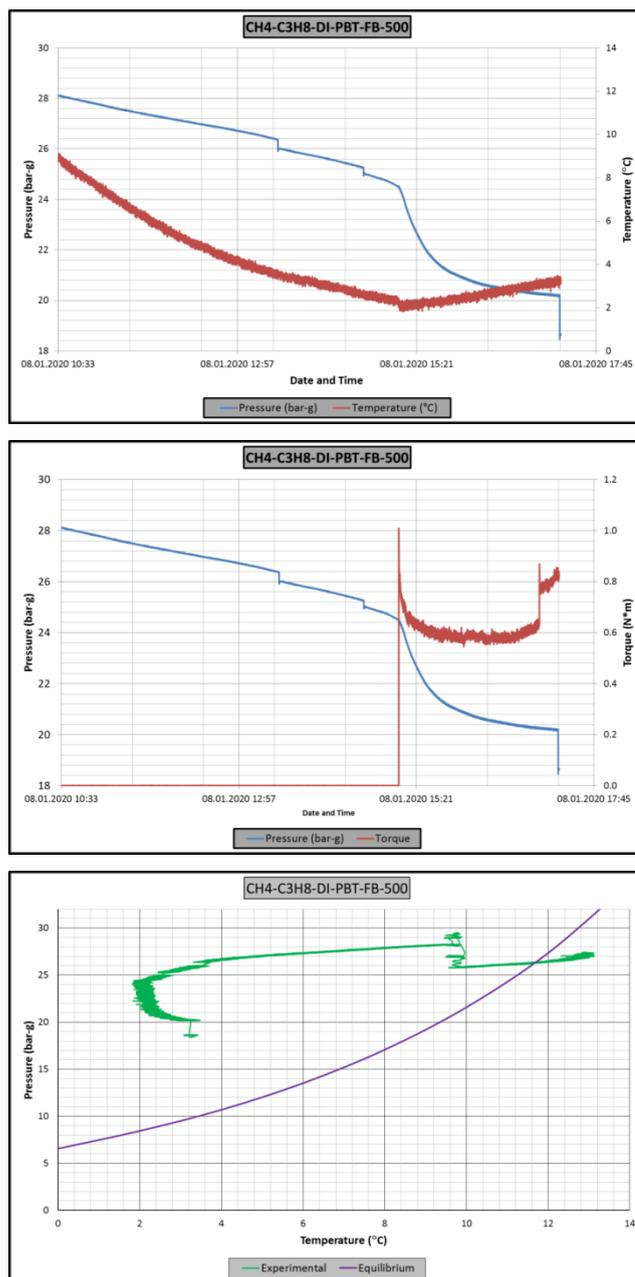
**Figure A.41** Raw data of experiment CH4-C3H8-PBT-FB-DI-500. A: Pressure – temperature vs. time graph, B: Pressure – torque vs. time graph, C: Pressure vs. temperature graph. (Driving force=16)
