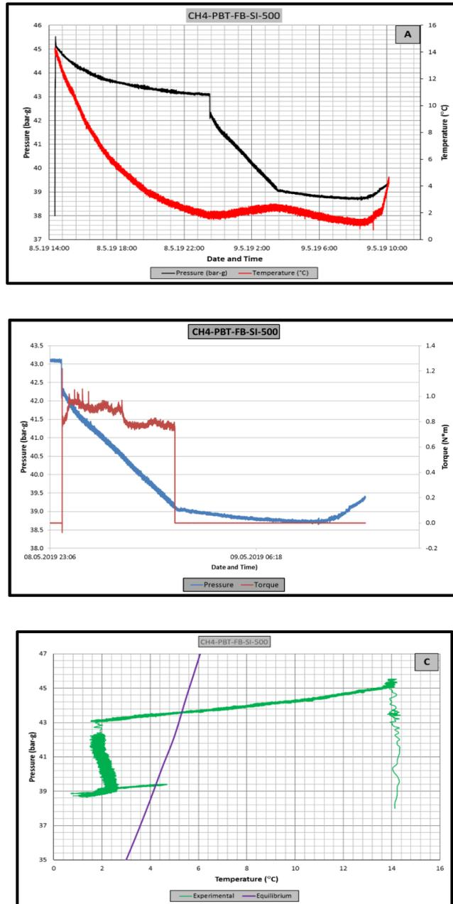
*Figure A.1* Raw data of experiment CH4-PBT-FB-SI-500. A: Pressure – temperature vs. time graph, B: Pressure – torque vs. time graph, C: Pressure vs. temperature graph
