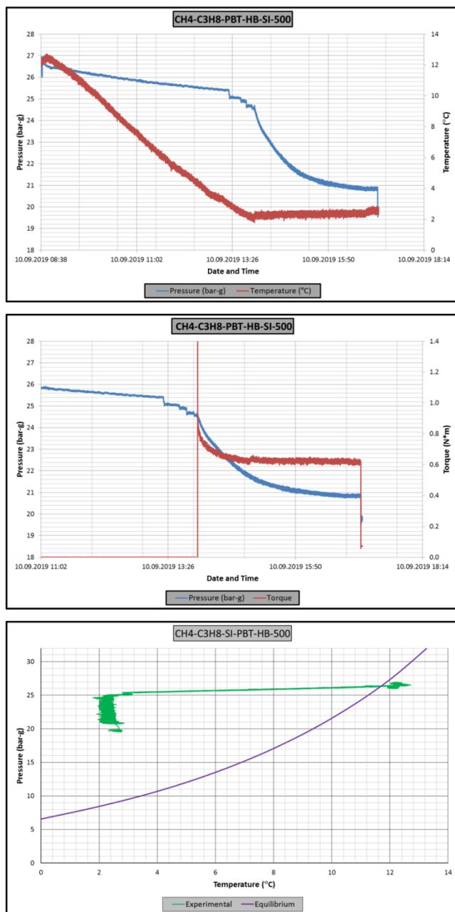
**Figure A.34** Raw data of experiment CH4-C3H8-PBT-HB-SI-500. A: Pressure – temperature vs. time graph, B: Pressure – torque vs. time graph, C: Pressure vs. temperature graph. (Driving force=16)
