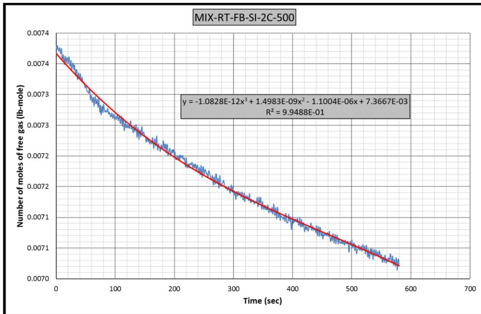
**Figure B.78** Gas consumption rate equation-1 for CH<sub>4</sub>-C<sub>3</sub>H<sub>8</sub>-RT-FB-SI-2C experiment
