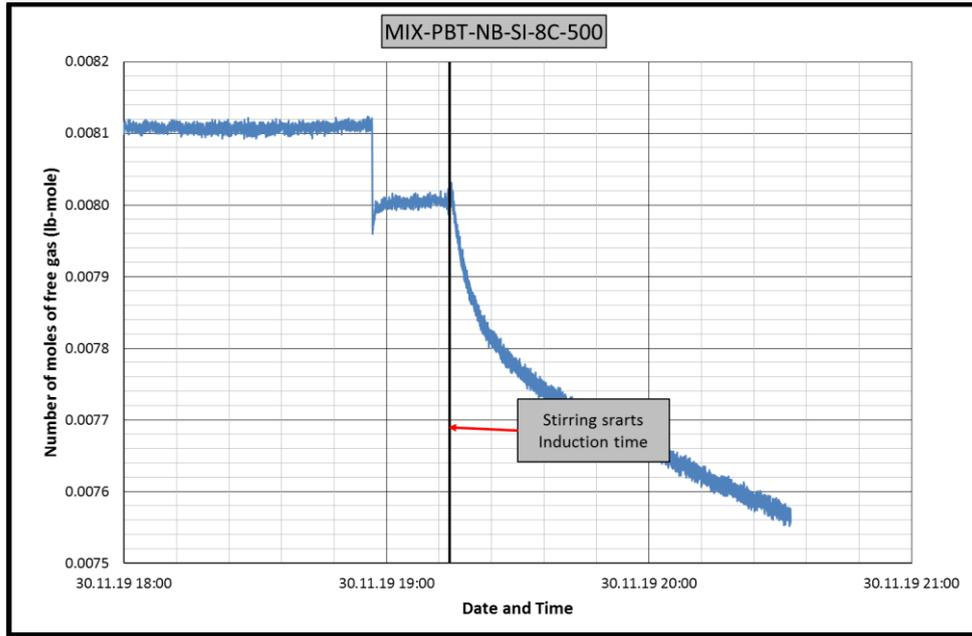
**Figure B.55** Change in number of moles of free gas in CH<sub>4</sub>-C<sub>3</sub>H<sub>8</sub>-PBT-NB-SI-8C experiment
