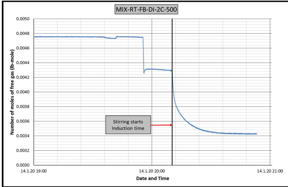
**Figure B.103** Change in number of moles of free gas in CH<sub>4</sub>-C<sub>3</sub>H<sub>8</sub>-RT-FB-DI-2C experiment
