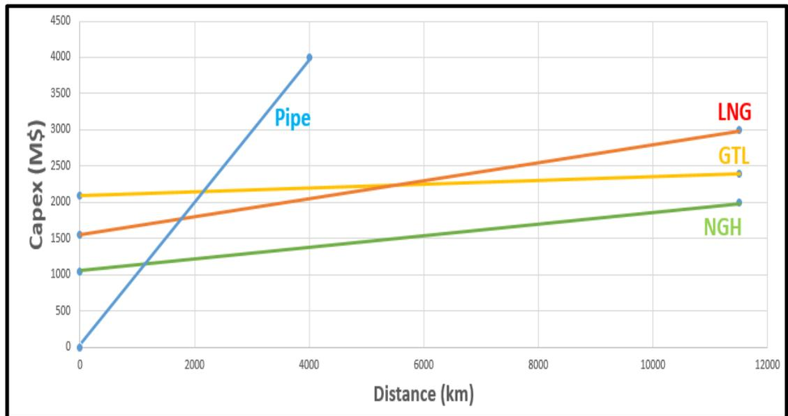
**Figure 2.9** Comparison of gas transportation with different methods [77]
