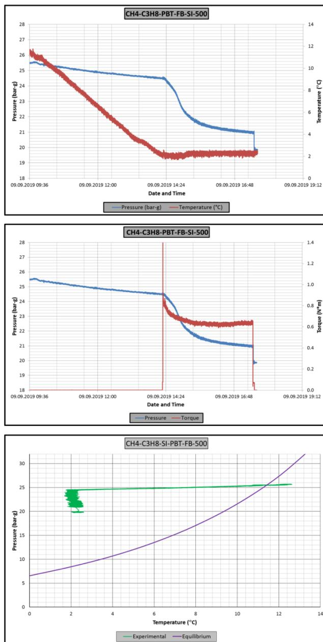
**Figure A.33** Raw data of experiment CH4-C3H8-PBT-FB-SI-500. A: Pressure – temperature vs. time graph, B: Pressure – torque vs. time graph, C: Pressure vs. temperature graph. (Driving force=16)
