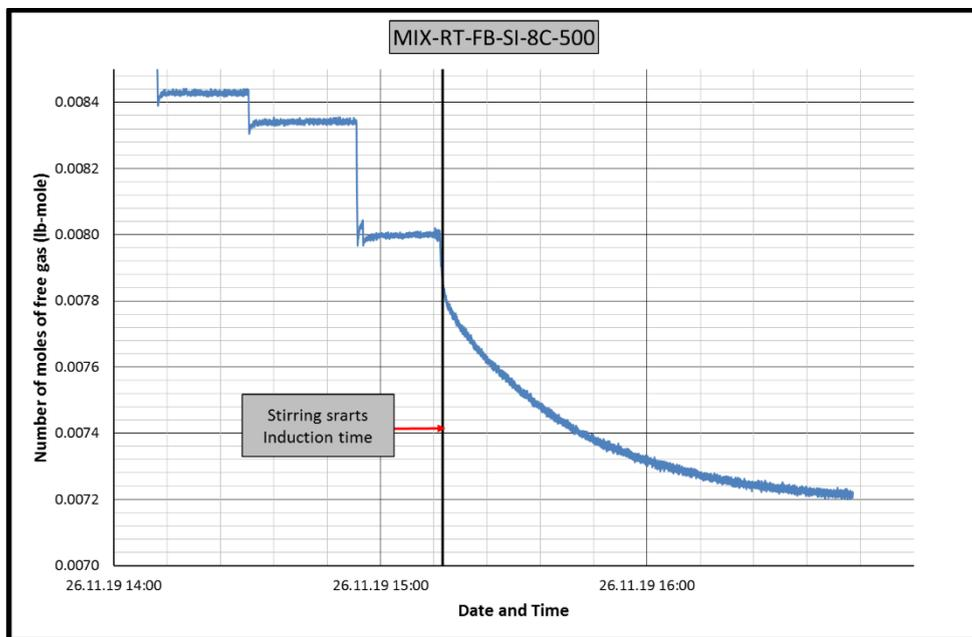
**Figure B.58** Change in number of moles of free gas in CH<sub>4</sub>-C<sub>3</sub>H<sub>8</sub>-RT-FB-SI-8C experiment
