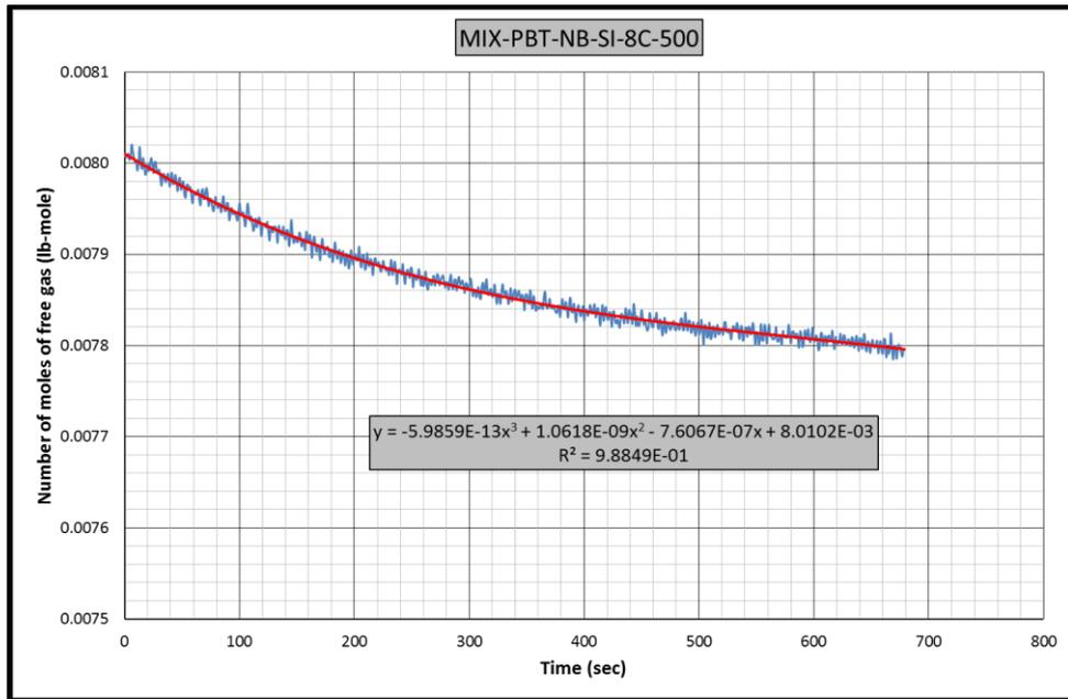
**Figure B.57** Gas consumption rate equation-2 for CH<sub>4</sub>-C<sub>3</sub>H<sub>8</sub>-PBT-NB-SI-8C experiment
