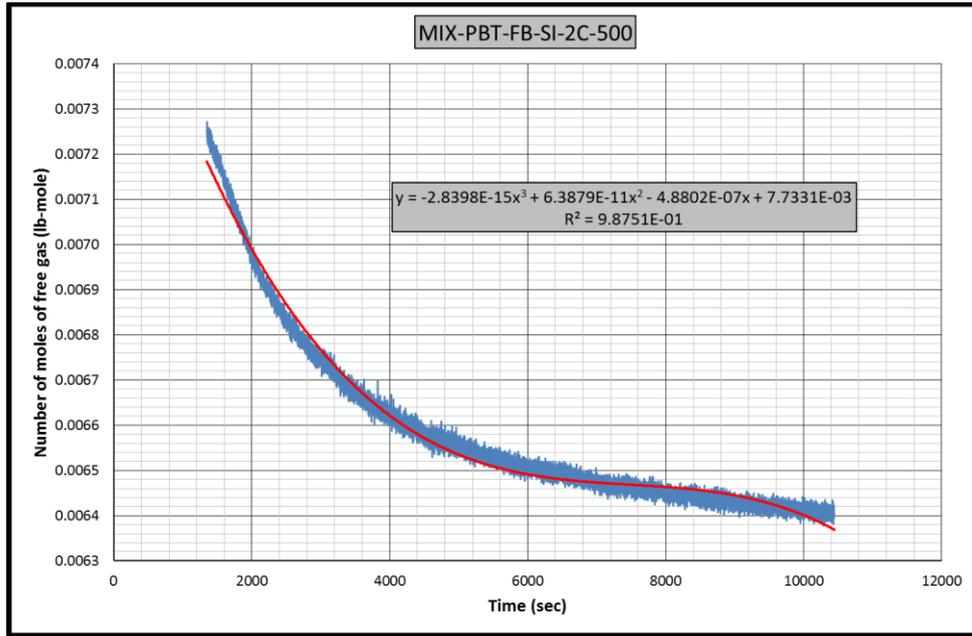
**Figure B.71** Gas consumption rate equation-2 for CH<sub>4</sub>-C<sub>3</sub>H<sub>8</sub>-PBT-FB-SI-2C experiment
