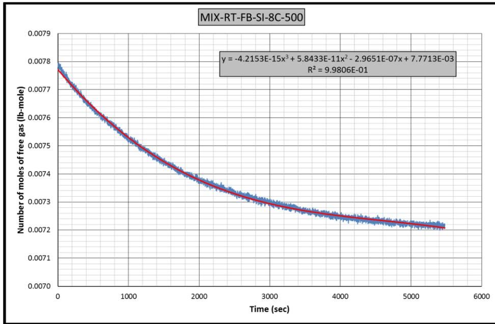
**Figure B.59** Gas consumption rate equation for CH<sub>4</sub>-C<sub>3</sub>H<sub>8</sub>-RT-FB-SI-8C experiment
