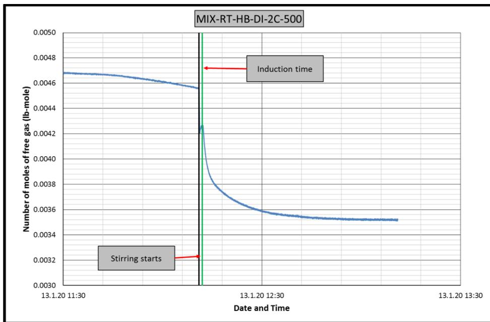
Figure B.106 Change in number of moles of free gas in CH<sub>4</sub>-C<sub>3</sub>H<sub>8</sub>-RT-HB-DI-2C experiment
