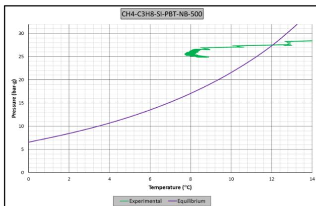
**Figure A.28** Raw data of experiment CH4-C3H8-PBT-NB-SI-500. A: Pressure – temperature vs. time graph, B: Pressure – torque vs. time graph, C: Pressure vs. temperature graph. (Driving force=8.5)
