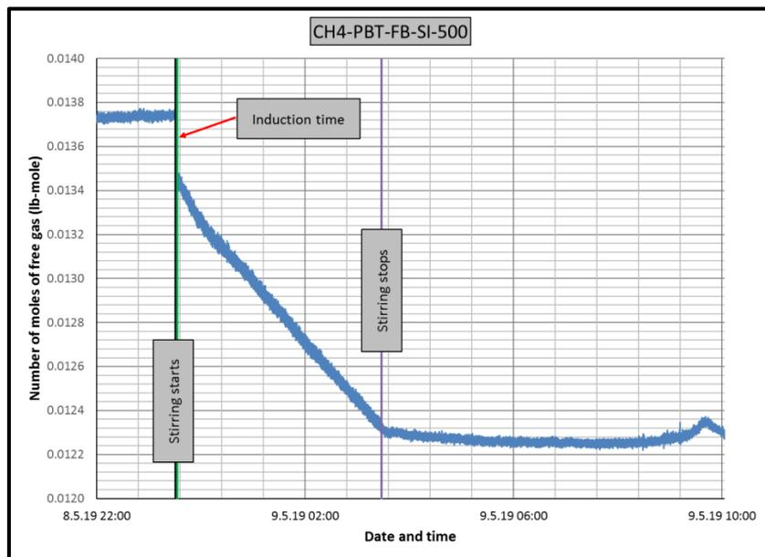
*Figure B.1* Change in number of moles of free gas in CH4-PBT-FB-SI experiment.
