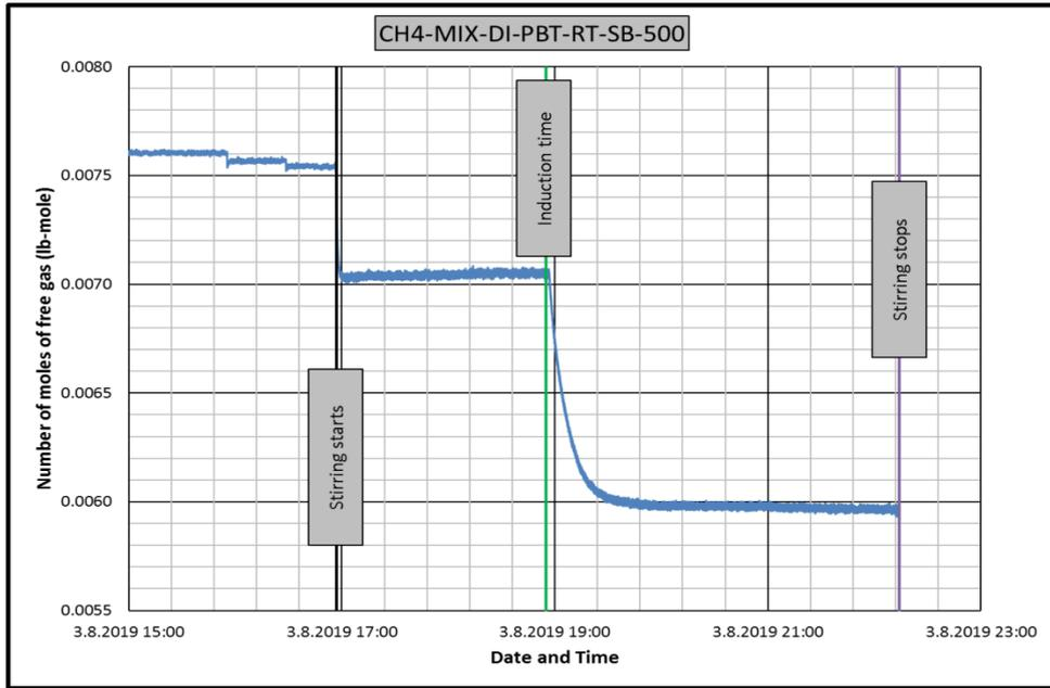
Figure B.45 Change in number of moles of free gas in CH4-MIX-PBT-RT-SB-DI experiment
