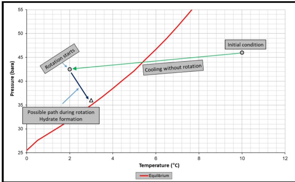
*Figure 5.12* Experimental conditions of methane experiments
