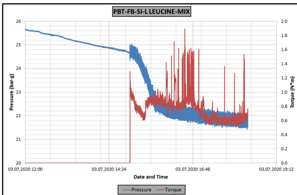
**Figure A.54** Raw data experiment PBT-FB-SI-L LEUCINE-MIX, A: Pressure, temperature vs time graph, B: Pressure, torque vs time graph
