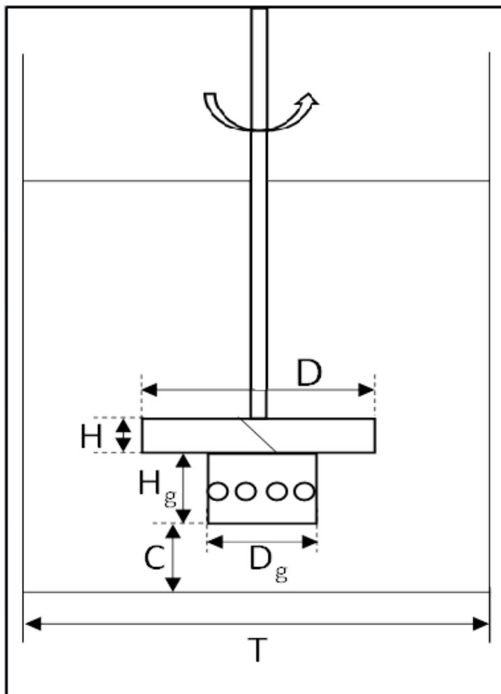
**Figure 5.4** Dimensions and position of mixing elements for PBT impeller
