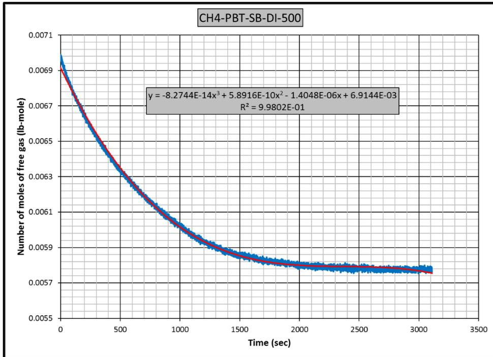
Figure B.22 Gas consumption rate equation for CH4-PBT-SB-DI experiment
