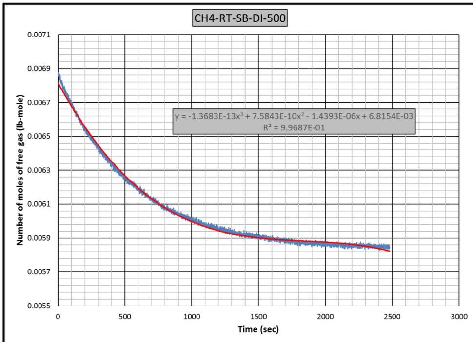
**Figure B.30** Gas consumption rate equation for CH4-RT-SB-DI experiment
