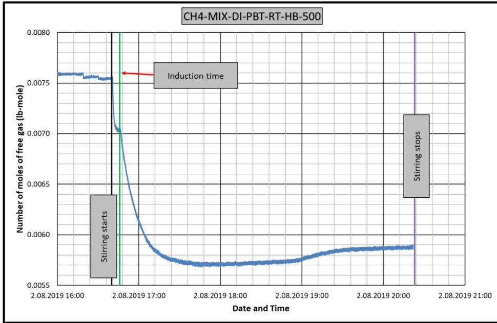
Figure B.43 Change in number of moles of free gas in CH4-MIX-PBT-RT-HB-DI experiment
