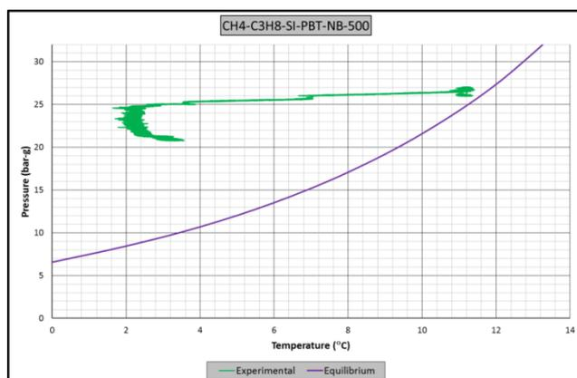
**Figure A.36** Raw data of experiment CH4-C3H8-PBT-NB-SI-500. A: Pressure – temperature vs. time graph, B: Pressure – torque vs. time graph, C: Pressure vs. temperature graph. (Driving force=16)
