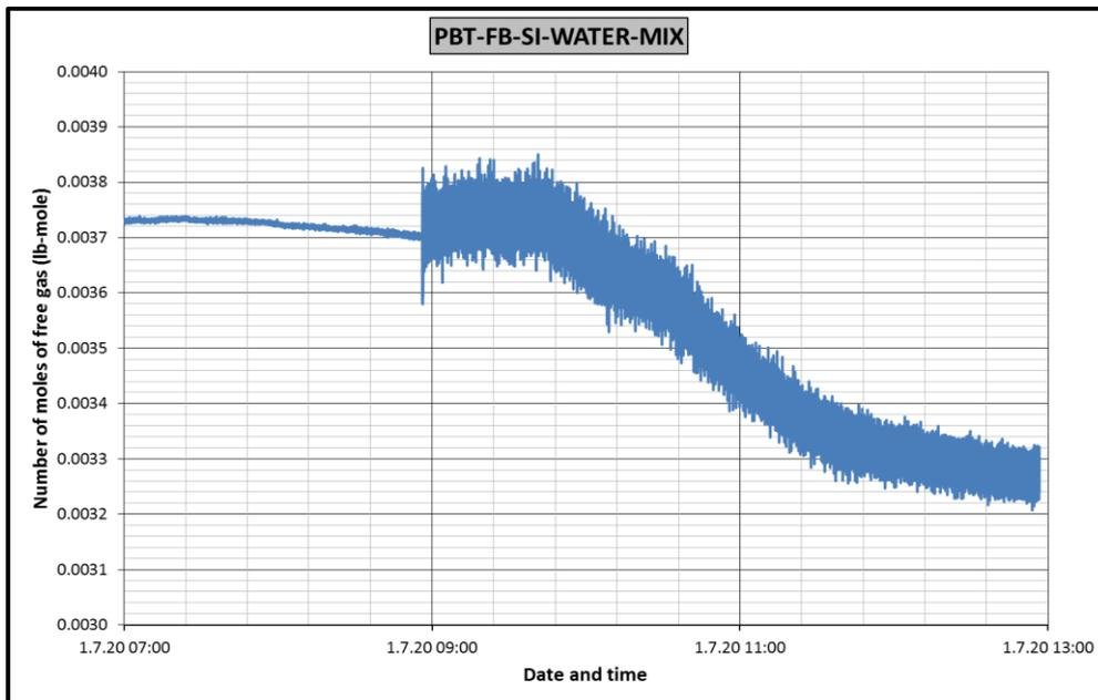
**Figure B.114** Change in number of moles of free gas in PBT-FB-SI-WATER-MIX experiment
