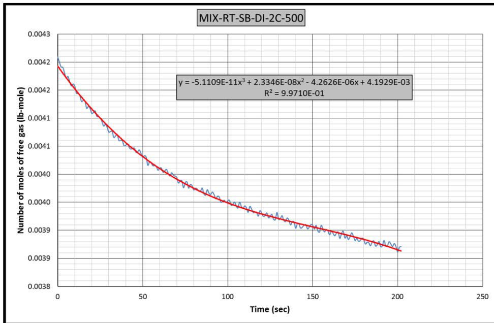
**Figure B.110** Gas consumption rate equation-1 for CH<sub>4</sub>-C<sub>3</sub>H<sub>8</sub>-RT-SB-DI-2C experiment
