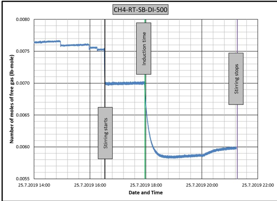
**Figure B.29** Change in number of moles of free gas in CH4-RT-SB-DI experiment
