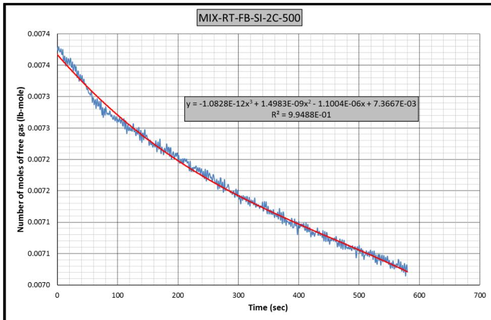
**Figure B.80** Gas consumption rate equation-1 for CH<sub>4</sub>-C<sub>3</sub>H<sub>8</sub>-RT-FB-SI-2C experiment
