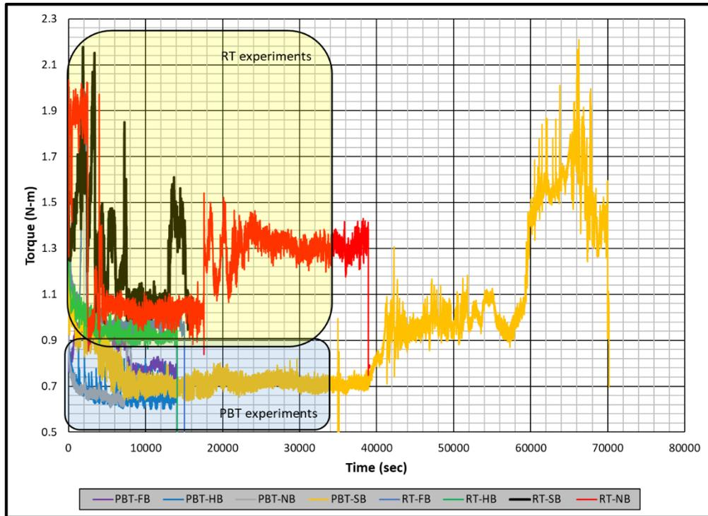
**Figure 6.10** Recorded torque values of single impeller experiments
