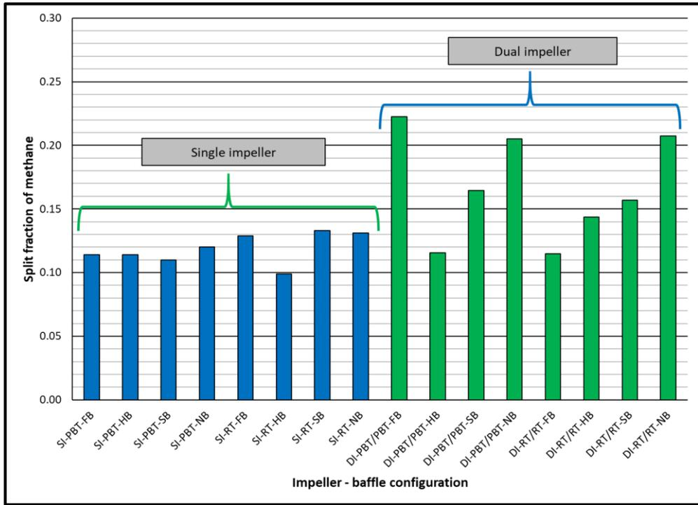
**Figure 7.11** Split fraction of methane for single and dual impeller experiments (experimental temperature 2 °C)
