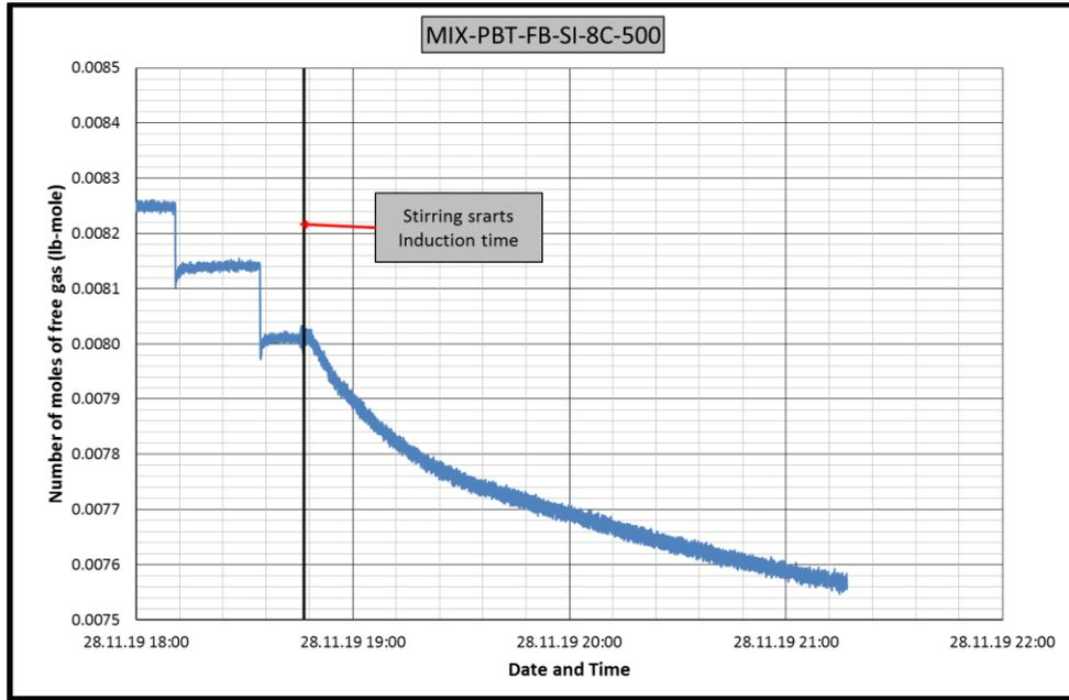
*Figure B.49* Change in number of moles of free gas in CH<sub>4</sub>-C<sub>3</sub>H<sub>8</sub>-PBT-FB-SI-8C experiment
