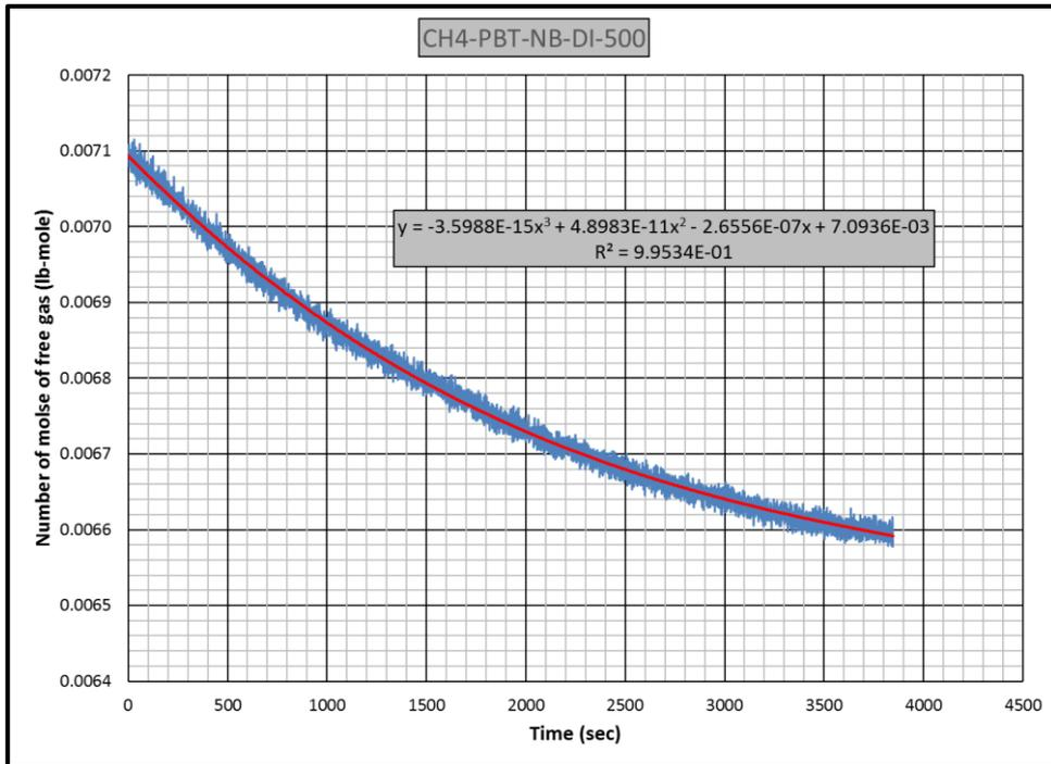
**Figure B.24** Gas consumption rate equation for CH4-PBT-NB-DI experiment
