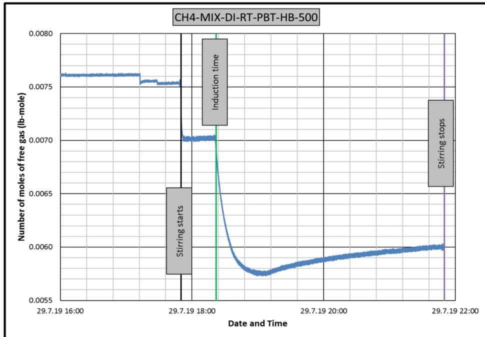
Figure B.35 Change in number of moles of free gas in CH4-MIX-RT-PBT-HB-DI experiment
