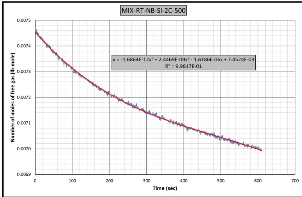
**Figure B.89** Gas consumption rate equation-1 for CH<sub>4</sub>-C<sub>3</sub>H<sub>8</sub>-RT-NB-SI-2C experiment
