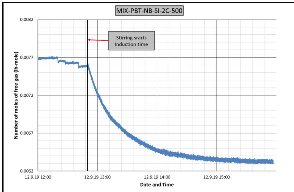
Figure B.76 Change in number of moles of free gas in CH<sub>4</sub>-C<sub>3</sub>H<sub>8</sub>-PBT-NB-SI-2C experiment
