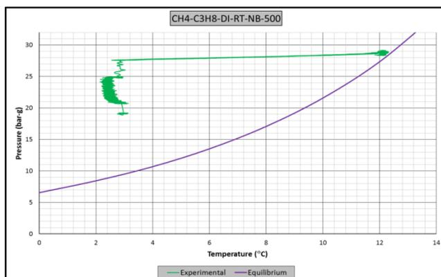
**Figure A.48** Raw data of experiment CH<sub>4</sub>-C<sub>3</sub>H<sub>8</sub>-RT-NB-DI-500. A: Pressure – temperature vs. time graph, B: Pressure – torque vs. time graph, C: Pressure vs. temperature graph. (Driving force=16)
