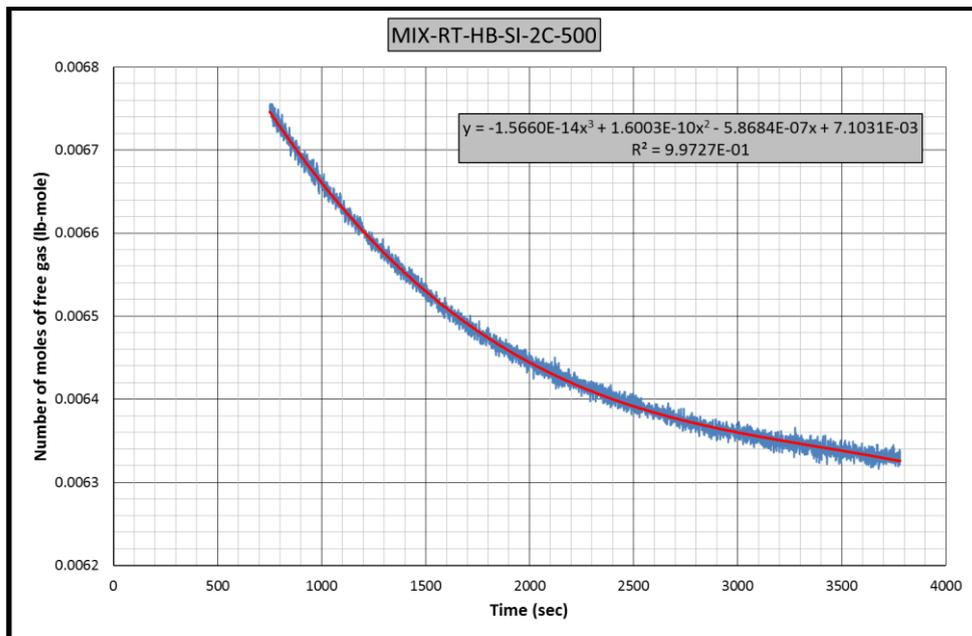
**Figure B.84** Gas consumption rate equation-2 for CH<sub>4</sub>-C<sub>3</sub>H<sub>8</sub>-RT-HB-SI-2C experiment
