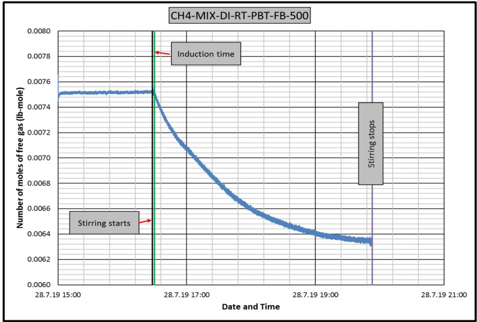
**Figure B.33** Change in number of moles of free gas in CH4-MIX-RT-PBT-FB-DI experiment
