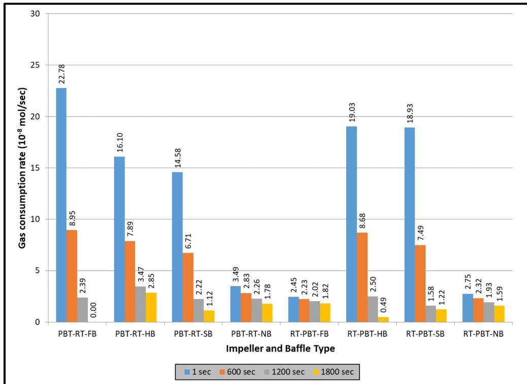
**Figure 6.16** Rate of hydrate formation of dual mixed impellers for time period of 1, 600, 1200 and 1800 seconds.
