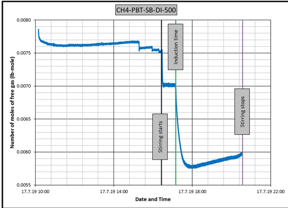
Figure B.21 Change in number of moles of free gas in CH4-PBT-SB-DI experiment
