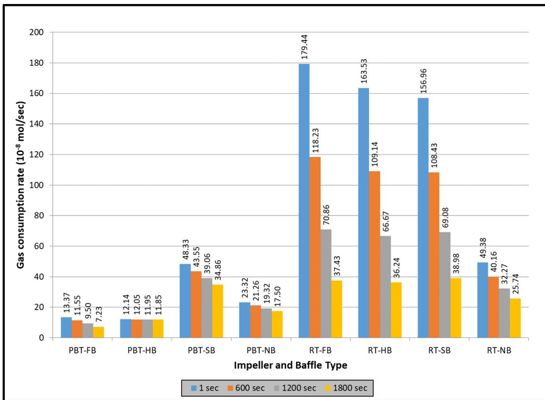
**Figure 6.7** Rate of hydrate formation in single impeller experiments
