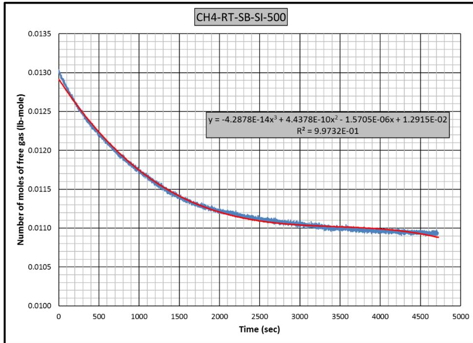
Figure B.14 Gas consumption rate equation for CH4-RT-SB-SI experiment
