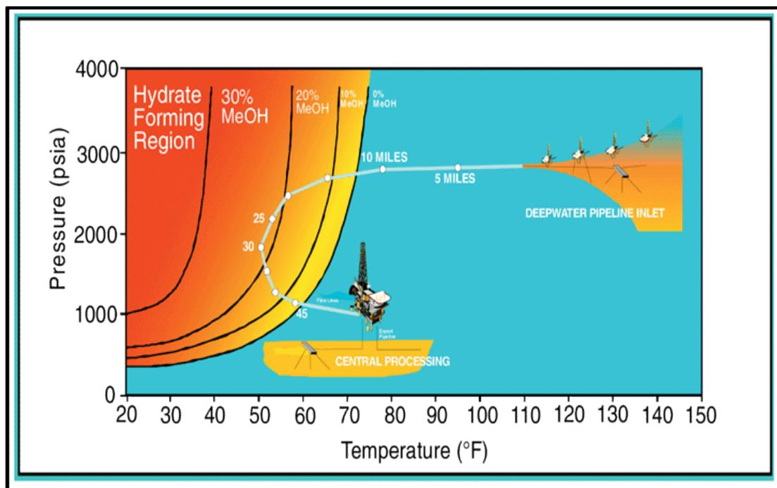
**Figure 3.3** Phase boundary of methane hydrates [117]
