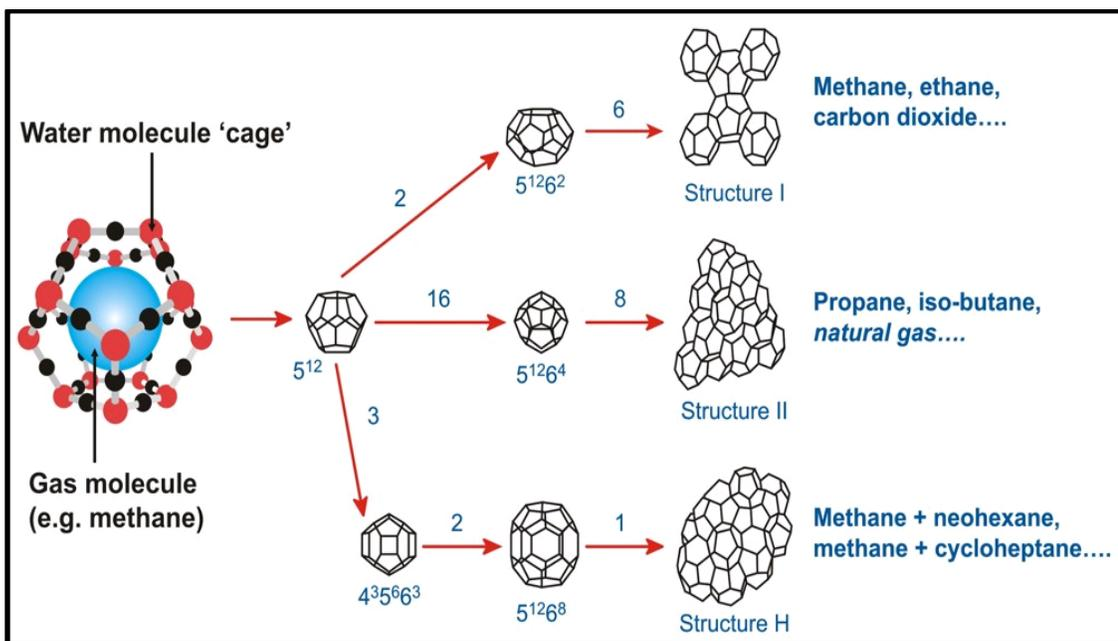
**Figure 2.4** Structures of gas hydrates [5]
