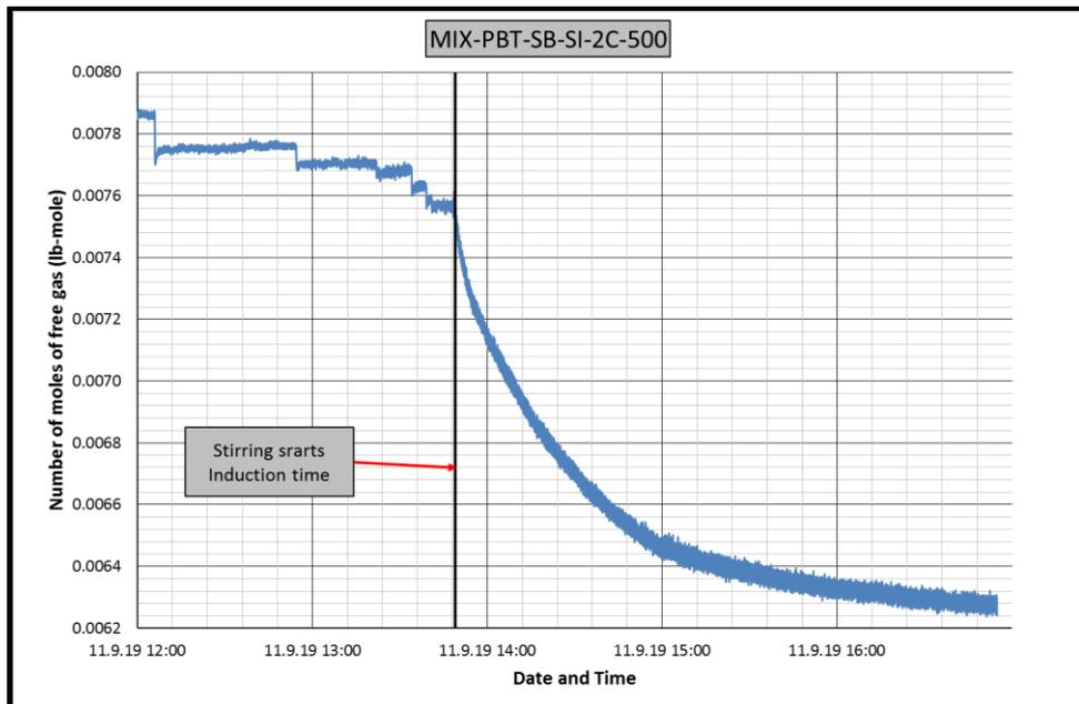
Figure B.74 Change in number of moles of free gas in CH<sub>4</sub>-C<sub>3</sub>H<sub>8</sub>-PBT-SB-SI-2C experiment
