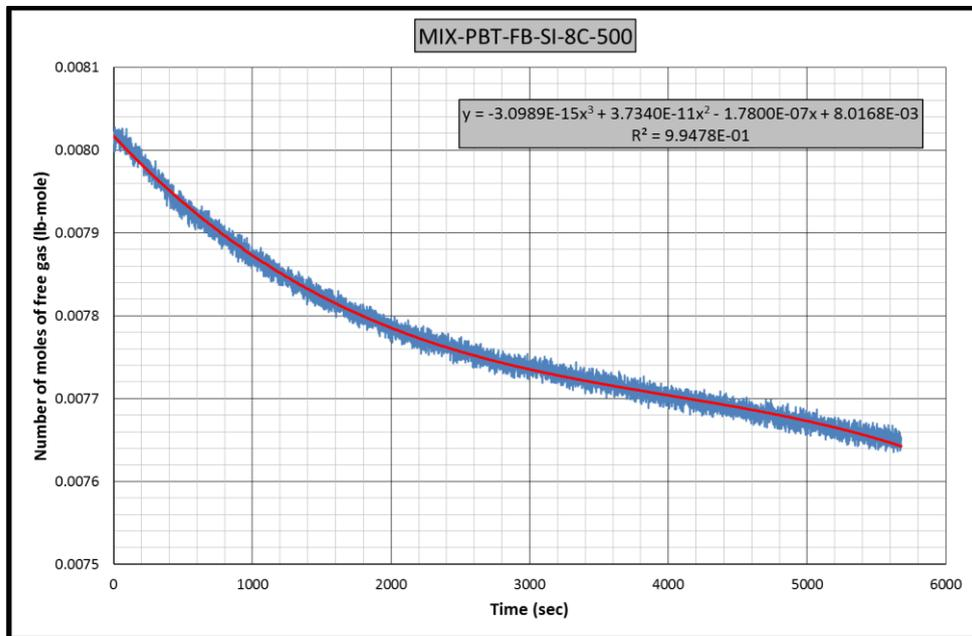
*Figure B.50* Gas consumption rate equation for CH<sub>4</sub>-C<sub>3</sub>H<sub>8</sub>-PBT-FB-SI-8C experiment
