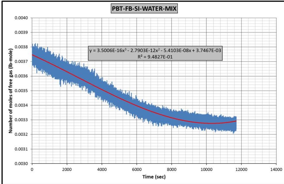
**Figure B.115** Gas consumption rate equation for PBT-FB-SI-WATER-MIX experiment
