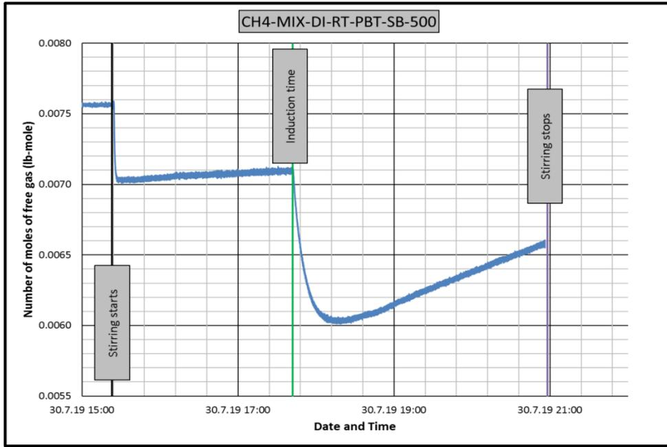
**Figure B.39** Change in number of moles of free gas in CH4-MIX-RT-PBT-SB-DI experiment
