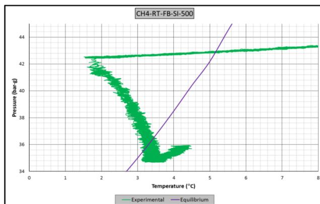
**Figure A.5** Raw data of experiment CH4-RT-FB-SI-500. A: Pressure – temperature vs. time graph, B: Pressure – torque vs. time graph, C: Pressure vs. temperature graph
