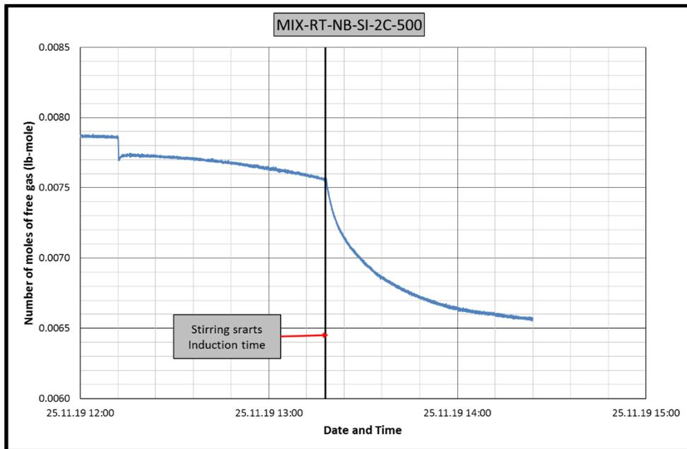
**Figure B.88** Change in number of moles of free gas in CH<sub>4</sub>-C<sub>3</sub>H<sub>8</sub>-RT-NB-SI-2C experiment
