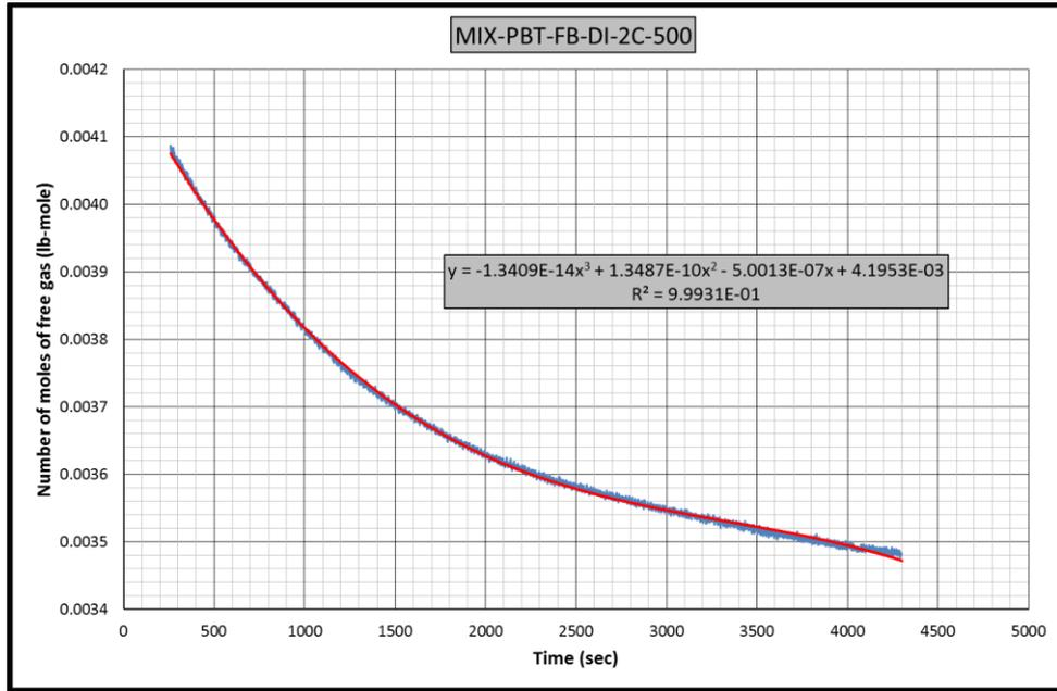
Figure B.93 Gas consumption rate equation-2 for CH<sub>4</sub>-C<sub>3</sub>H<sub>8</sub>-PBT-FB-DI-2C experiment
