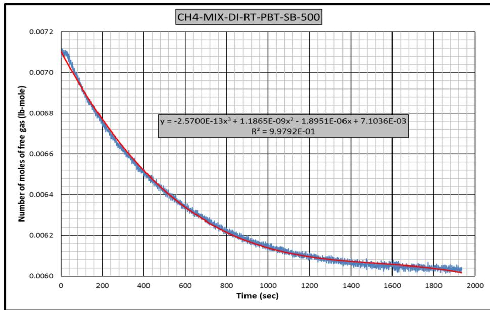
**Figure B.40** Gas consumption rate equation for CH4-MIX-RT-PBT-SB-DI experiment
