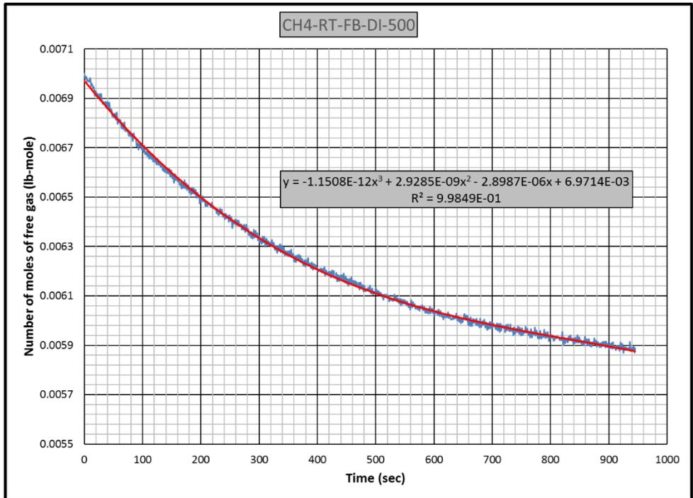
Figure B.26 Gas consumption rate equation for CH4-RT-FB-DI experiment
