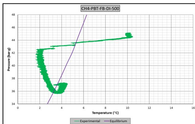
**Figure A.9** Raw data of experiment CH4-PBT-FB-DI-500. A: Pressure – temperature vs. time graph, B: Pressure – torque vs. time graph, C: Pressure vs. temperature graph
