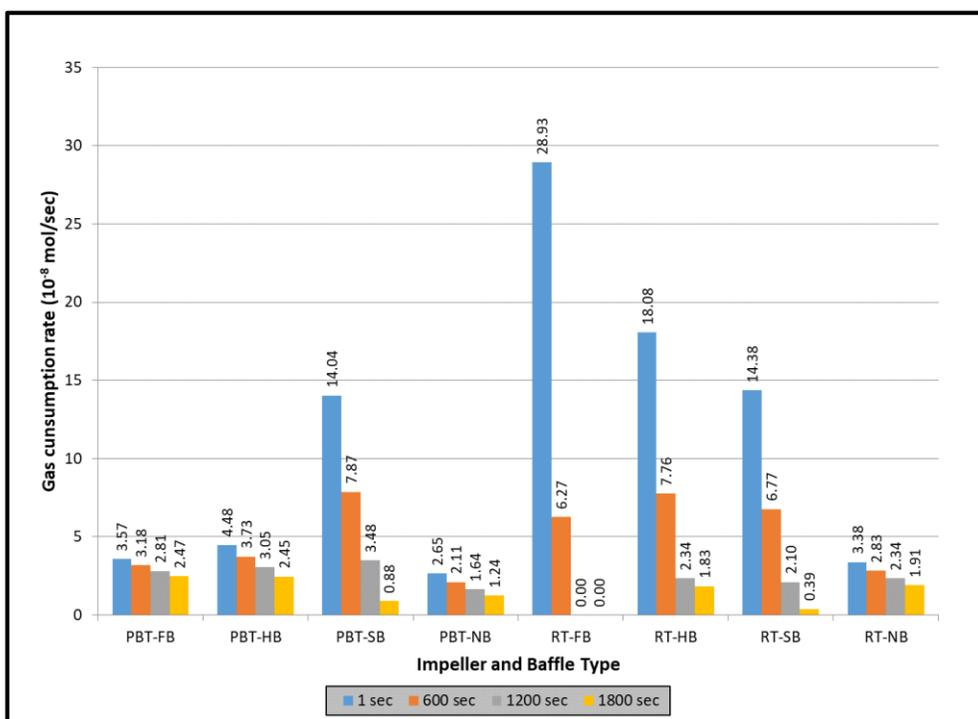
Figure 6.13 Rate of hydrate formation of PBT/PBT and RT/RT dual impellers for time period of 1, 600, 1200 and 1800 seconds
