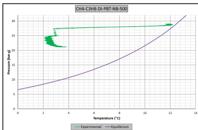
**Figure A.44** Raw data of experiment CH4-C3H8-PBT-NB-DI-500. A: Pressure – temperature vs. time graph, B: Pressure – torque vs. time graph, C: Pressure vs. temperature graph. (Driving force=16)
