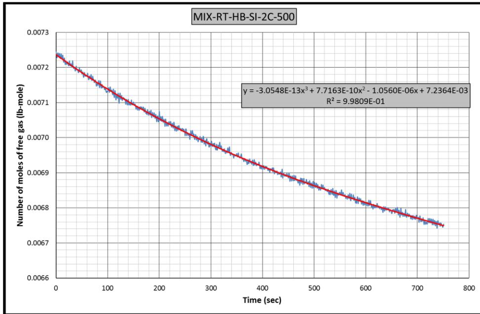
**Figure B.83** Gas consumption rate equation-1 for CH<sub>4</sub>-C<sub>3</sub>H<sub>8</sub>-RT-HB-SI-2C experiment
