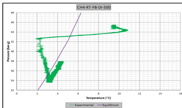
**Figure A.13** Raw data of experiment CH4-RT-FB-DI-500. A: Pressure – temperature vs. time graph, B: Pressure – torque vs. time graph, C: Pressure vs. temperature graph
