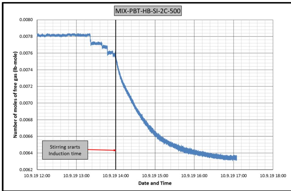
**Figure B.72** Change in number of moles of free gas in CH<sub>4</sub>-C<sub>3</sub>H<sub>8</sub>-PBT-HB-SI-2C experiment
