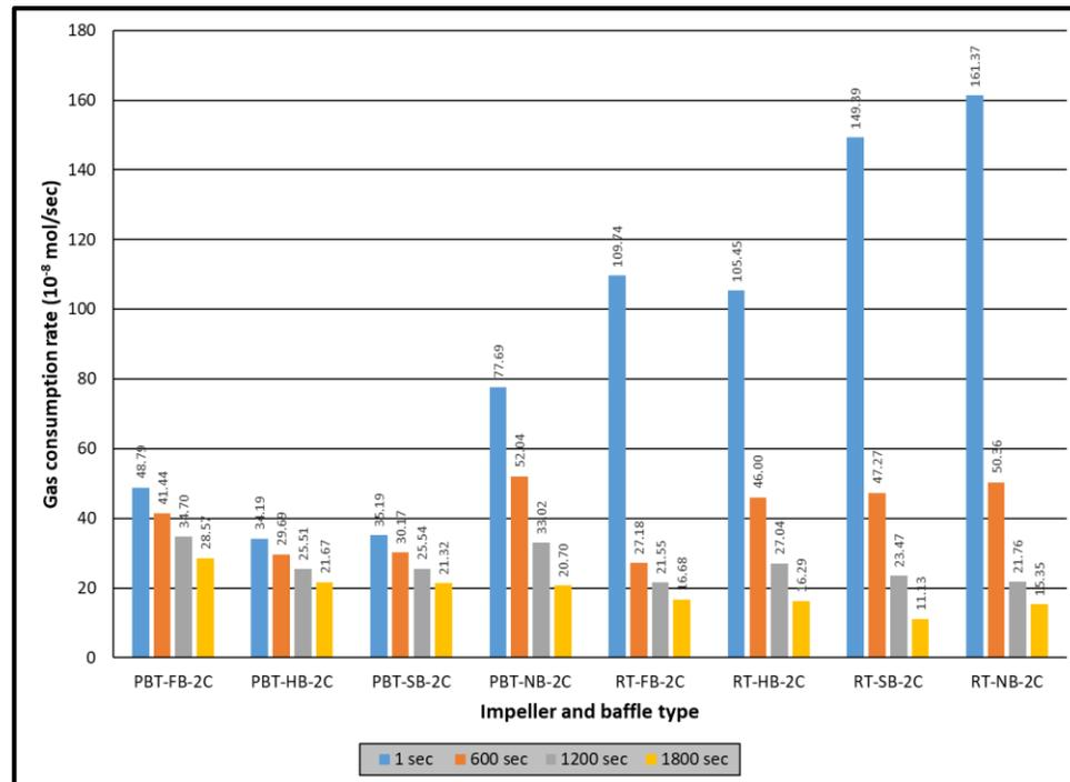
**Figure 7.10** Rate of hydrate formation of mixture gas with single impeller and higher driving force (experimental temperature 2 °C)
