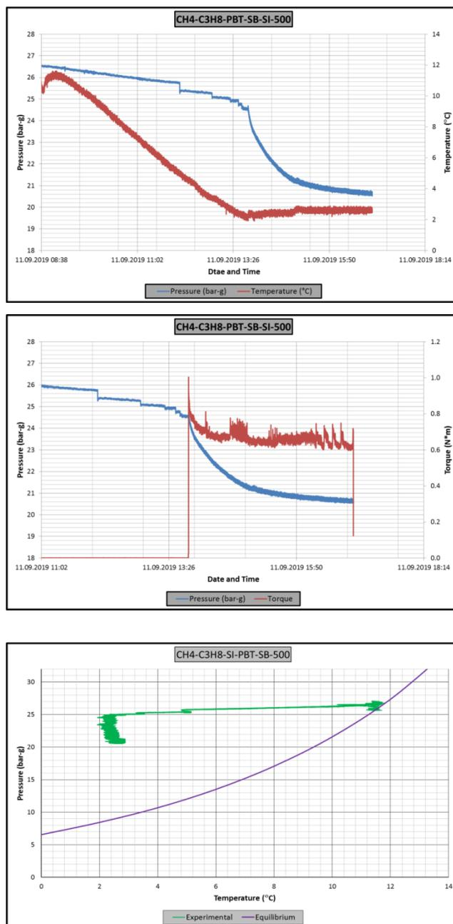
**Figure A.35** Raw data of experiment CH4-C3H8-PBT-SB-SI-500. A: Pressure – temperature vs. time graph, B: Pressure – torque vs. time graph, C: Pressure vs. temperature graph. (Driving force=16)
