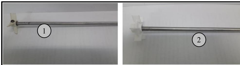
*Figure 5.11* Single impeller for transparent reactor
