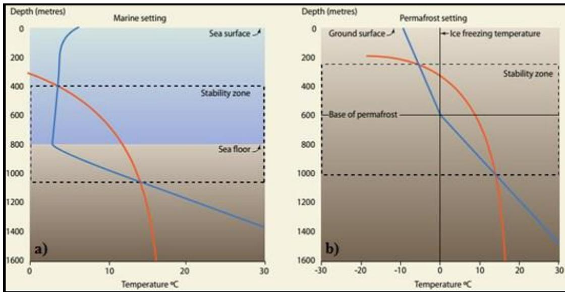
**Figure 2.6** Gas hydrate stability conditions for a) marine hydrates b) permafrost hydrates (Orange curve: hydrate equilibrium curve, Blue curve: thermal gradient curve) [47]
