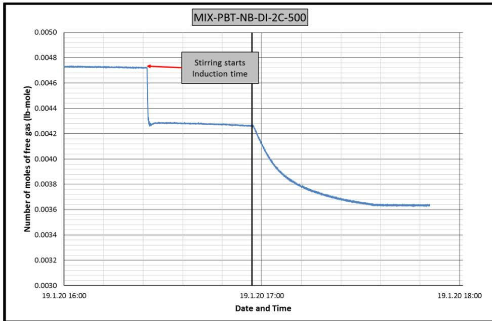
Figure B.100 Change in number of moles of free gas in CH<sub>4</sub>-C<sub>3</sub>H<sub>8</sub>-PBT-NB-DI-2C experiment
