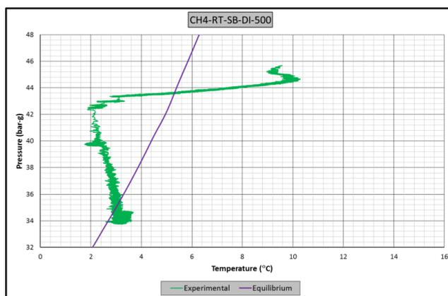
**Figure A.15** Raw data of experiment CH4-RT-SB-DI-500. A: Pressure – temperature vs. time graph, B: Pressure – torque vs. time graph, C: Pressure vs. temperature graph
