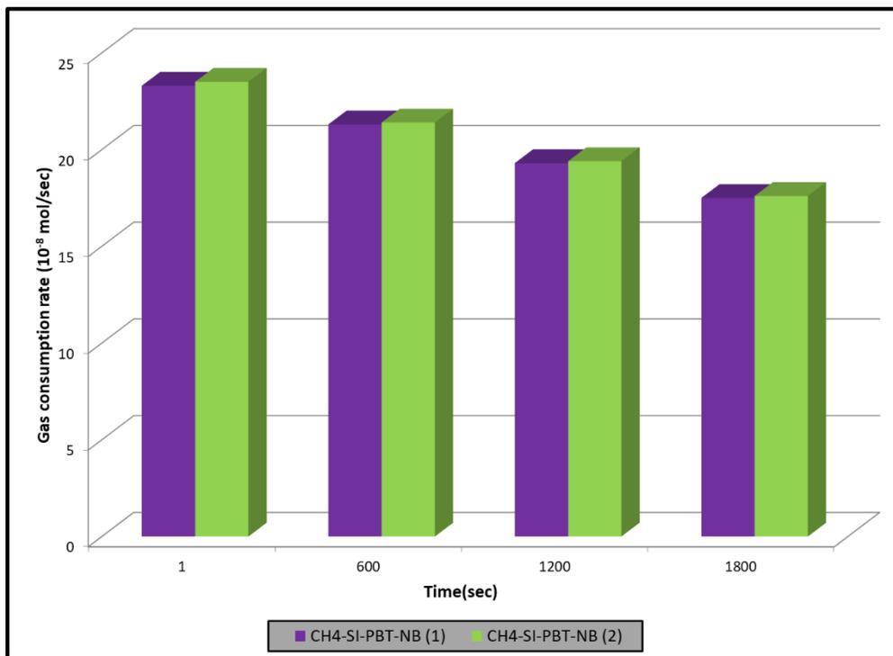
**Figure 6.17** Repeatability test of CH4-SI-PBT-NB in terms of gas consumption rate
