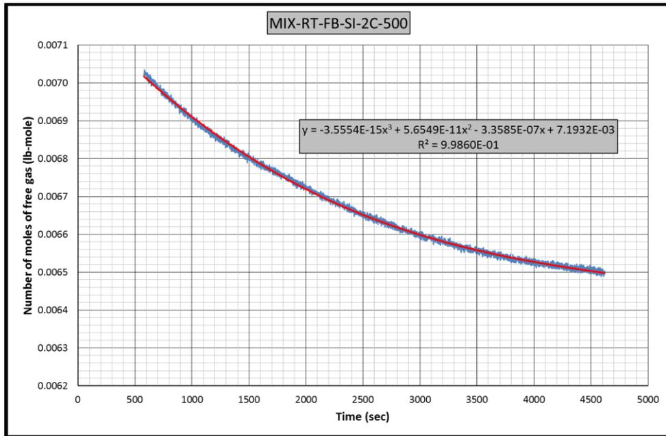
**Figure B.81** Gas consumption rate equation-2 for CH<sub>4</sub>-C<sub>3</sub>H<sub>8</sub>-RT-FB-SI-2C experiment
