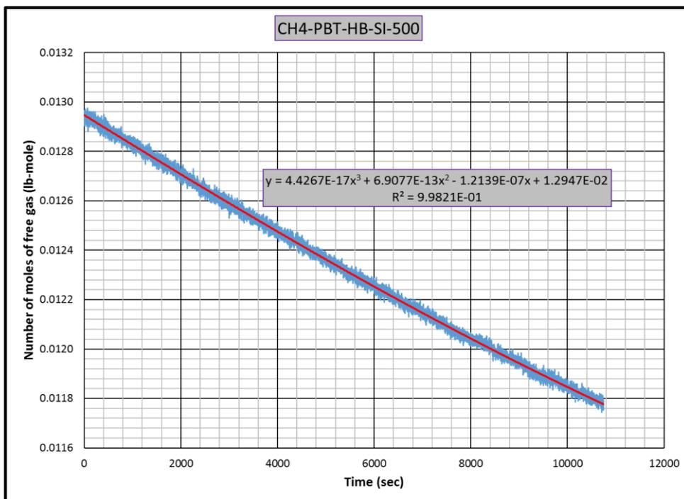
**Figure B.4** Gas consumption rate equation for CH4-PBT-HB-SI experiment
