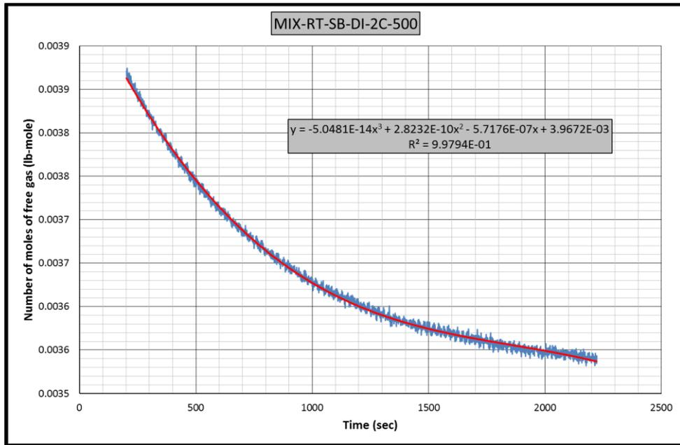
**Figure B.111** Gas consumption rate equation-2 for CH<sub>4</sub>-C<sub>3</sub>H<sub>8</sub>-RT-SB-DI-2C experiment
