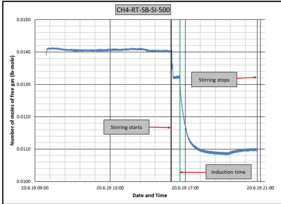
Figure B.13 Change in number of moles of free gas in CH4-RT-SB-SI experiment
