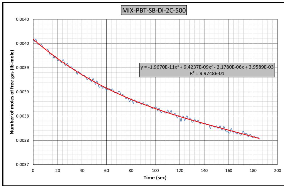
**Figure B.98** Gas consumption rate equation-1 for CH<sub>4</sub>-C<sub>3</sub>H<sub>8</sub>-PBT-SB-DI-2C experiment
