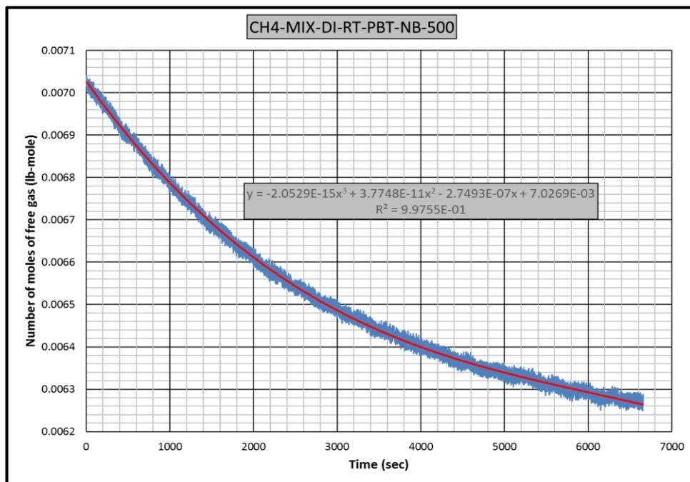
**Figure B.38** Gas consumption rate equation for CH4-MIX-RT-PBT-NB-DI experiment
