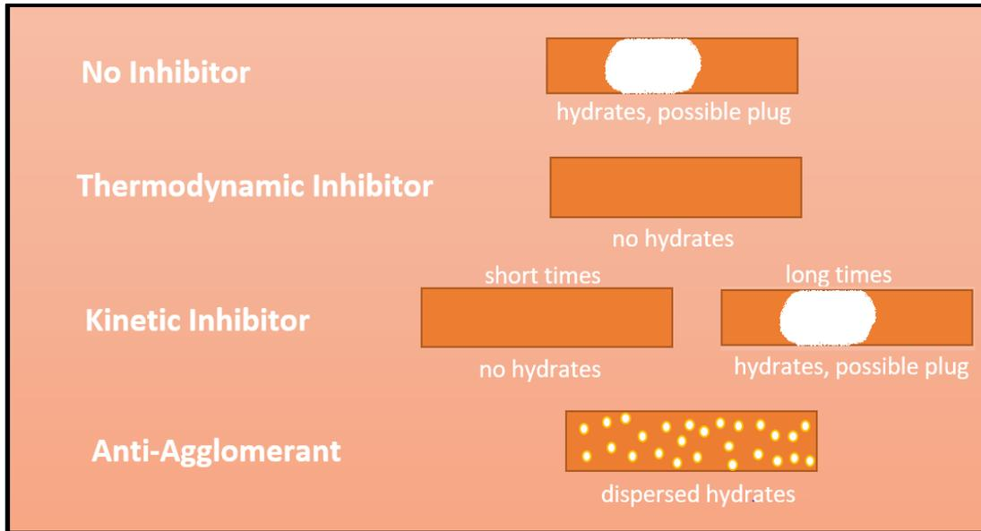
*Figure 3.2* Design of different behaviors from inhibitors
