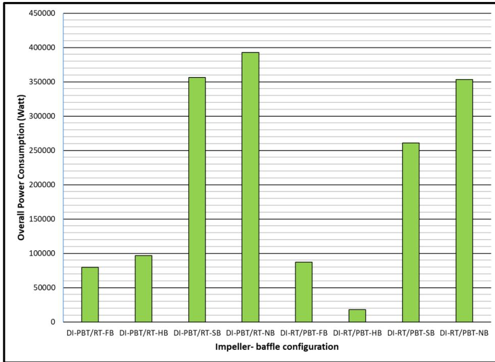
**Figure 6.14** Overall power consumption of dual-mixed impeller experiments
