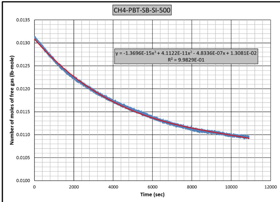
**Figure B.6** Gas consumption rate equation for CH4-PBT-SB-SI experiment
