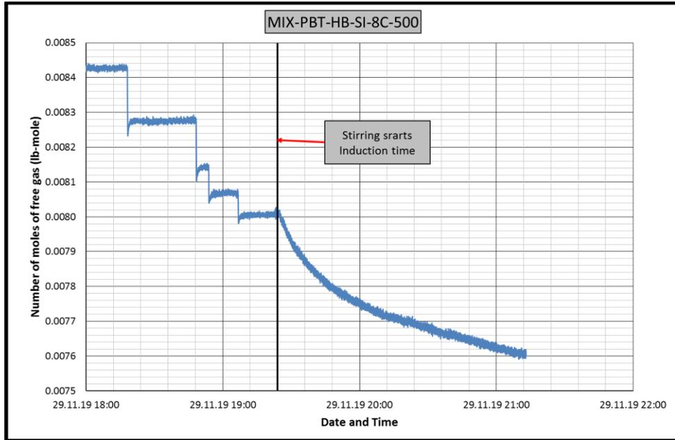
**Figure B.51** Change in number of moles of free gas in CH<sub>4</sub>-C<sub>3</sub>H<sub>8</sub>-PBT-HB-SI-8C experiment
