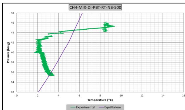
**Figure A.20** Raw data of experiment CH4-PBT-RT-NB-MIX-DI-500. A: Pressure – temperature vs. time graph, B: Pressure – torque vs. time graph, C: Pressure vs. temperature graph
