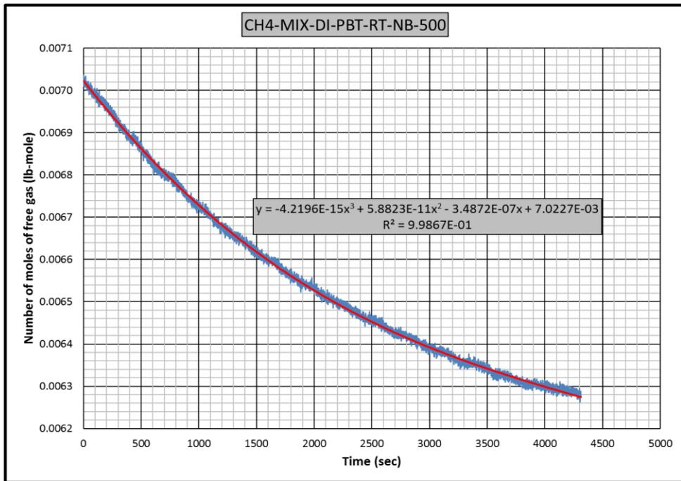
**Figure B.48** Gas consumption rate equation for CH4-MIX-PBT-RT-NB-DI experiment
