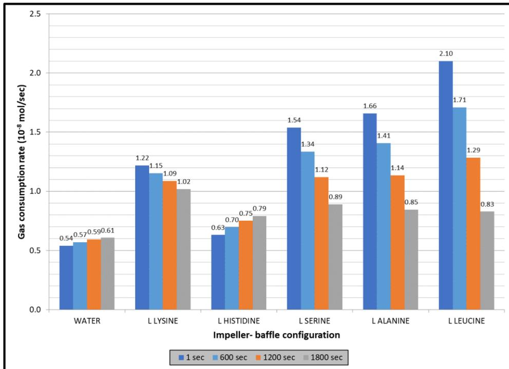
**Figure 8.2** Hydrate formation rates of methane-propane mixture and amino acid solutions
