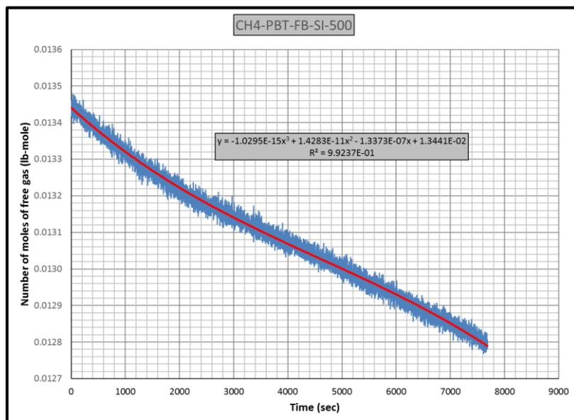
*Figure B.2* Gas consumption rate equation for CH4-PBT-FB-SI experiment
