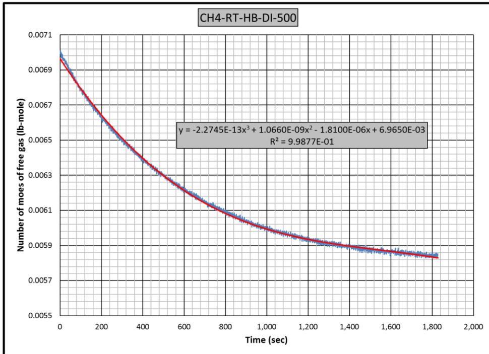
**Figure B.28** Gas consumption rate equation for CH4-RT-HB-DI experiment
