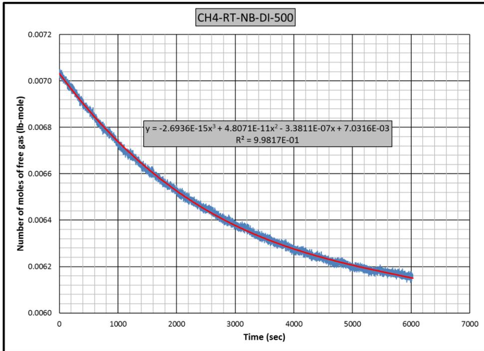
Figure B.32 Gas consumption rate equation for CH4-RT-NB-DI experiment
