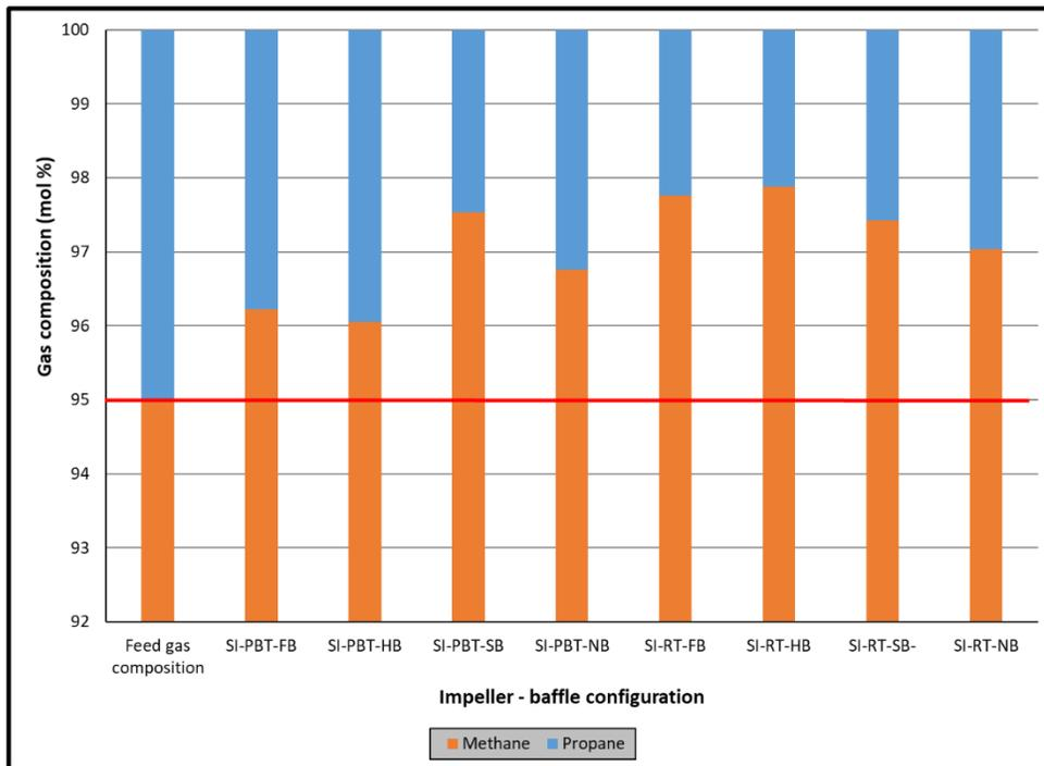
Figure 7.5 Composition of feed gas and free gas at the end of single impeller experiments (lower driving force)
