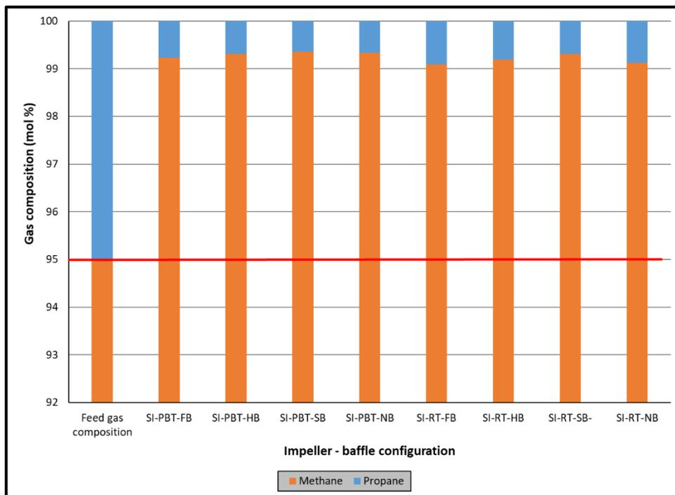
**Figure 7.6** Composition of feed gas and free gas at the end of single impeller experiments (higher driving force)
