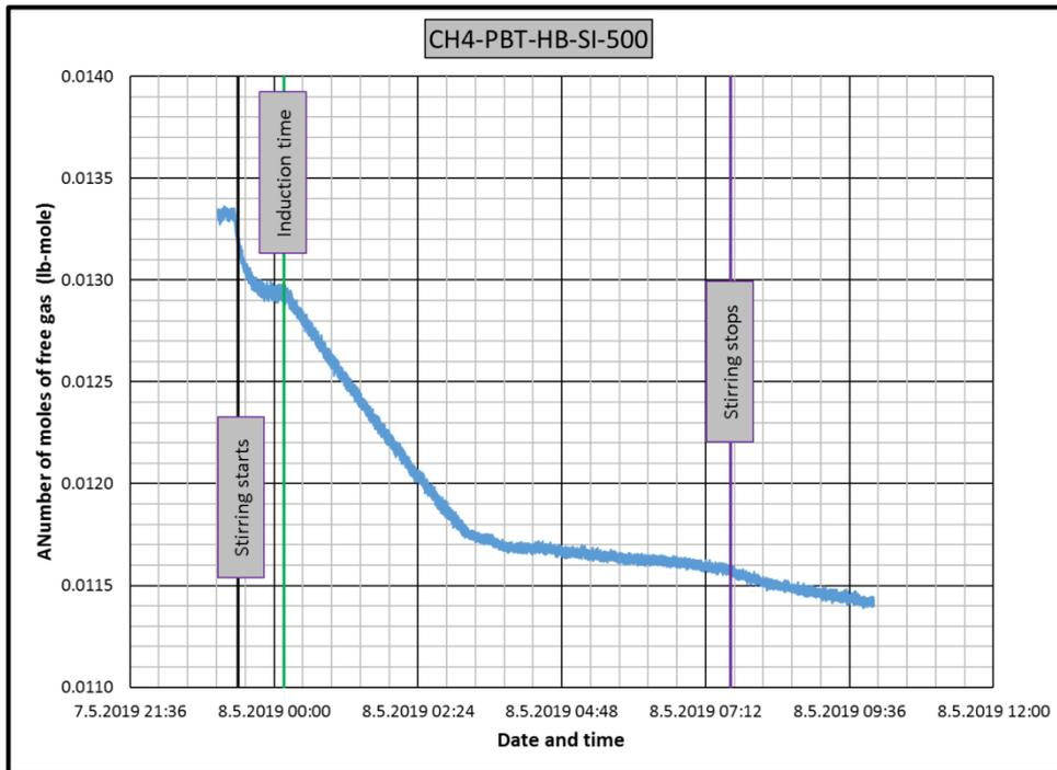
**Figure B.3** Change in number of moles of free gas in CH4-PBT-HB-SI experiment
