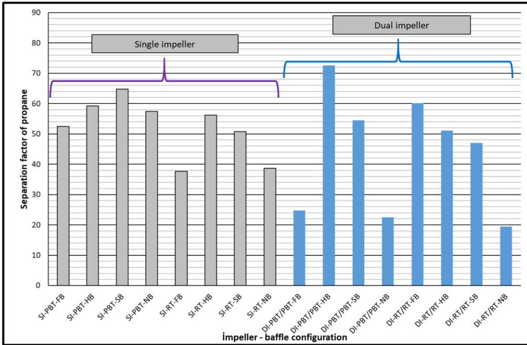
**Figure 7.13** Separation factor of propane for single and dual impeller experiments (experimental temperature 2 °C)
