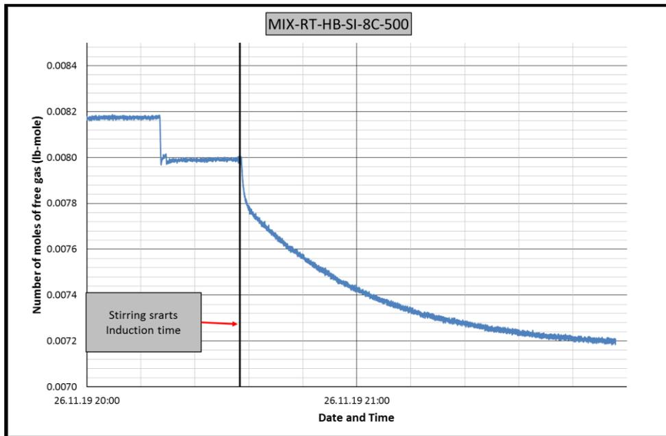
**Figure B.60** Change in number of moles of free gas in CH<sub>4</sub>-C<sub>3</sub>H<sub>8</sub>-RT-HB-SI-8C experiment
