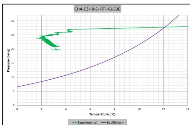
**Figure A.38** Raw data of experiment CH4-C3H8-RT-HB-SI-500. A: Pressure – temperature vs. time graph, B: Pressure – torque vs. time graph, C: Pressure vs. temperature graph. (Driving force=16)
