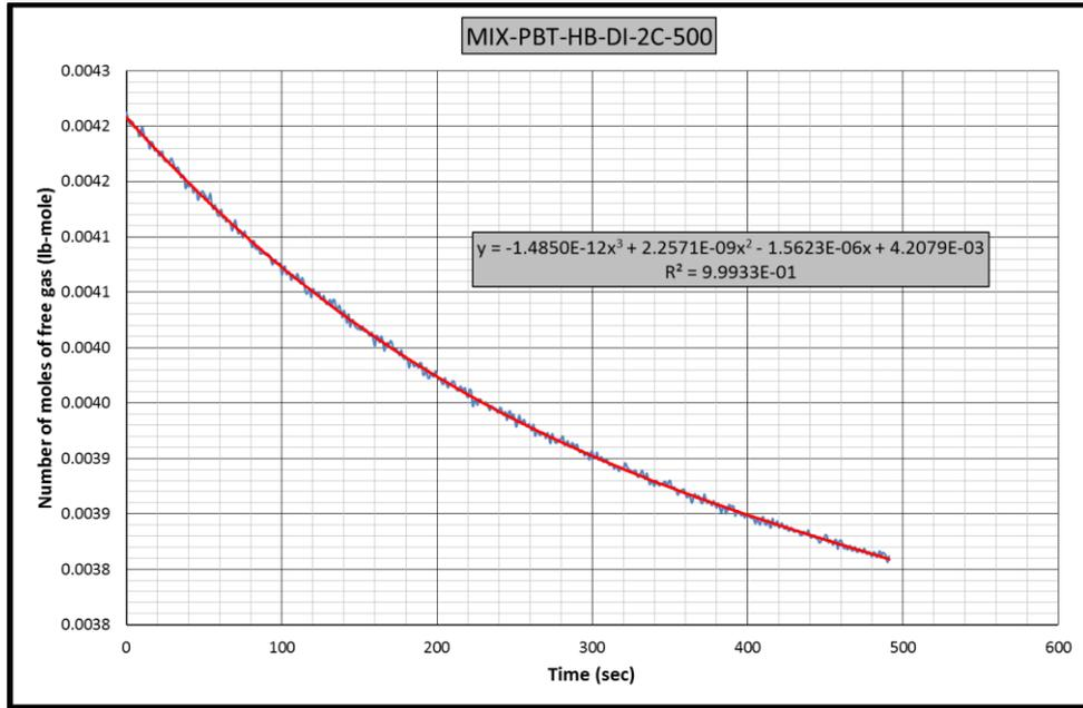
*Figure B.95* Gas consumption rate equation-1 for CH<sub>4</sub>-C<sub>3</sub>H<sub>8</sub>-PBT-HB-DI-2C experiment
