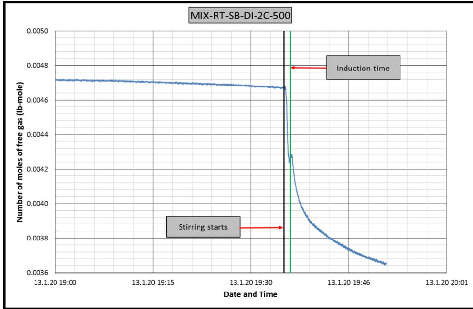
**Figure B.109** Change in number of moles of free gas in CH<sub>4</sub>-C<sub>3</sub>H<sub>8</sub>-RT-SB-DI-2C experiment
