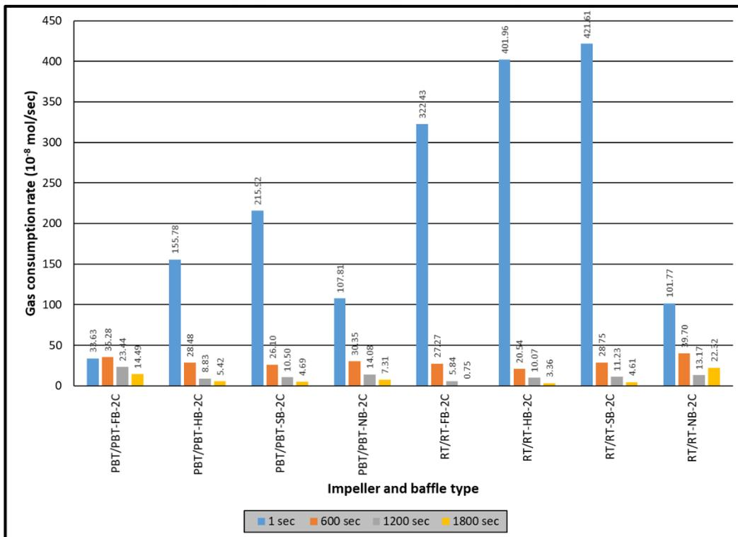
**Figure 7.14** Rate of hydrate formation of mixture gas with dual impeller (experimental temperature 2 °C)
