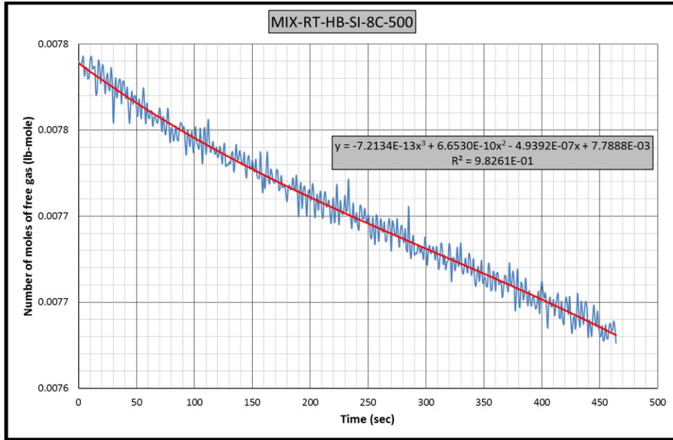
**Figure B.61** Gas consumption rate equation-1 for CH<sub>4</sub>-C<sub>3</sub>H<sub>8</sub>-RT-HB-SI-8C experiment
