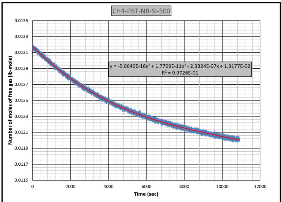
**Figure B.8** Gas consumption rate equation for CH4-PBT-NB-SI experiment
