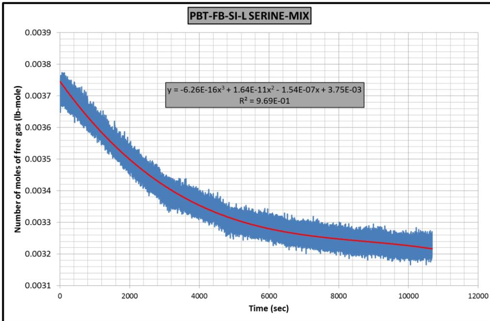
*Figure B.121* Gas consumption rate equation for PBT-FB-SI-L SERINE-MIX experiment
