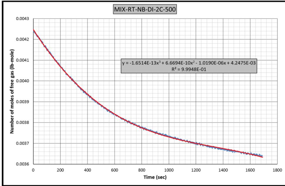
**Figure B.113** Gas consumption rate equation for CH<sub>4</sub>-C<sub>3</sub>H<sub>8</sub>-RT-NB-DI-2C experiment
