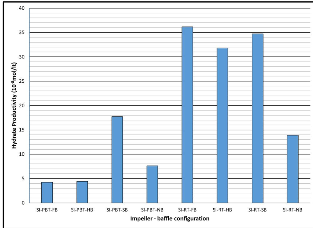
**Figure 6.8** Hydrate productivity of single impeller experiments
