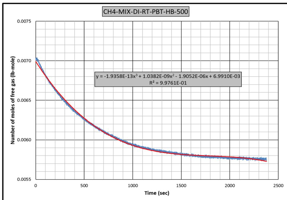
Figure B.36 Gas consumption rate equation for CH4-MIX-RT-PBT-HB-DI experiment
