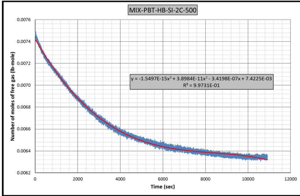
Figure B.73 Gas consumption rate equation for CH<sub>4</sub>-C<sub>3</sub>H<sub>8</sub>-PBT-HB-SI-2C experiment
