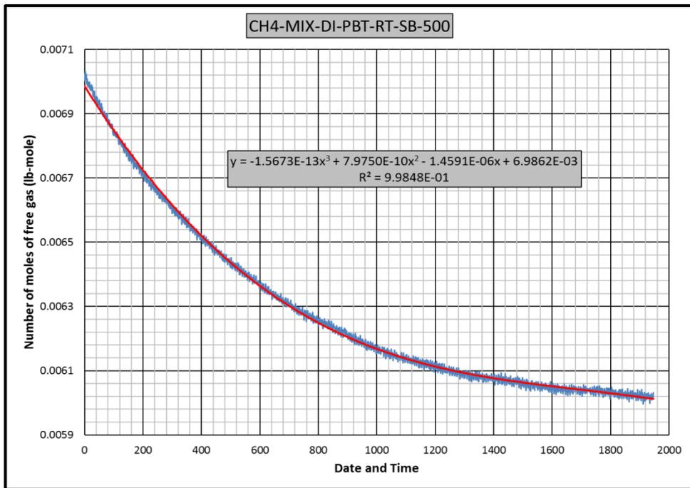
Figure B.46 Gas consumption rate equation for CH4-MIX-PBT-RT-SB-DI experiment
