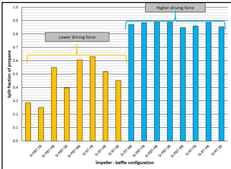
Figure 7.3 Split fraction of propane of single impeller mixture hydrate experiments
