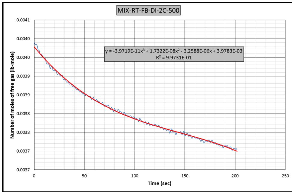
**Figure B.104** Gas consumption rate equation-1 for CH<sub>4</sub>-C<sub>3</sub>H<sub>8</sub>-RT-FB-DI-2C experiment
