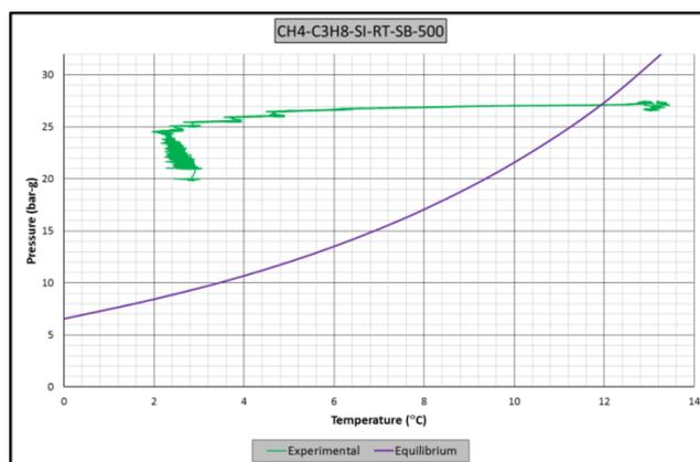
**Figure A.39** Raw data of experiment CH4-C3H8-RT-SB-SI-500. A: Pressure – temperature vs. time graph, B: Pressure – torque vs. time graph, C: Pressure vs. temperature graph. (Driving force=16)
