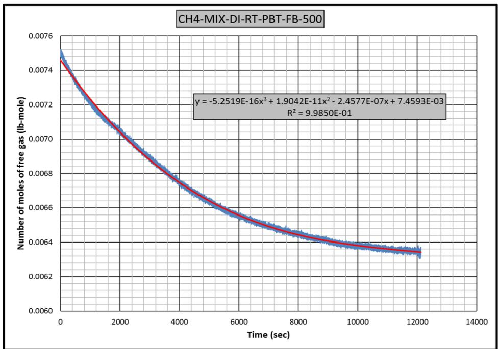
**Figure B.34** Gas consumption rate equation for CH4-MIX-RT-PBT-FB-DI experiment
