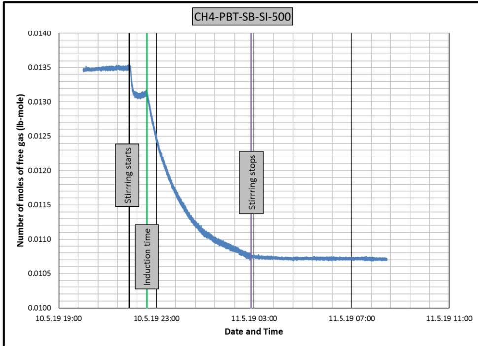
**Figure B.5** Change in number of moles of free gas in CH4-PBT-SB-SI experiment
