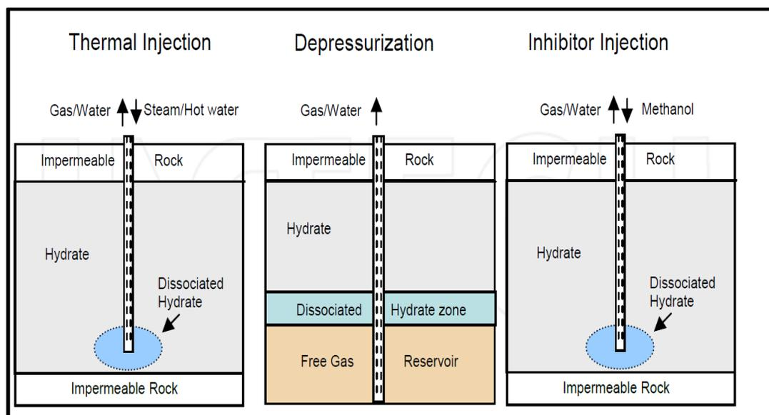
**Figure 2.2** Gas hydrate production methods [27]
