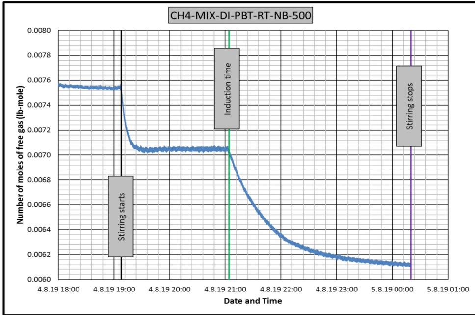
**Figure B.47** Change in number of moles of free gas in CH4-MIX-PBT-RT-NB-DI experiment
