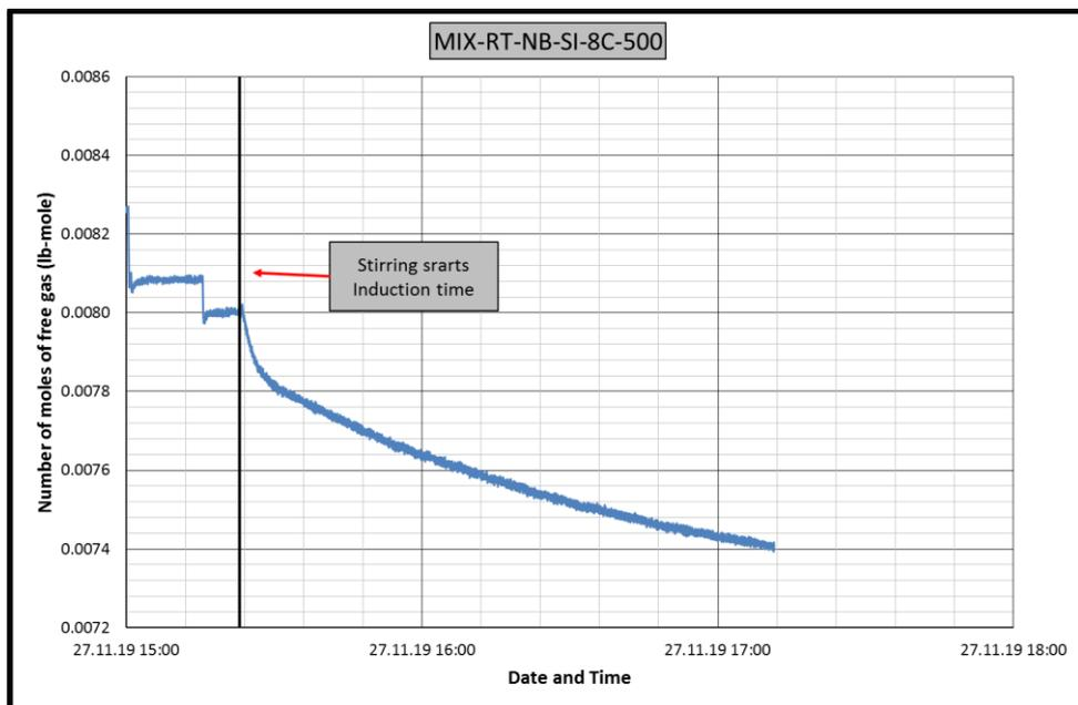
**Figure B.66** Change in number of moles of free gas in CH<sub>4</sub>-C<sub>3</sub>H<sub>8</sub>-RT-NB-SI-8C experiment
