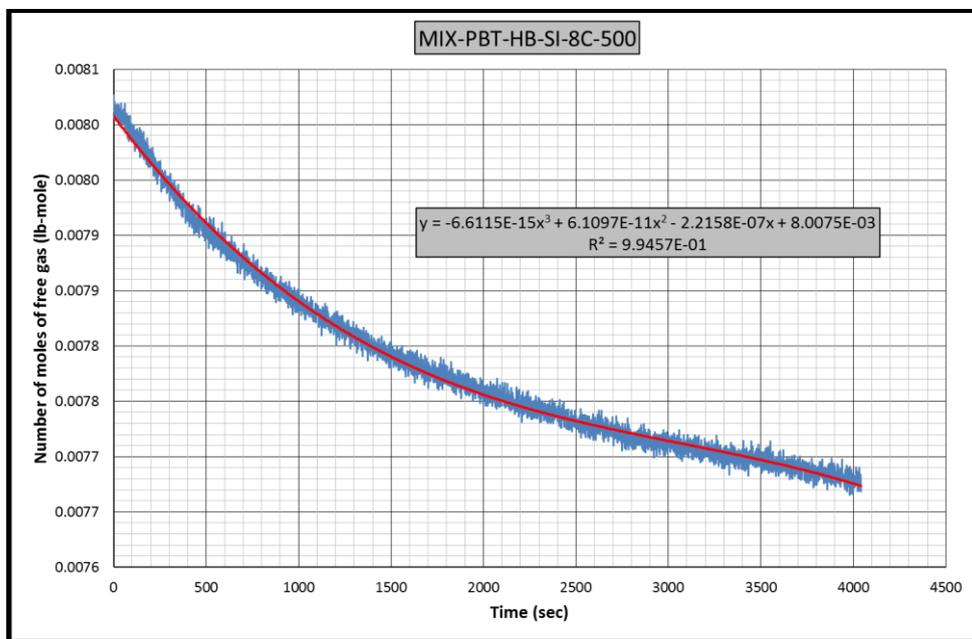
**Figure B.52** Gas consumption rate equation for CH<sub>4</sub>-C<sub>3</sub>H<sub>8</sub>-PBT-HB-SI-8C experiment
