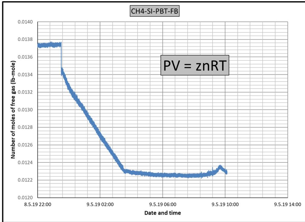
**Figure 6.4** Calculated number of moles of free gas during hydrate formation
