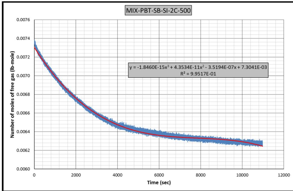
Figure B.75 Gas consumption rate equation for CH<sub>4</sub>-C<sub>3</sub>H<sub>8</sub>-PBT-SB-SI-2C experiment
