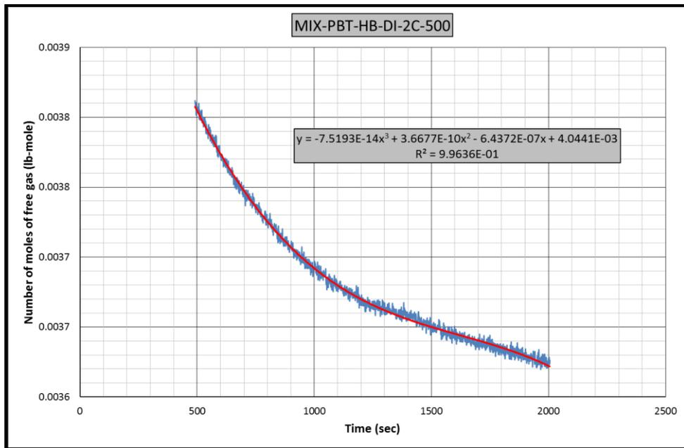
*Figure B.96* Gas consumption rate equation-2 for CH<sub>4</sub>-C<sub>3</sub>H<sub>8</sub>-PBT-HB-DI-2C experiment
