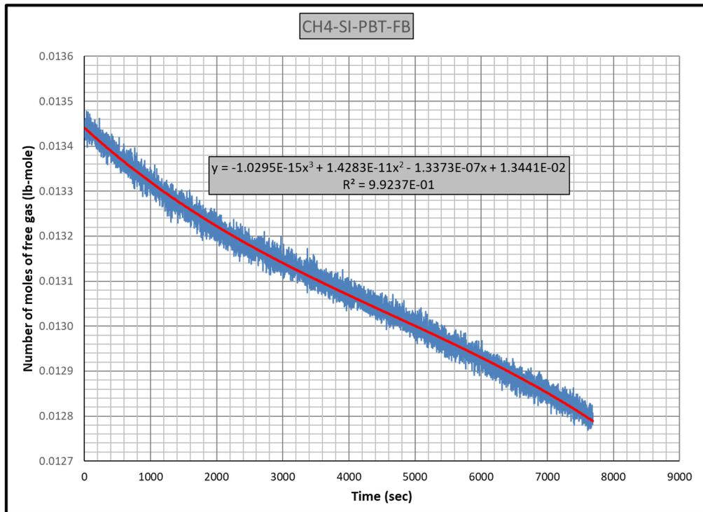
**Figure 6.5** Gas consumption rate equation
