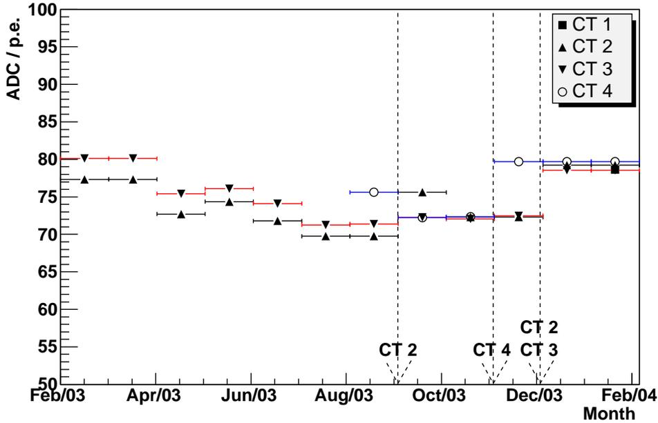
Fig. 10. Evolution of the mean  $\gamma_e^{ADC}$  per camera in 2003/04. The large arrows correspond to an HV increase for the labelled telescope. Telescopes were installed in the following order: CT3, CT2, CT4 and CT1.
